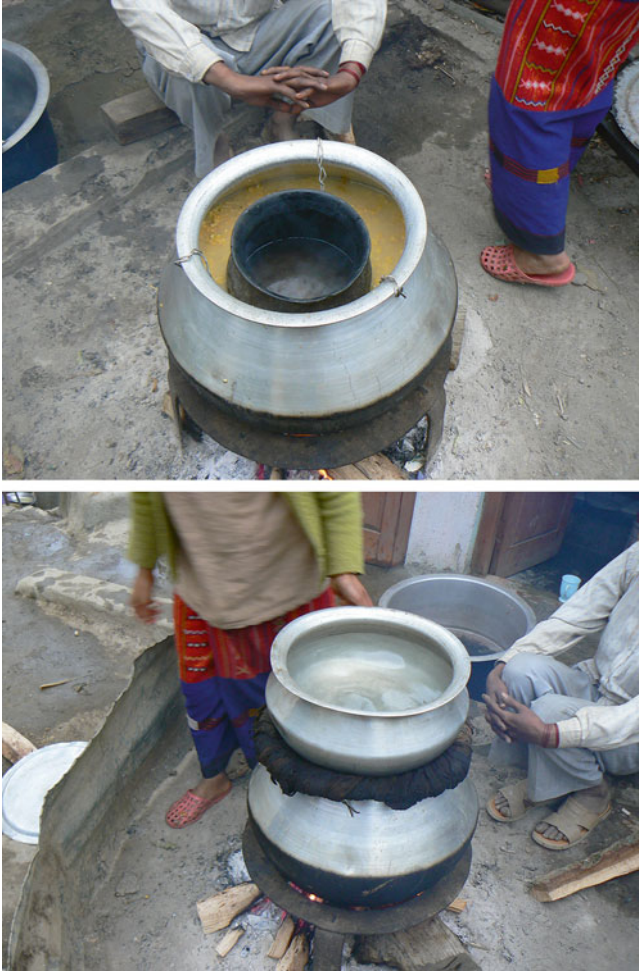
Fig. 7.11 Distilled alcoholic drinks are made by a simple method. Cereal grains are boiled in a large container, and a smaller container is placed within it, as indicated in the upper photograph . Vaporized alcohol is then cooled down by another vessel containing water, and distilled spirit accumulates in the small container as seen in the lower photograph
