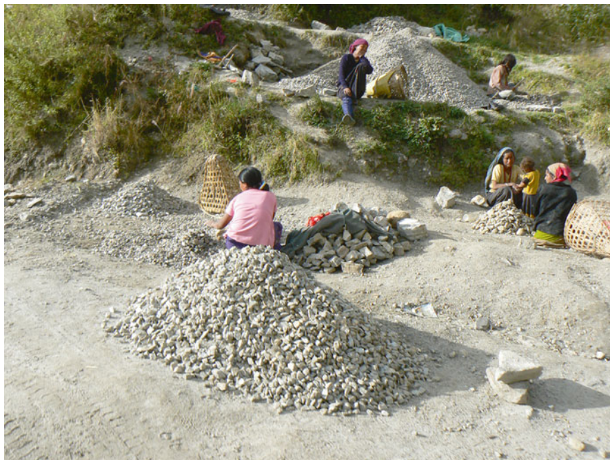
Fig. 4.49 Women crush rocks with a hammer to make pebbles by the roadside. The pebbles are used as construction material for roads and bridges
