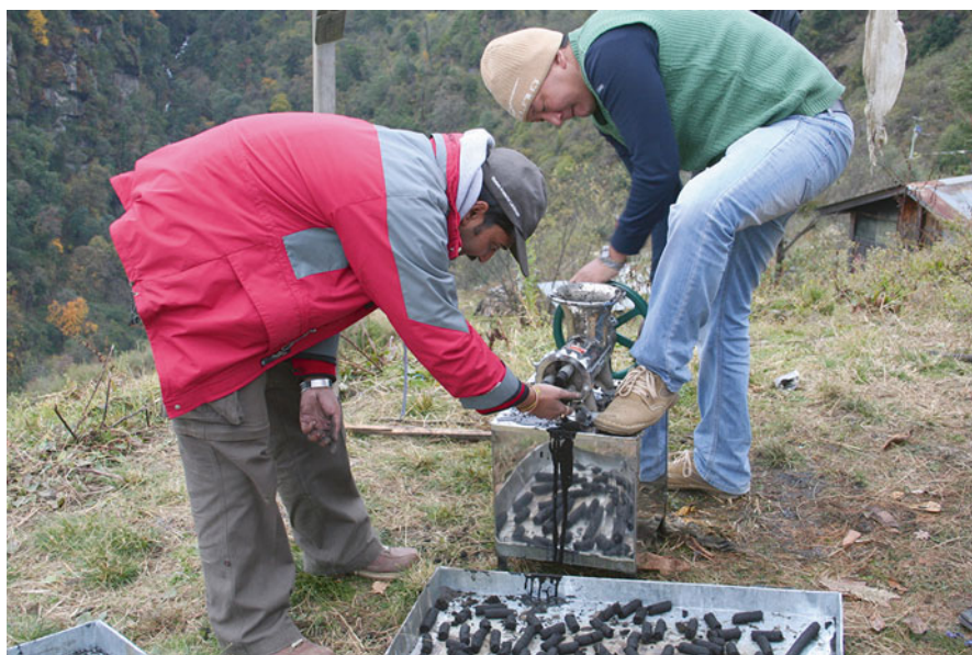
Fig. 5.17 This device was invented to streamline the process of fuel production from yak dung. Yak dung is inserted into the device, and burning and carbonization result in a piece of rod-shaped fuel (This photograph was provided by Mr. Pijush Kumar Dutta of the World Wide Fund for Nature)
