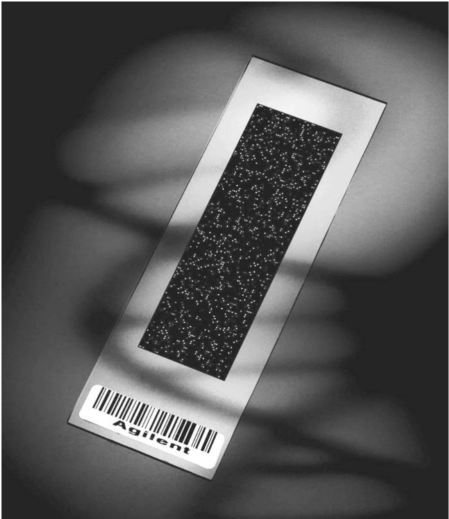
FIGURE 17.2 Example of a microarray printed on the standard 1" × 3" glass slide format; the slides are accessible to standard 1" × 3" microarray scanners. (Courtesy of Agilent Technologies, www.agilent.com .)
