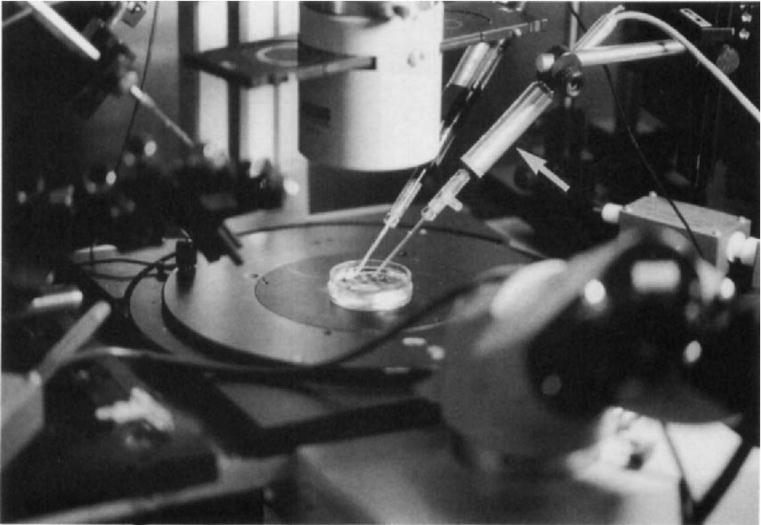
Fig. 7 The experimental setup used for the ion-selective vibrating electrode is mounted over a Zeiss IM35. Both the electrode and the headstage preamplifier (arrow) are vibrated together by stepper motors under computer control. Images are viewed remotely by video through the microscope side-port. The whole assembly is enclosed in a box-like Faraday cage.
