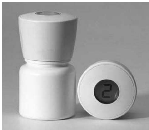
Figure 35.5 MEMS. Pill box that measures compliance by recording openings.
