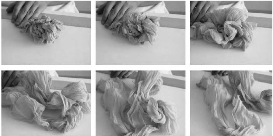
Figure 4. Fabric self shape recovery.
