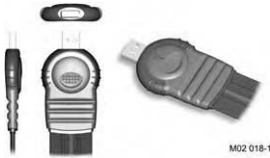
Figure 5a. Proposed USB Connector Design.
