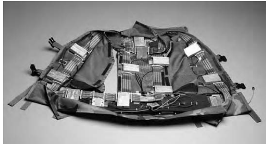
Figure 7. Double Loop Antenna Integrated into MOLLE Vest.
