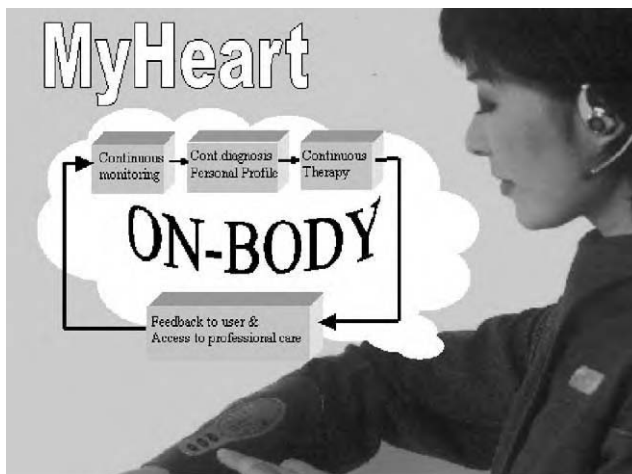
Figure 2.1. Major functional building blocks of the MyHeart system. MyHeart solutions consists of monitoring capabilities that enable a continuous diagnosis to adapt and enable therapy by direct feedback to the user but also to provide timely access to premium institutional points-of-care.
