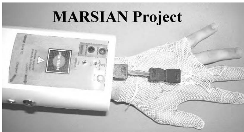
Figure 9. MARSIAN, Modular Autonomous Recorder System for measurement of Autonomic Nervous system activity, is an ambulatory micro central composed of smart clothing and gloves and a wrist device.
