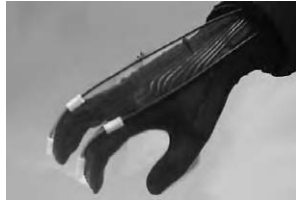
Figure 5. The sensing glove and the electrogoniometers for the calibration phase.
