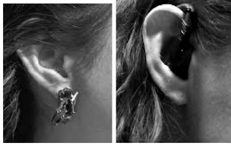
Figure 2. The photoplethysmograph sensor (left) is very sensitive to placement and motion artifacts. The thermistor sensor on the right is much less sensitive. Both can be used to measure heart rate.
