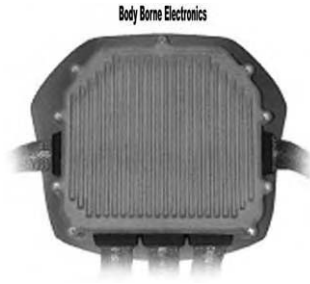
Figure 6. OFW CPU with Attached Electro-Textile Cables.
