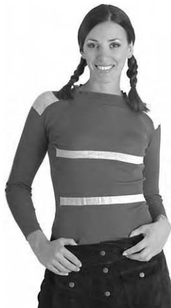
Figure 3. Prototype of smart clothes with electrodes for movement measurement at shoulders and respiration bands (courtesy of European IST WEALTHY project) [5].
