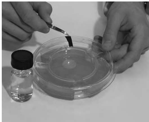
Figure 3. At the Hohenstein Institutes skin equivalents are used to evaluate the functions of medical textiles.
