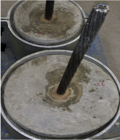
FIGURE 3.69 Cable embedded in test sample using a slow set resin.
