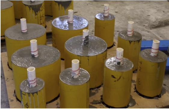
FIGURE 3.66 Post the pouring of cement into the casting molds.
