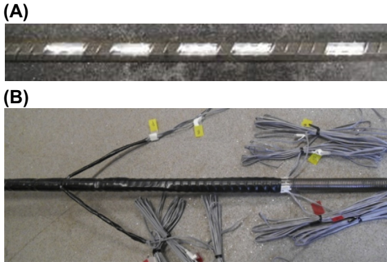
FIGURE 2.78 Rockbolt and the strain gauges. (A) Ground and polish sections of a rockbolt prior to application of strain gauges; (B) view of final instrumented strain-gauged rockbolt.
