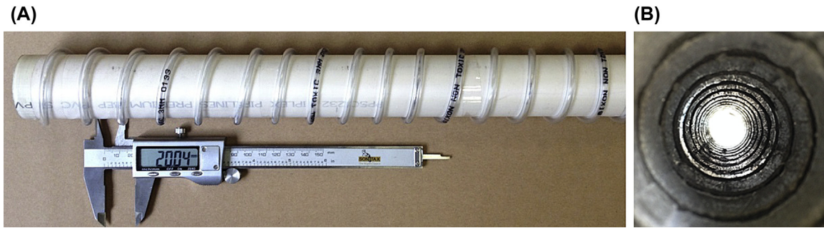
FIGURE 3.27 Spiral plastic tube wound around outside of the pipe and the corresponding rifled borehole. (A) spiral plastic tube wound around outside of the pipe; (B) corresponding rifled borehole.
