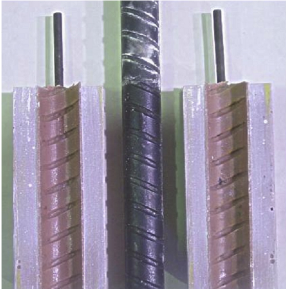
FIGURE 2.58 Resin–bolt separation after postencapsulation. After Aziz, N., Pratt, D., Williams, R., 2003. Double shear testing of bolts . In: Proceedings 4th Underground Coal Operator’s Conference , Wollongong, Australia.
