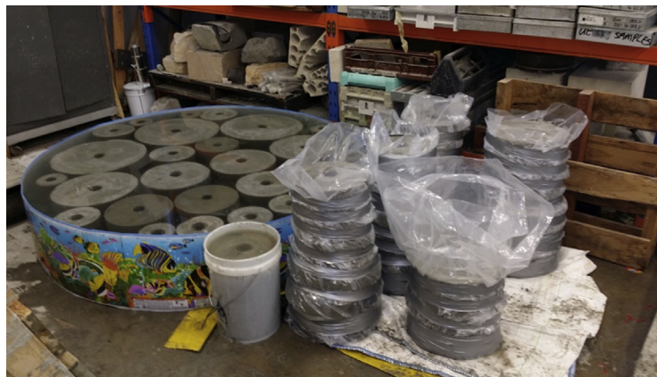
FIGURE 3.68 Test samples fully submerged in water for curing.
