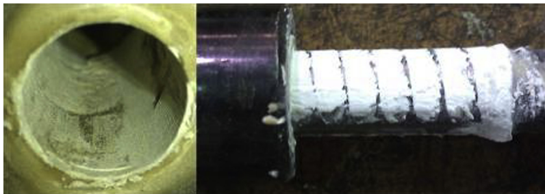
FIGURE 2.27 Parallel shear failure of the resin observed in laboratory pull-out tests.
