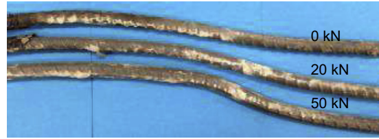
FIGURE 2.81 Deformed rockbolt for different levels of pretension.
