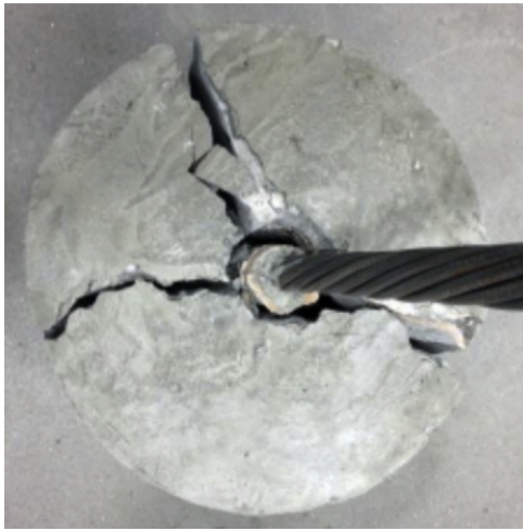
FIGURE 3.73 Typical failure mode of test samples with two or three fractures.
