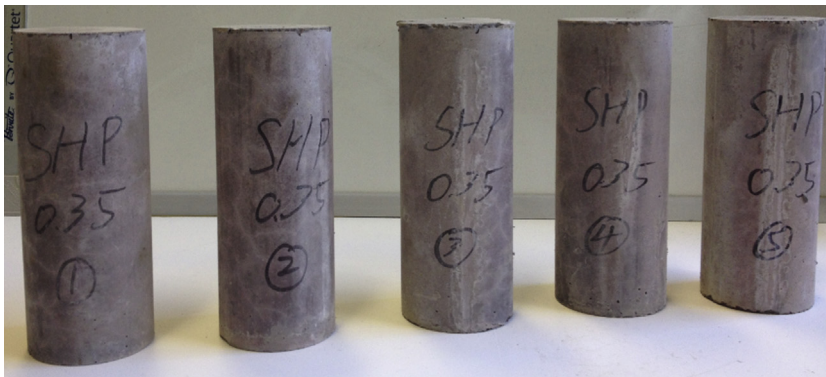
FIGURE 3.30 Cylindrical samples based on the International Society for Rock Mechanics Standard.
