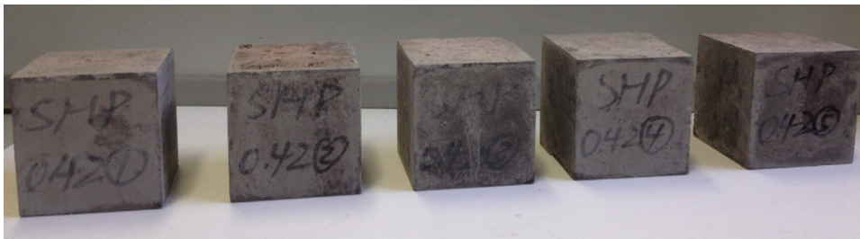
FIGURE 3.31 Cubic samples followed the Australian Standard.
