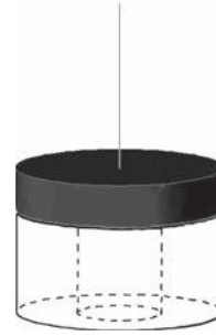
Figure 5. Schematic of a pullout specimen with support.
