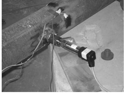
Figure 3. Pressure sensor and strain gauges.
