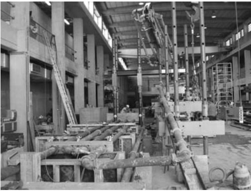
Figure 2. 105 m loop circuit.
