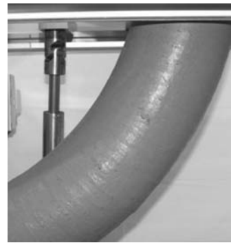
Figure 21. Fabricated elbow pipe, textile reinforcement embedded in concrete.
