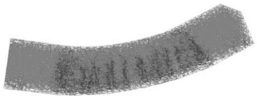
Figure 10. Typical crack pattern in simulated 4 point bending test with 2% fibres.
