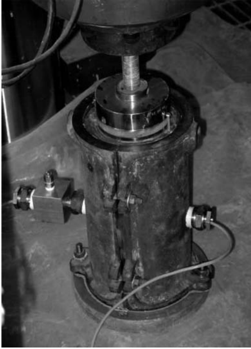
Figure 1. Formwork pressure device.
