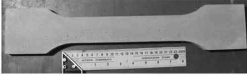
Figure 5. Small dog bone specimen used to derive tensile strength and behavior of ECC.
