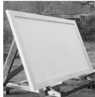
Figure 15. Sand stone imitating panel surface.
