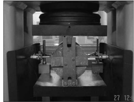
Figure 5. Split cylinder test setup.
