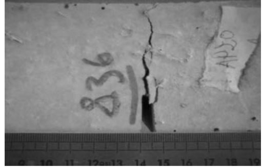
Figure 1. Detail from 70 \times 70 \times 280 \text{ mm}^3 notched beam after breaking.
