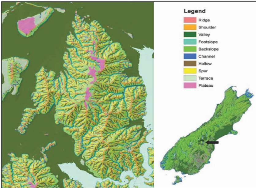
Figure 2. Left - Part of the national landform element map of New Zealand. The Benmore Range is a dry greywacke landscape, and the landform elements shown are based on the combined TOPHAT landscape position model and form element model (local slope and curvature). The final set of landform elements contains 10 classes describing the most common landform features. Right - The landform elements for the South Island of New Zealand based on the combined TOPHAT landscape position model and form element model (local slope and curvature) with the Benmore Range arrowed.
