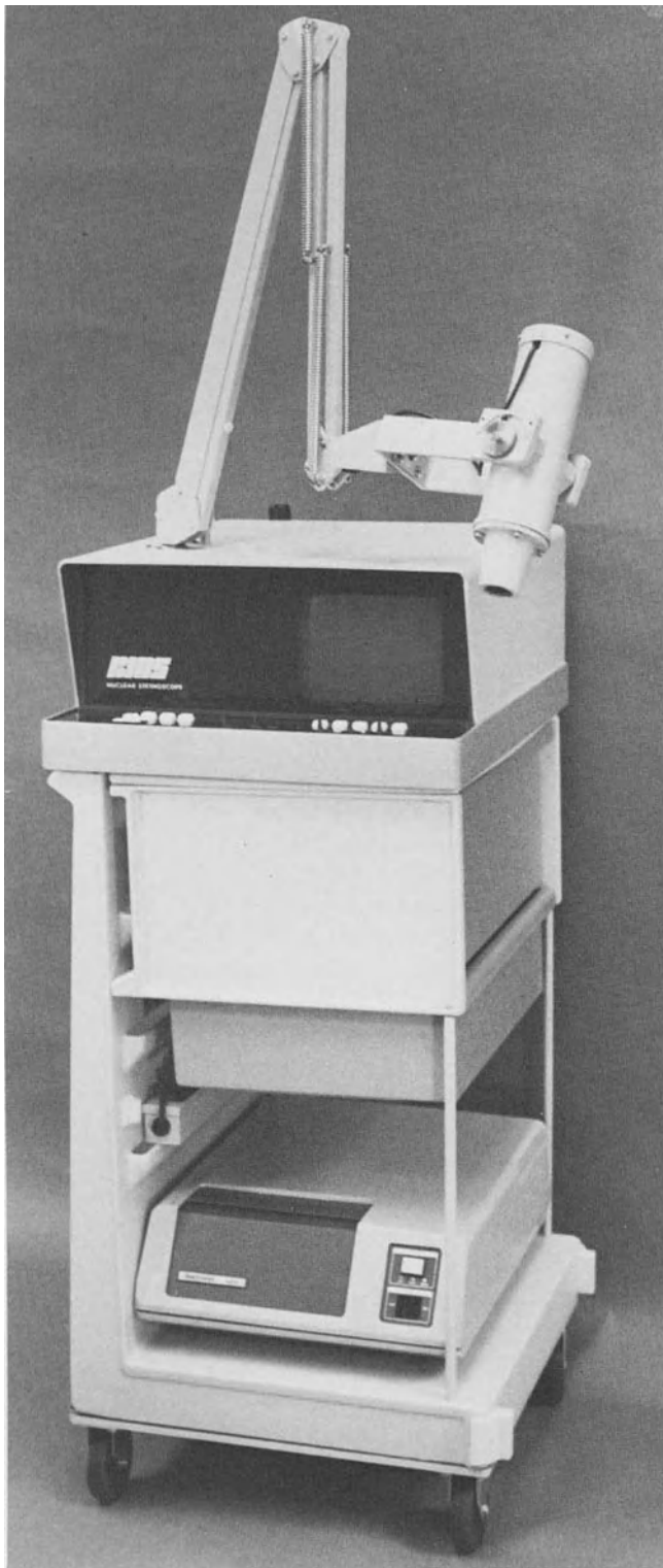
Fig. 3-4. A nonimaging, gated, scintigraphic probe. Note that this device is mobile. The single crystal probe detector is suspended from a free-moving arm that allows the probe detector to be positioned in space. The console contains a small video screen for the display of data as well as controls for acquisition and processing of information by the self-contained microcomputer. A video copier is seen on the bottom of the cart, permitting copies of the studies to be made. The system depicted is the Nuclear Stethoscope™ Cardiac Probe, a trademark of Bios Inc., Valhalla, New York.
