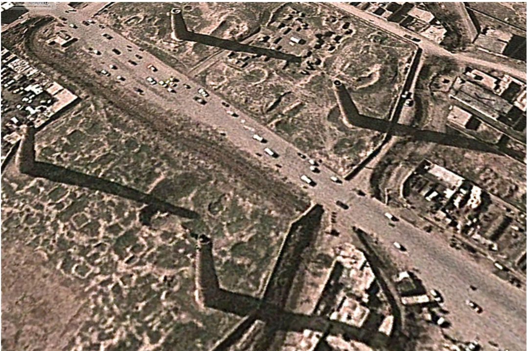
View from space of four of the five remaining minarets in Herat in 2012 (© GoogleEarth). The minarets (~ 55 m high) lean perilously far from the vertical and are the subject of UNESCO restoration
