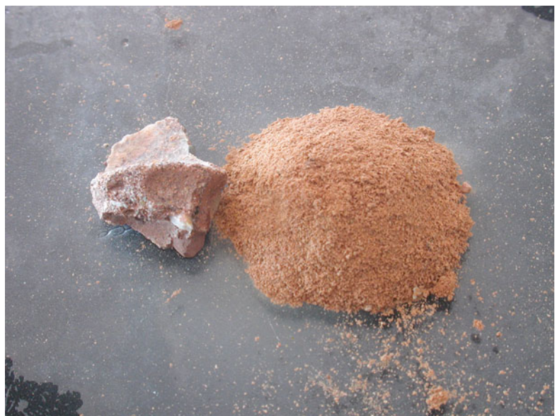
Fig. 7.9 Stability of conglomerate ( left ) and degradation of siltstone ( right ) after only a few minutes of immersion in water
