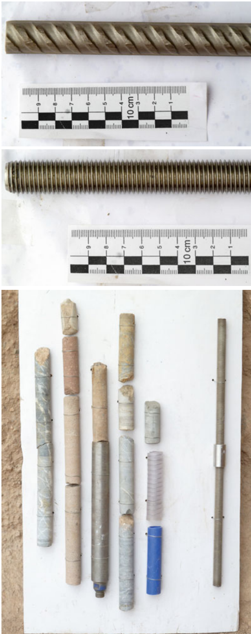
Figs. 13.23, 13.24, and 13.25 Anchor material of V2A-steel, typical bore cores, and different materials used for the stabilization
