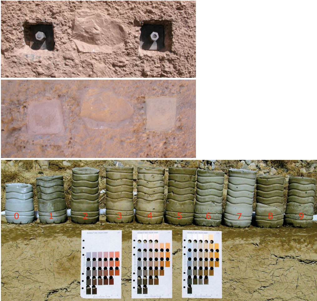
Fig. 11.17 Covering of anchor heads with proper mortar (test site)
