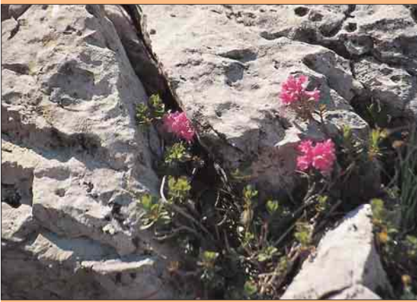
7.31 Massive dolomite – a very hard rock that does not effervesce readily with dilute HCl. Typically makes a sharp ring when struck with a hammer. Width of view 25cm.
