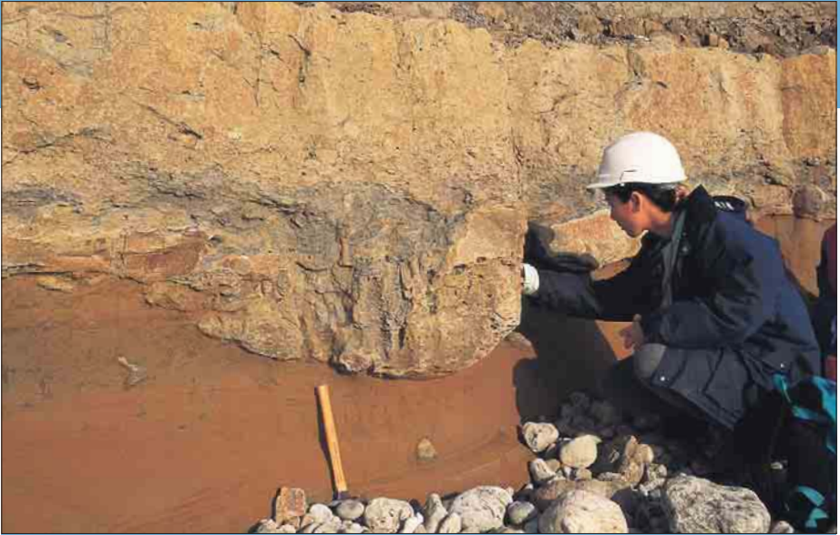
Nose to the rocks. Detailed field observation of discontinuity, Osmington Mills, S. England.
