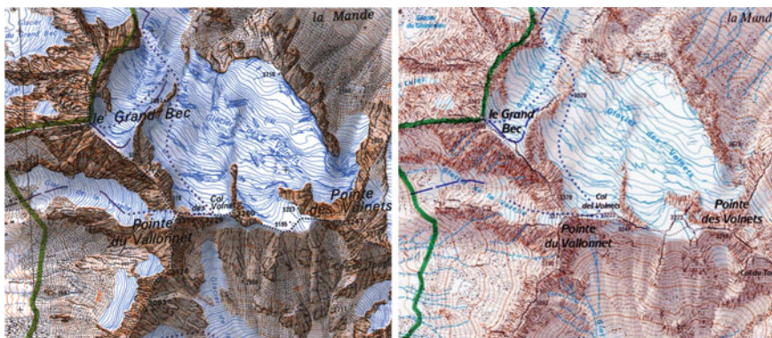
Fig. 11.6 Mountain representation: (left) current map obtained manually in the past; (right) test with numeric representation
