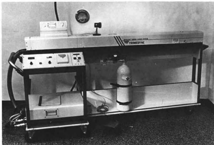
Figure 6-1. Prototype clinical laser system for cardiac application. The power supply, laser tube and head, along with a pulse modulator are mounted on a mobile cart. (Reproduced with permission from The Futura Publishing Co, Inc, Mt Kisco, NY, 1986.)
