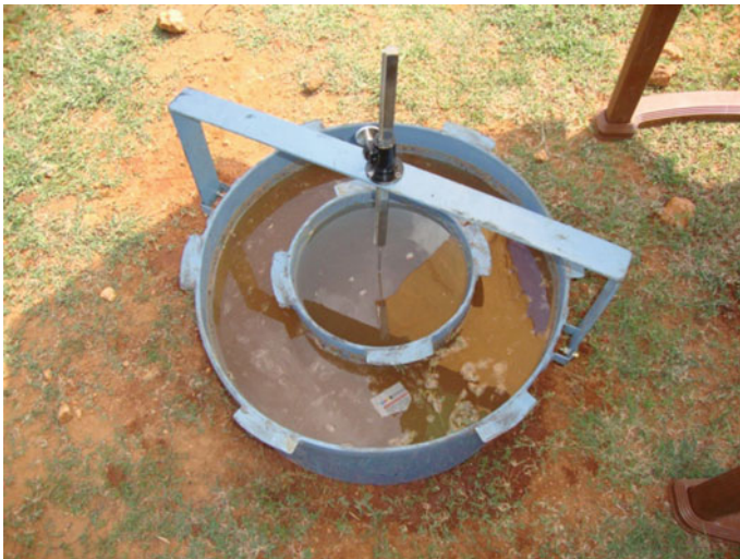
Fig. 2 Field photograph showing conducting infiltration test using double-ring infiltrometer
