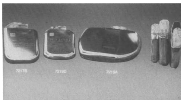
Fig. 1. Decline of implantable cardioverter defibrillator (ICD) size shown for the PCD (Medtronic). The original model 7216A of 1989 had a volume of 209 ml, the model 7217B of 1990 a volume of 113 ml and the model 7219D of 1993 a volume of 83 ml. Diameters were 27, 20, and 18 mm, respectively
