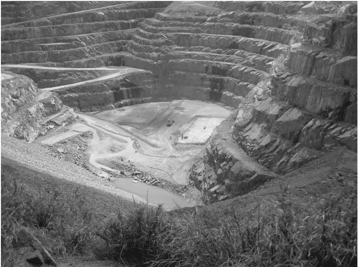
FIGURE 6.1. A typical deep open-pit created by a hard-rock mining operation. In this case, about 50 m of regolith (mostly oxidized broken rock or oxide) is located above the main ore body.
