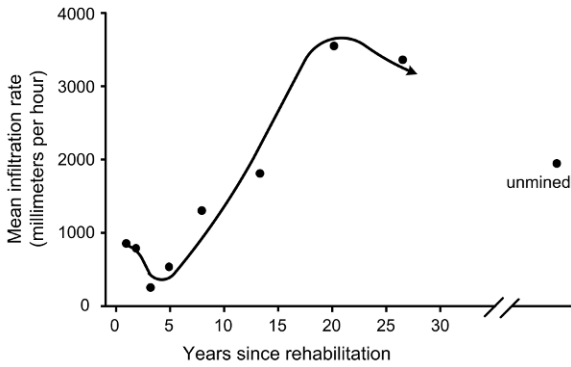
FIGURE 4.12. Measured water infiltration rates on rehabilitated sites of increasing age and on an unmined site at Gove.
