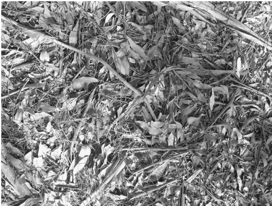
FIGURE 12.3. Coarse mulch material has remained intact on a verge slope, protecting it from the erosive forces of rain and wind storm events. This mulch was sourced from when the forest was cleared to construct the roadway.
