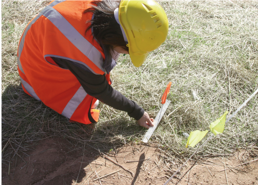
PLATE 6.3. Restoration practitioner making additional measurements that will be used to determine the effectiveness of strips of mulch in trapping sediments eroding from upslope.
