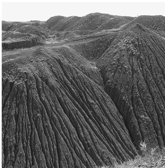
FIGURE 8.2. A typical open-cut coal mining operation that has created extensive piles of spoil (over-burden). Note the erosion on the steep slopes of these spoil piles. The road on the top indicates that these spoil piles are up to 50 m high.
