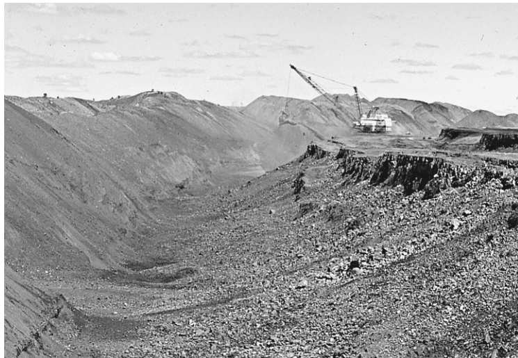
FIGURE 8.1. An example of an open-cut coal mining operation where massive drag-lines are used to strip soil and over-burden and expose the coal layer.
