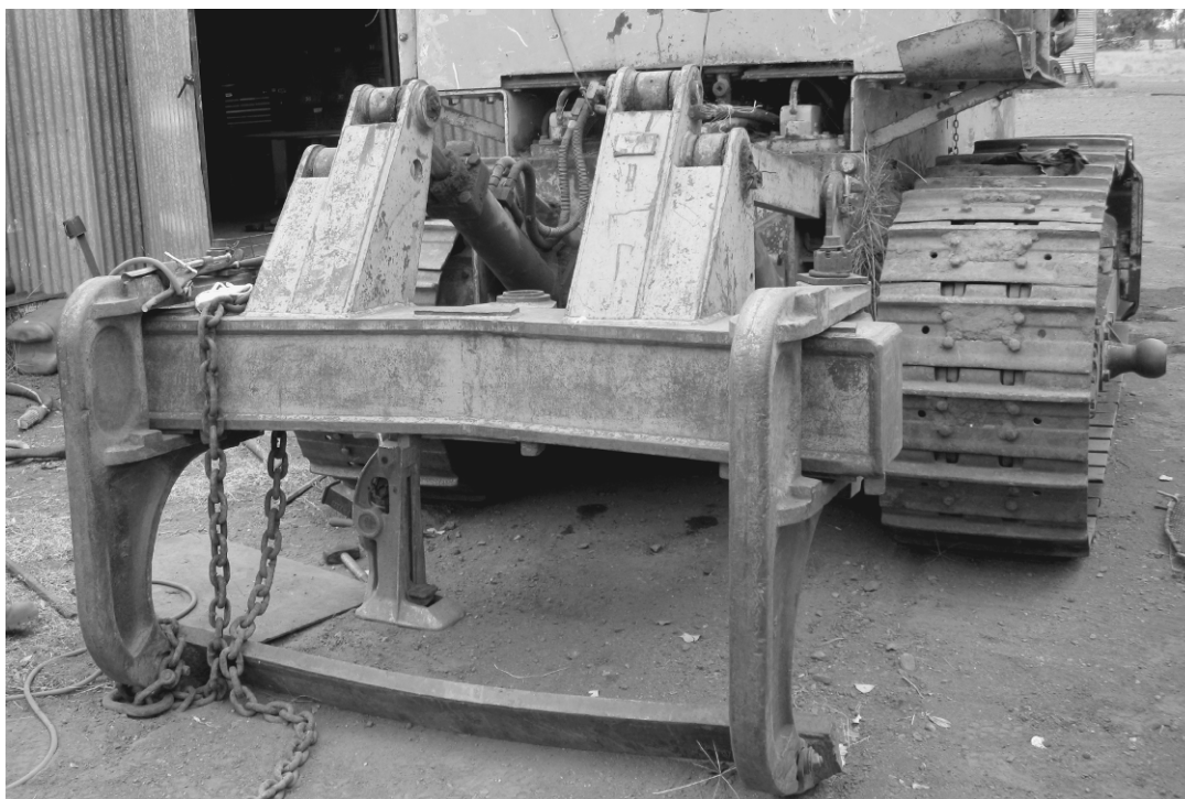
FIGURE 9.3. A blade-plow used to control rangeland shrubs by severing their roots below ground.
