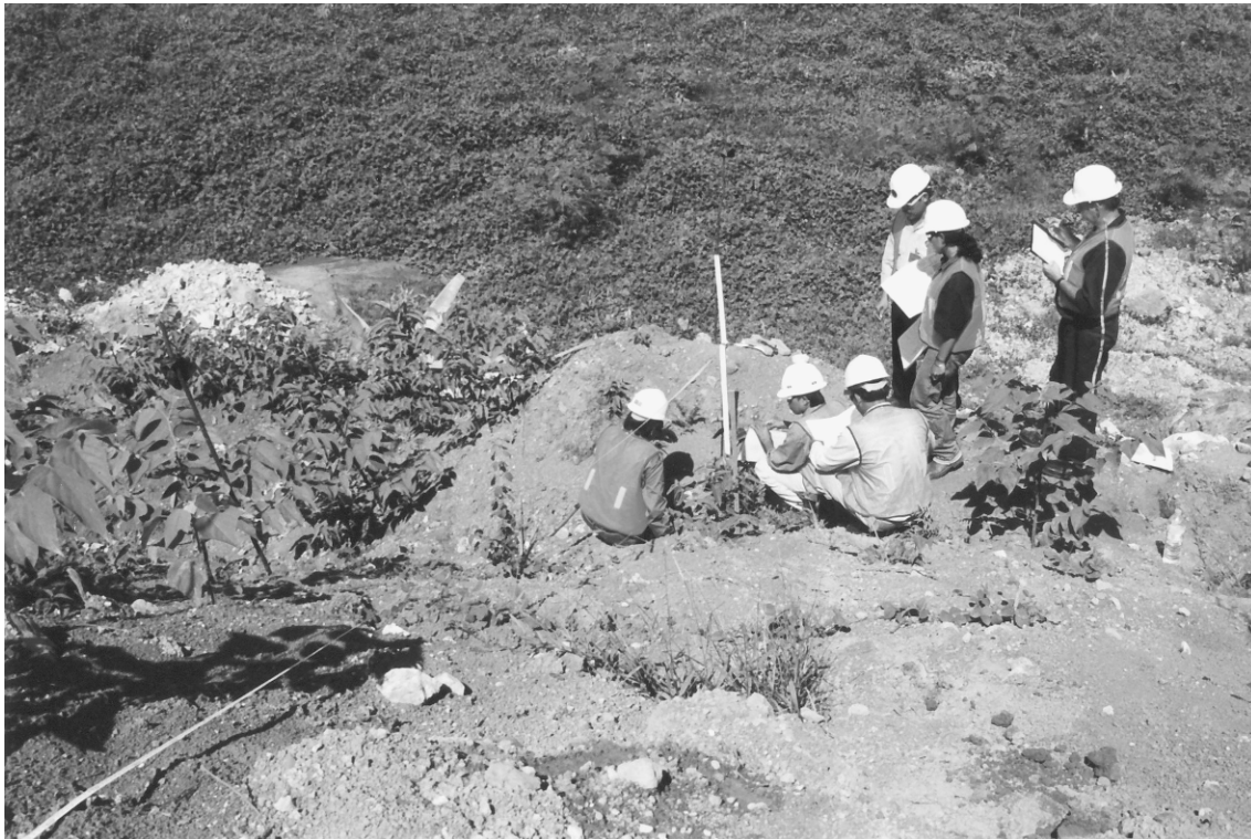
FIGURE 4.17. Restoration practitioners measuring surface condition indicators on “paddock-dumped” locations on a mine site in East Kalimantan (photo looking downslope).
