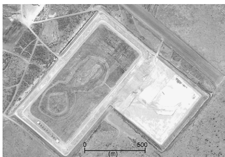
FIGURE 7.1. An aerial view of tailings storage facilities constructed as rectangular ponds with steep sides to reduce their landscape footprint. Photograph courtesy of Harley Lacy.
