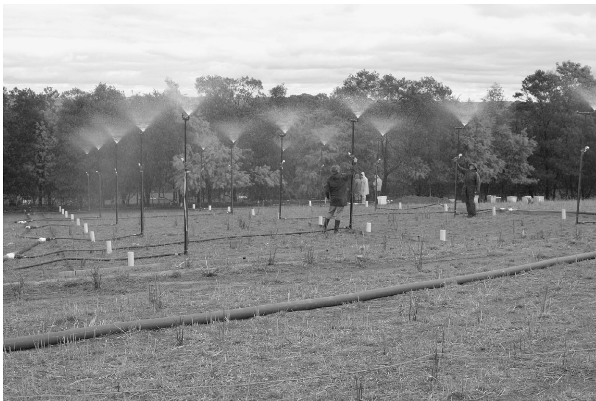
FIGURE 10.6. A rainfall simulator in action delivering water from sprinklers to pasture and tree-belt plots at about 45 mm per hour.
