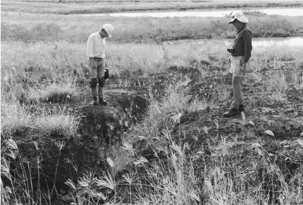
FIGURE 8.10. An example of a gully cutting into a slope reformed from spoil heaps created by open-cut coal mining. Grass plant root systems were unable to sufficiently ameliorate the dispersion properties of the spoil.
