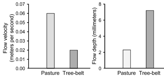
FIGURE 10.7. Runoff or overland flow velocities and depths produced by applying 24.4 mm of water in 30 minutes to pasture and tree-belt plots. See Ellis et al. (2006).
