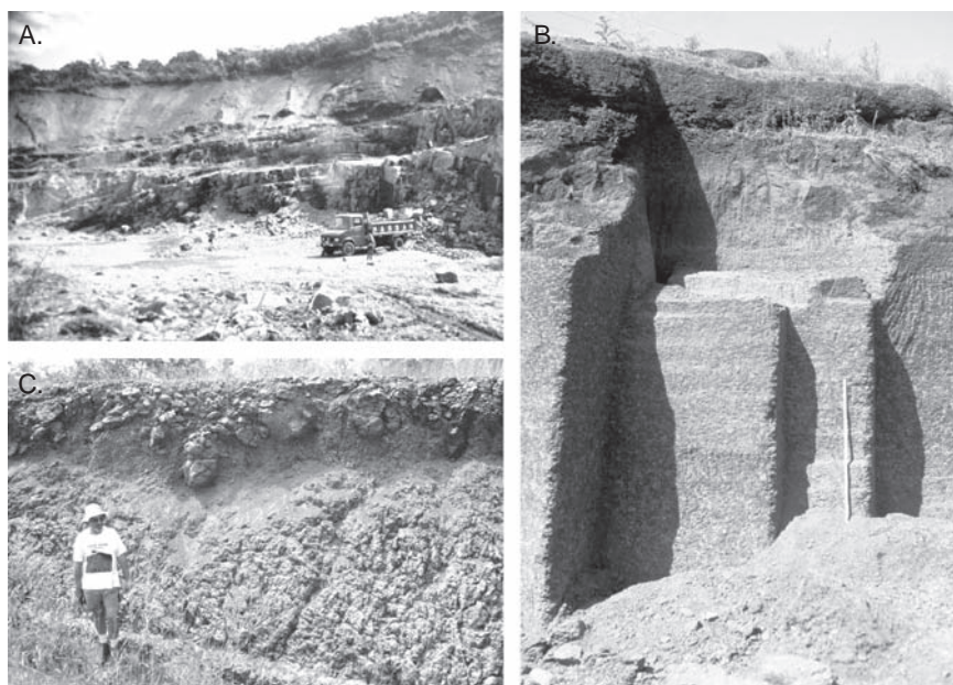
Figure 3.4 Examples of laterite and ferricrete profiles. (A) Mercedes Quarry near Panjim, Goa ( 15^{\circ}29'N , 73^{\circ}53'E ), where an entire laterite weathering profile developed upon Proterozoic greywacke is exposed. (B) Laterite quarrying at Bidar ( 17^{\circ}55'N , 77^{\circ}33'E ), showing recently cut sections (with 1 m rule for scale) where material from the upper parts of the profile (zone IV on Fig. 3) has been extracted for laterite bricks. The Bidar laterite localities were used by Newbold (1846) to argue for laterite as an in situ weathering product. (C) Ferricrete profile exposed in a road cutting to the south of Palika Ba ( 13^{\circ}28'N , 15^{\circ}14'W ), near the Gambia River, Gambia, West Africa.
