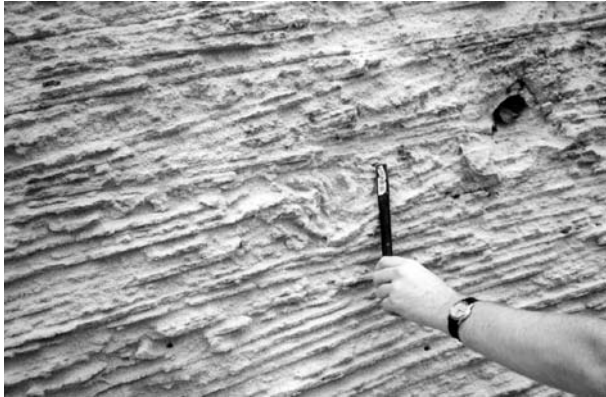
Figure 5.3 Differentially cemented laminae (chisel for scale). The finer grained laminae are better cemented and more resistant to weathering than the coarser-grained laminae. (Note the slumped laminae in the centre of the figure.)
