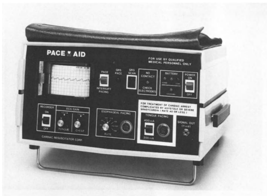
Figure 3. The Pace-Aid device for external pacing using either tongue-epigastrium electrode placement for ventricular stimulation or oesophageal placement for atrial stimulation.
