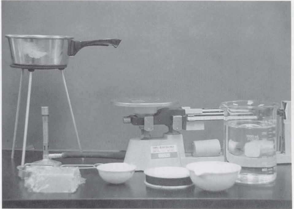
Figure 1 Equipment for measurement of unit weight of cohesive soils. Balance accurate to 0.01 g, solidified wax block, and wax bath, container filled with water, and evaporating dish
