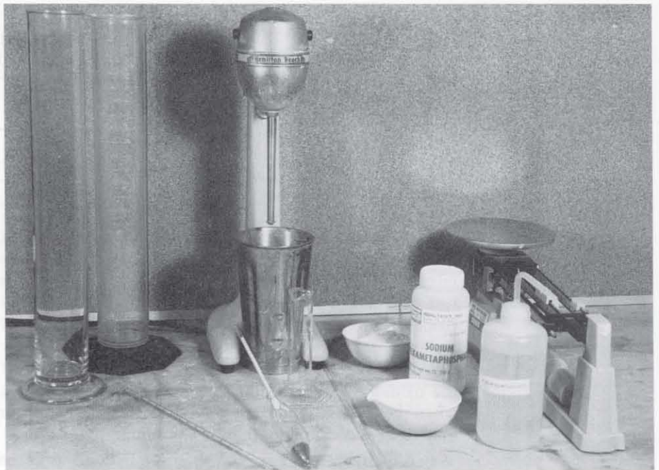
Figure 1 Equipment for hydrometer analysis. From left to right, two graduated cylinders, also called sedimentation cylinders, a thermometer, a hydrometer, dispersion apparatus, two porcelain evaporating dishes, a stock solution of sodium hexametaphosphate, and a scale.
