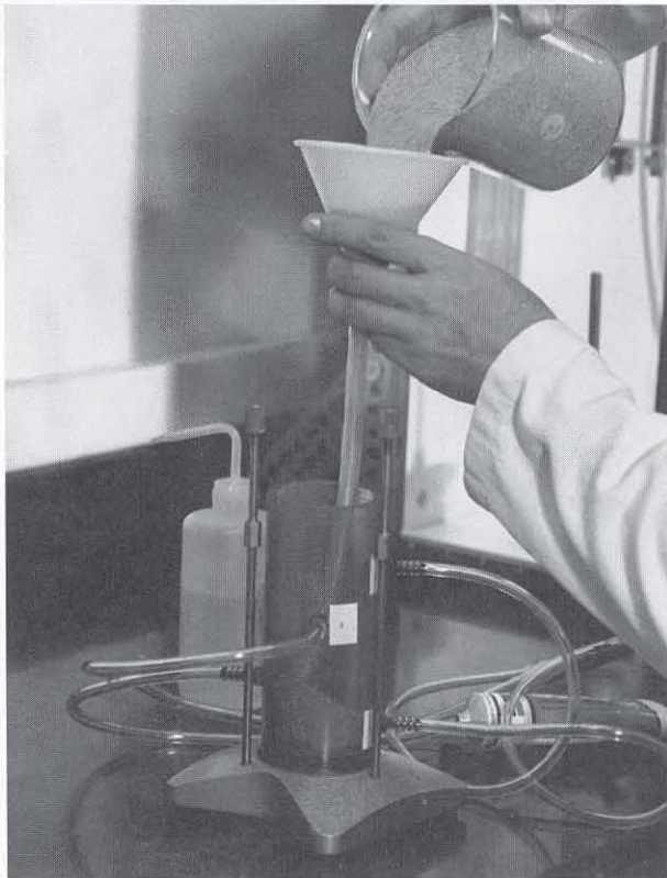
Figure 7 A loose specimen is obtained by using a funnel and a flexible nozzle. Denser specimens are obtained by tapping or vibrating loose samples.
