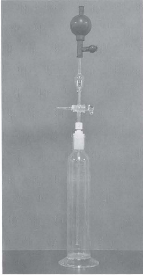
Figure 2 The Andreasen pipette, its sedimentation cylinder, and a rubber pumping and sucking device.
