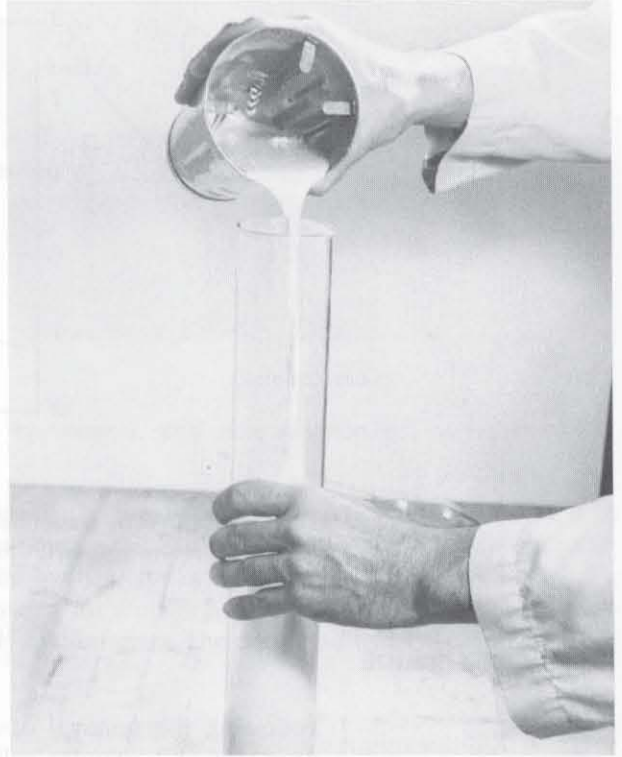
Figure 7 After dispersion, the soil suspension is poured into the sedimentation cylinder.
