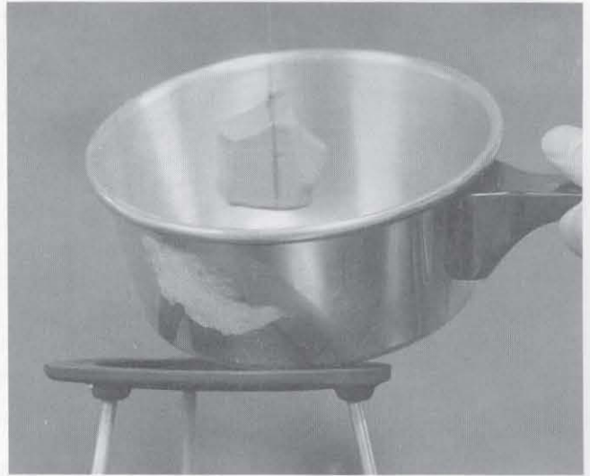
Figure 4 The specimen is immersed in a bath of melted wax.
