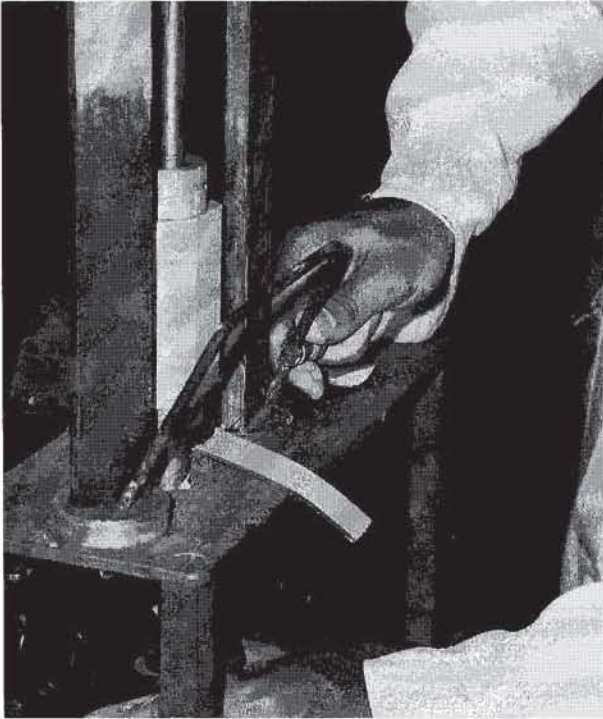
Figure 1 The sample is installed on a trimming frame. The vertical guides are adjusted to obtain the desired sample diameter.
