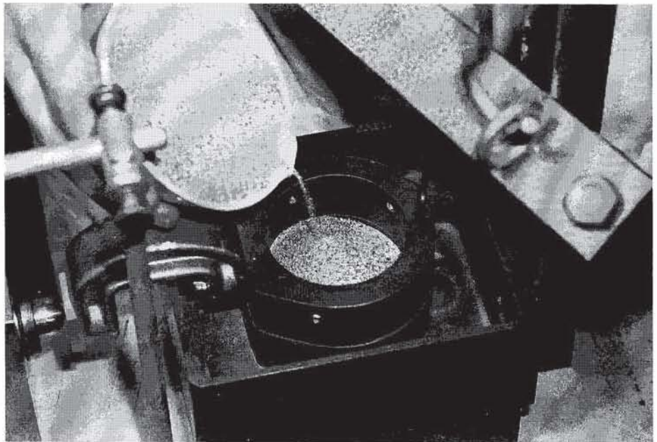
Figure 8 Filling the shear box with sand.
