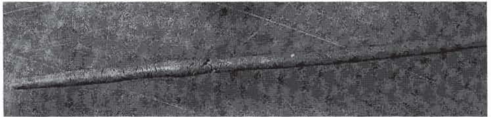
Figure 2 The 3-mm-diameter soil thread crumbles when the water content is equal to the plastic limit.
