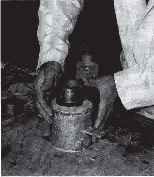
Figure 5 A stack of rings of identical diameter is pushed into the soil mass. The lowest ring has a cutting edge. The other cylinders are oedometer floating rings.
