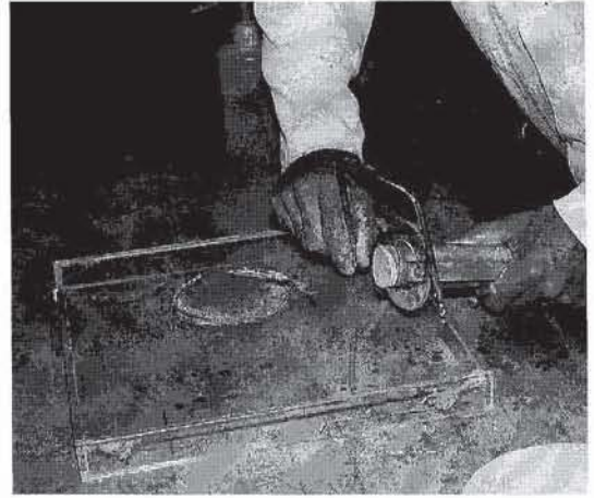
Figure 8 After extruding about 1 cm of soil from the sampling tube, the bottom surface of the sample is cut with a wire saw.
