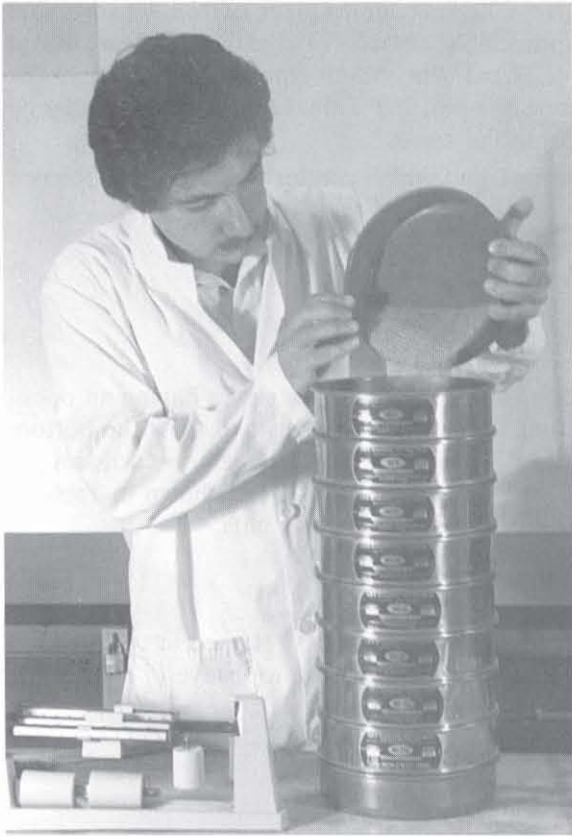
Figure 3 The soil sample is poured on the stack of sieves with a pan at the bottom.
