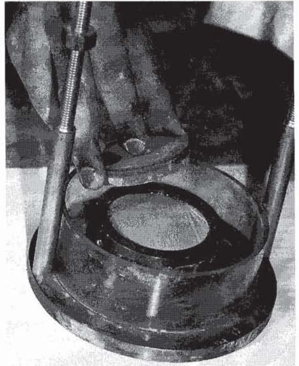
Figure 8 Filter papers are added to the top and bottom surfaces of the specimen. Then the floating ring is placed on the bottom porous stone and the top porous stone is positioned.
