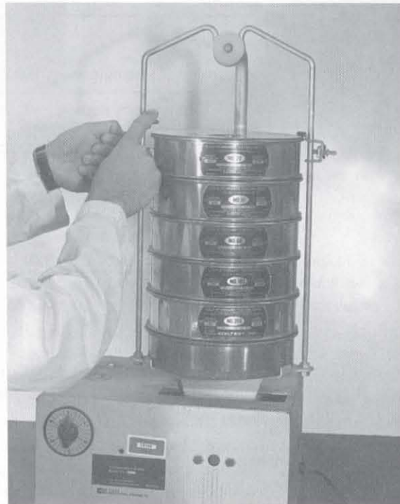
Figure 2 The stack of sieves is mounted on a mechanical shaker.
