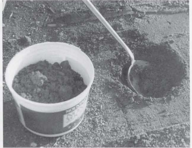
Figure 9 A hole is excavated with an opening size slightly larger than the base plate opening.
