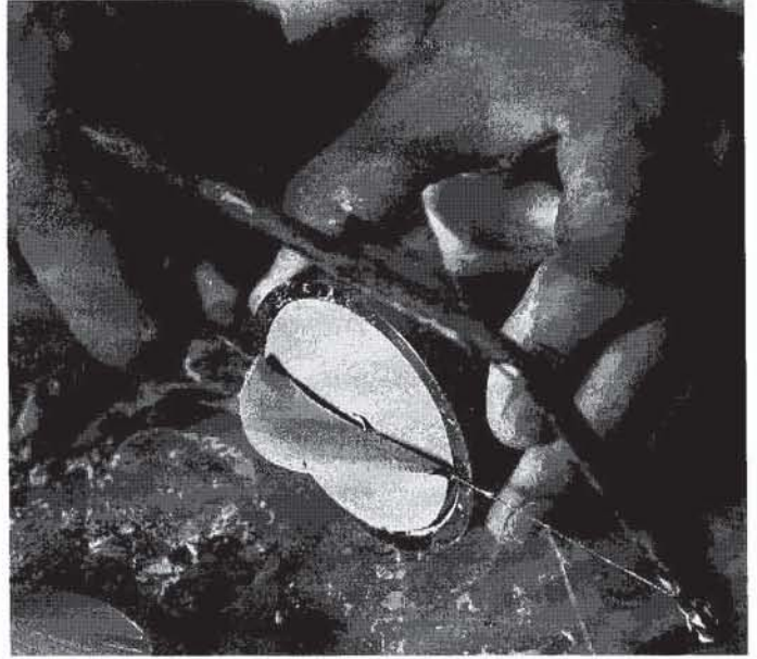
Figure 6 After removing the stack of rings filled with soil, the wire saw is inserted in the interstices between two rings, and the soil excess is cut off.
