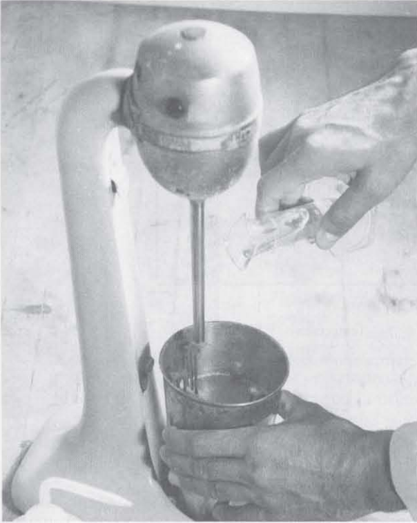
Figure 6 The soil sample is placed in a dispersion cup and the dispersing agent is added.
