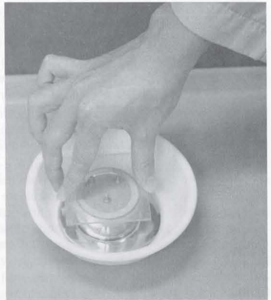
Figure 5 Press the three prongs of the prong plate carefully onto the sample and force it under the mercury.
