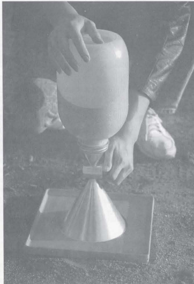
Figure 11 During the actual field test, the valve of the the sand cone is opened and the sand flows down to fill the excavated hole.
