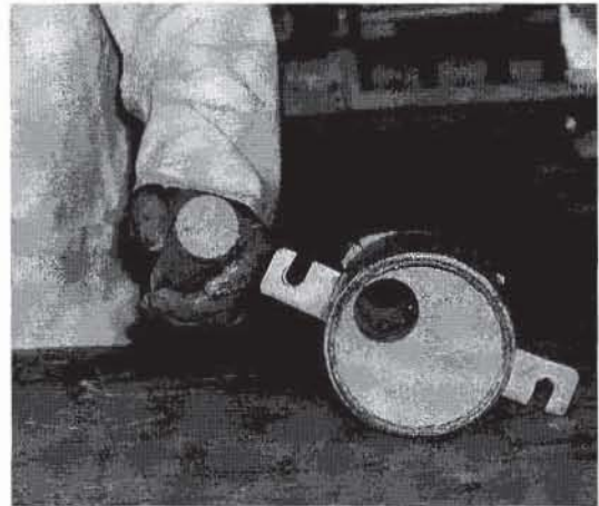
Figure 6 The soil specimen is now in the sampling tube.
