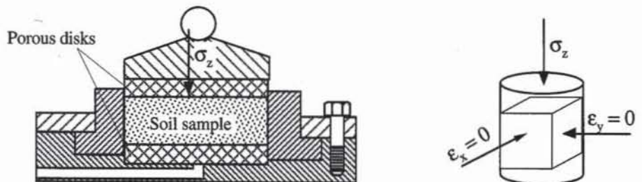
Figure 4 Consolidation cell, and strains and stresses applied to samples during the confined compression test.
