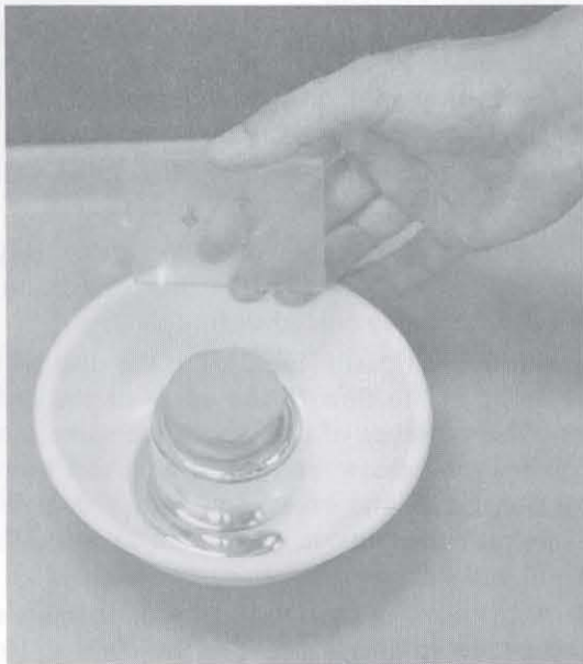
Figure 4 Place the immersion cup in a clean evaporating dish, itself located inside a large tray. Place the dry soil pat on the mercury surface.
