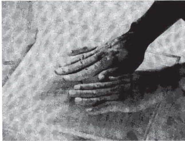
Figure 1 The soil specimen is rolled under the fingers into a thread 3 mm in diameter.
