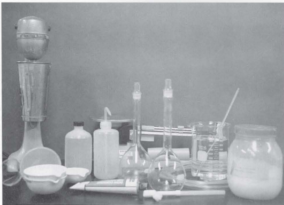
Figure 1 Equipment for measurement of specific density. Balance sensitive to 0.01g, 500-mL volumetric flask, evaporating dish, supply of deaired water, and thermometer.
