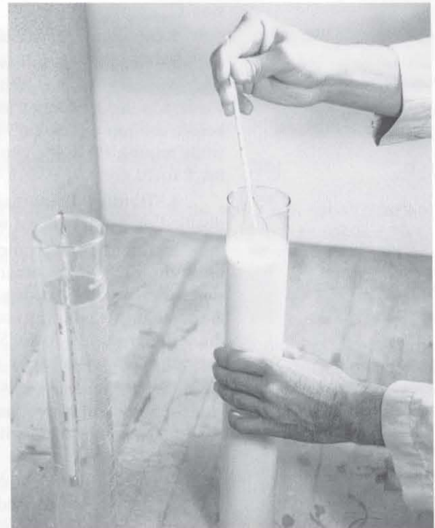
Figure 9 At selected time intervals, the hydrometer is slowly and carefully immersed.
