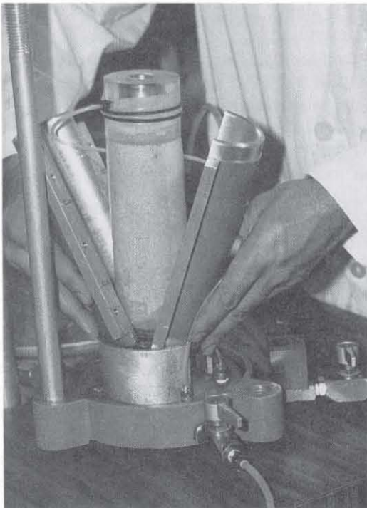
Figure 7 Once the vacuum is applied internally to the sample, the split mold is removed.
