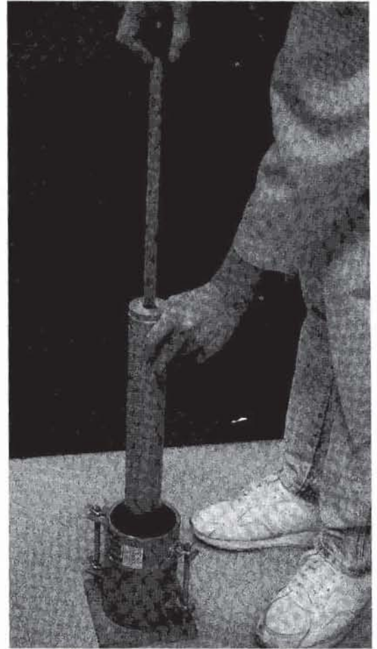
Figure 7 The soil is compacted by applying 25 blows with the rammer.
