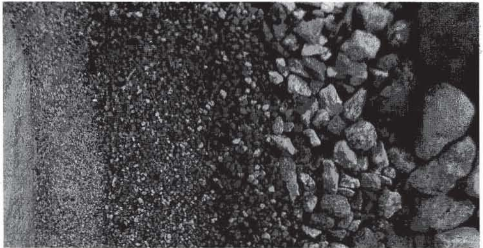
Figure 1 The particles of this soil were divided into six size groups in the laboratory. The largest particle shown is 15 mm in diameter. The largest sizes in each group from left to right are 0.07, 0.3, 1, 2, 5, and 15 mm, respectively.
