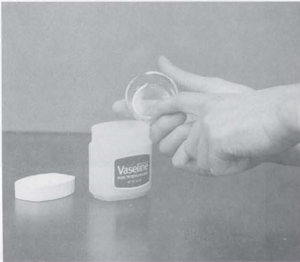
Figure 2 Lightly coat the inside of the shrinkage limit dish with petroleum jelly or silicon grease.
