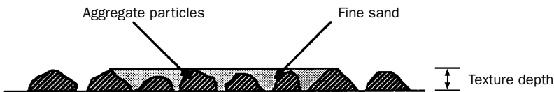
FIGURE 25.4 Measurement of macrotexture using the sand patch test.
