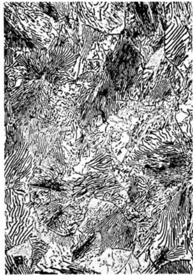
FIGURE 8.9 Relatively coarse pearlite in a plain carbon steel ( \times 200 ) (from A.R. Bailey (1967) The Structure and Strength of Metals , by permission of Metallurgical Services Laboratories Ltd).
