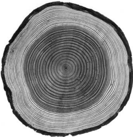
FIGURE 44.2 Cross-section through the trunk of a Douglas fir tree showing the annual growth rings, the darker heartwood, the lighter sapwood and the bark (© Building Research Establishment).
