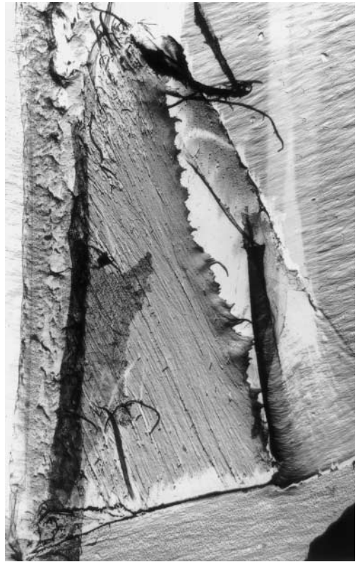
FIGURE 44.15 Electron micrograph of the cell wall in Norway spruce timber ( Picea abies ) showing the parallel and almost vertical microfibrils of an exposed portion of the S 2 layer (© Building Research Establishment).
