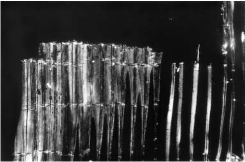
FIGURE 47.1 Kink bands and compression creases in the tension face of a scaffold board which failed in bending on site. Note how the crack pathway has followed the line of the top compression crease which had been induced some time previously (magnification \times 150 ) (© Building Research Establishment).
