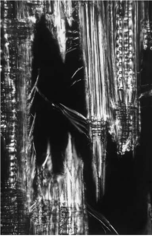
FIGURE 46.9 Tensile failure in spruce ( Picea abies ) showing mainly transverse cross-wall failure of the earlywood (left) and longitudinal intra-wall shear failure of the latewood cells (right) ( \times 110 , polarised light) (© Building Research Establishment).
