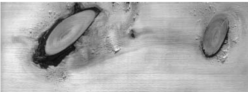
FIGURE 44.4 Black or dead knot surrounded by the bark of the branch and hence showing discontinuity between branch and tree trunk (© Building Research Establishment).
