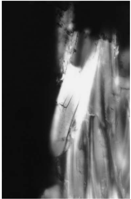
FIGURE 46.12 Crack-stopping in a fractured rotor blade. The orientation of the secondary cracks corresponds to the microfibrillar orientation of the middle layer of the secondary cell wall ( \times 990 , polarised light) (© Building Research Establishment).
