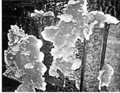
S. lacrymans (dry rot) fruiting body on burnt timber.
