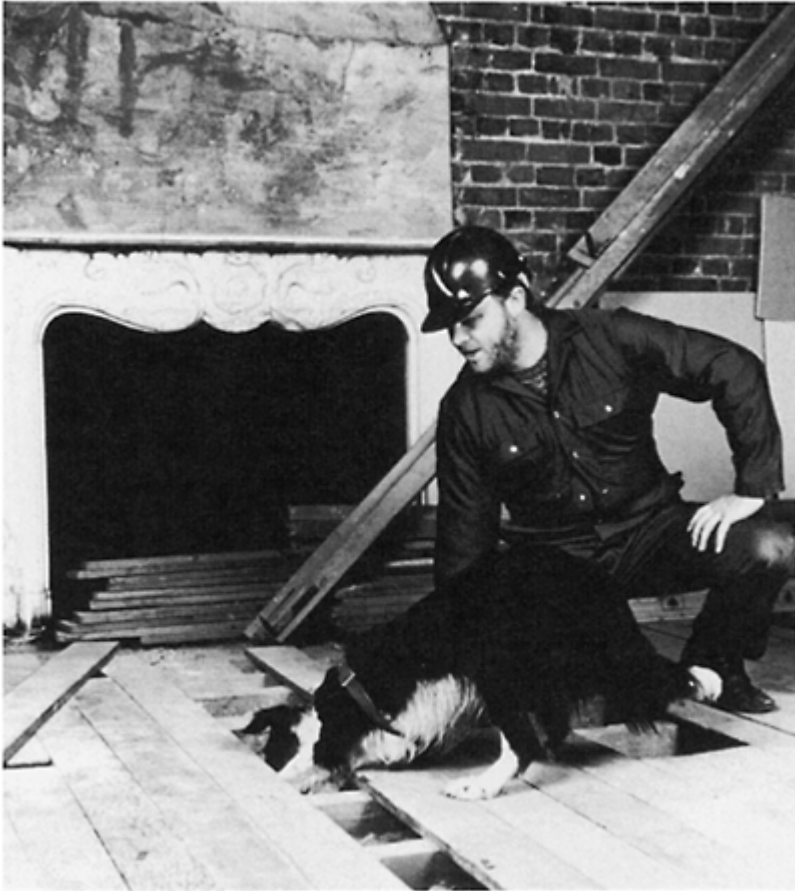
Figure 7.1 Canine detection in a floor void.
