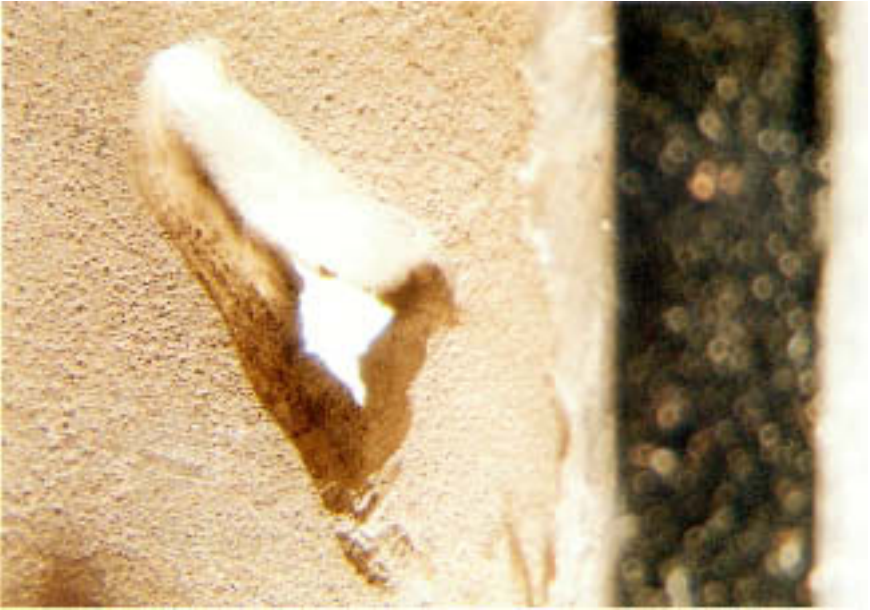
Figure 11.11 Erosion site resulting from lodgement of a foreign body inside a tube. (Magnification: 8 \times .)
