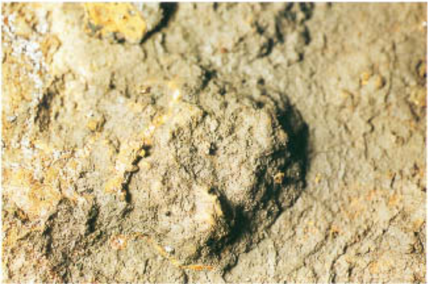
Figure 3.21 As in Figs. 3.19 and 3.20, after several hours of exposure to air. Note the reddening.
