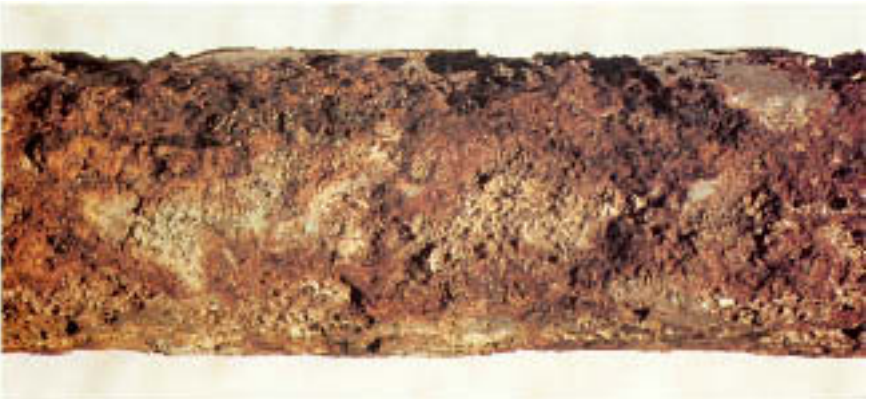
Figure 4.11 General wastage on a 304 stainless steel heat exchanger tube.
