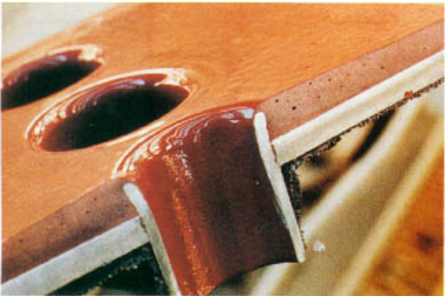
Figure 3.25 Epoxy-coated section of a tube sheet and rolled tube.
