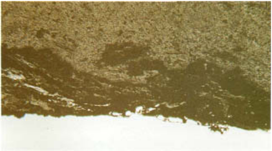
Figure 5.20 Small area on an internal surface with a breach in the galvanized layer. (Magnification: 110 \times , unetched.)
