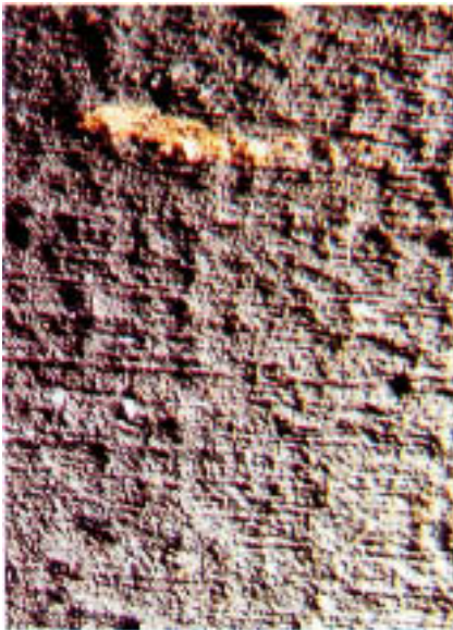
Figure 7.7 Surface striations and shallow grooves on a carbon steel case coupling. Acid etched the metal along microstructural irregularities producing the grooves. Compare to Fig. 7.8. (Magnification: 7.5 \times .)
