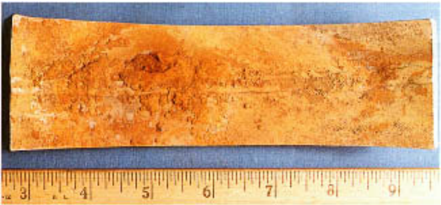
Figure 15.20 Internal surface of 14-in. diameter stainless steel pipe. The circumferential weld is in the center of the specimen.
