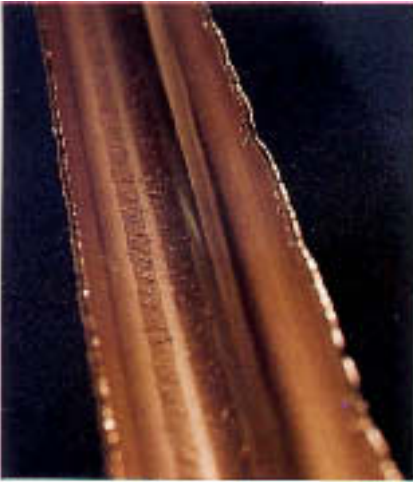
Figure 14.9 Zone of defects running along the internal surface.
