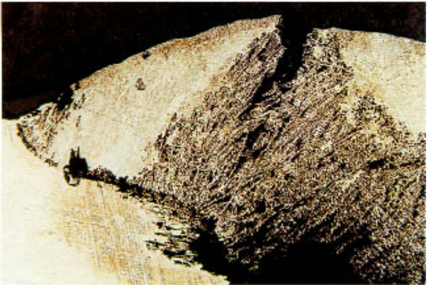
Figure 15.1 Preferential corrosion of the less noble of two phases in a weld bead (cross section). (Magnification: 50 \times .)
