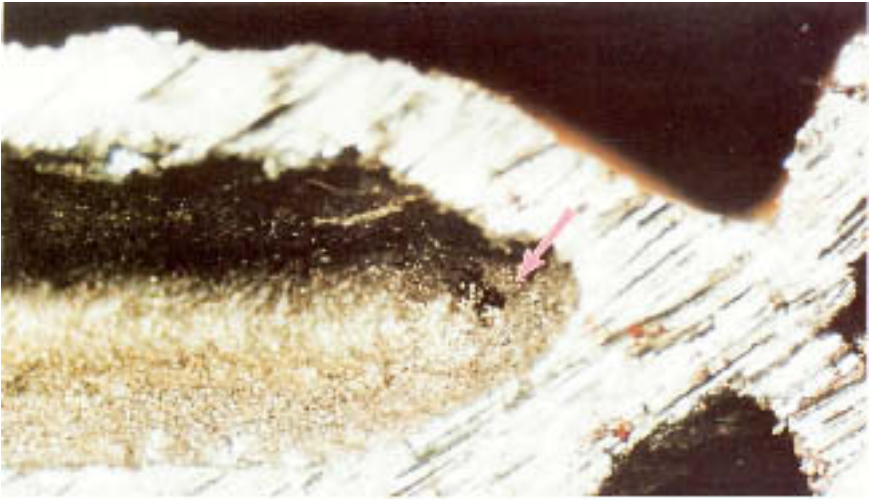
Figure 15.14 Pore formed by emergence of weld cavity at the surface. (Magnification: 15 \times .)
