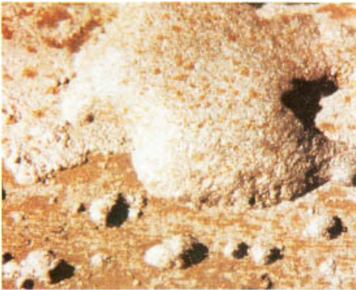
Figure 4.22 As in Fig. 4.21 but with deposits and corrosion products removed to reveal numerous depressions. (Magnification: 7.5 \times .)
