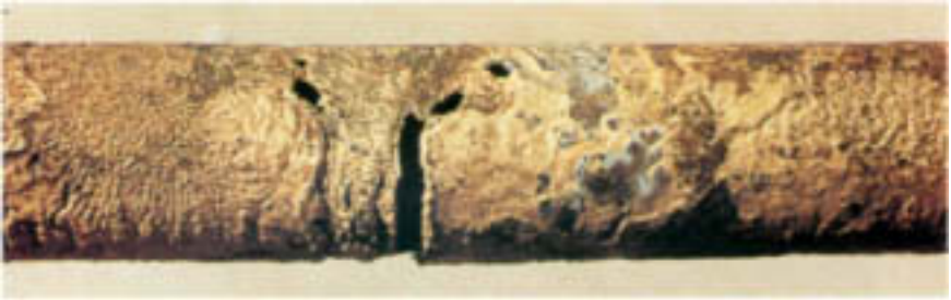
Figure 8.9A A brass condenser tube severely wasted by condensing vapors containing ammonia.
