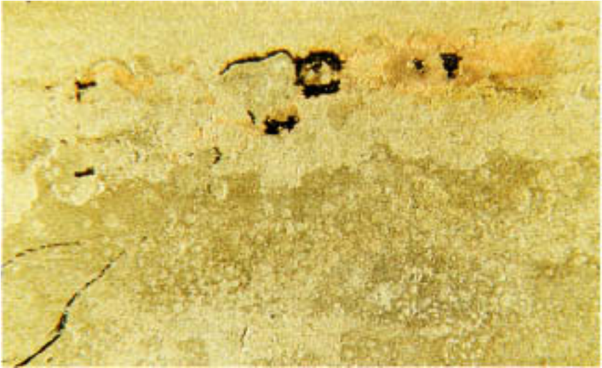
Figure 13.12 Close-up of a 90:10 cupronickel condenser's internal surface after acid cleaning. Elemental copper stains mark regions of shallow denickelification.
