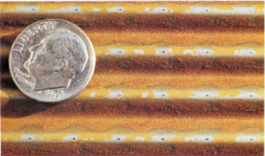
Figure 2.20 Austenitic stainless steel plate from plate-and-frame heat exchanger. The orange oxide was formed from corrosion product originating at the regularly spaced pits. Pits are present near points of contact between adjacent plates. Corrugations run at right angles on adjacent plates.
