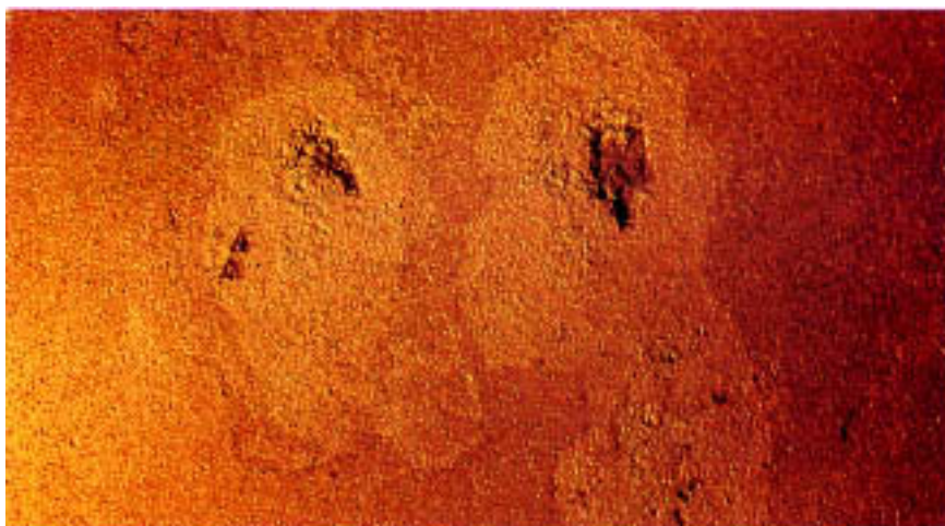
Figure 6.26 Small, pitlike depressions near the center of lightly etched regions. Each lightly etched region was covered by a gelatinous soap deposit in service. Note how the deeper, more localized metal loss occurred away from the lightly etched border.
