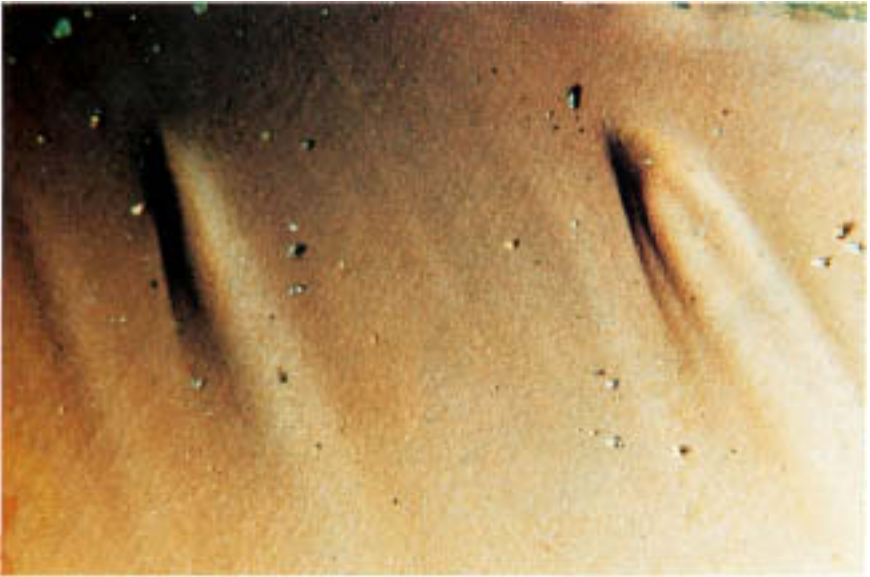
Figure 11.2 Comet-tail erosion patterns on copper. (Magnification: 15 \times .)
