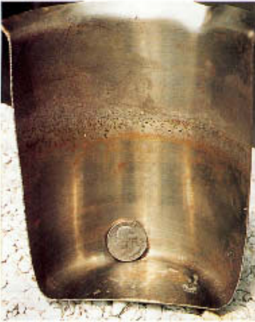
Figure 2.7 Severe waterline attack in stainless steel beaker. The beaker contained a chlorinated biocide tablet in water over a weekend. Perforations occurred in 40 hours or less, giving a minimum corrosion rate of 4380 mils (11.1 cm) per year at the perforations.
