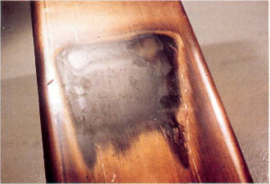
Figure 1.6 Dark oxide and deposit lobes on a copper continuous caster mold from a steel-making operation. Since heat transfer is high, even small amounts of deposit are unacceptable.
