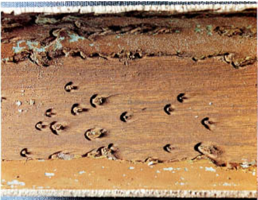
Figure 11.1 Horseshoe-shaped depressions on the internal surface of a brass heat exchanger tube.
