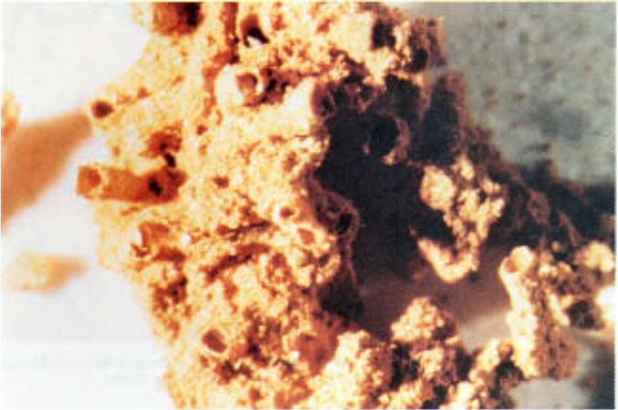
Figure 6.17B Close-up of small tubelike “casts.” More than 50% by volume of the surrounding material is composed of these casts.
