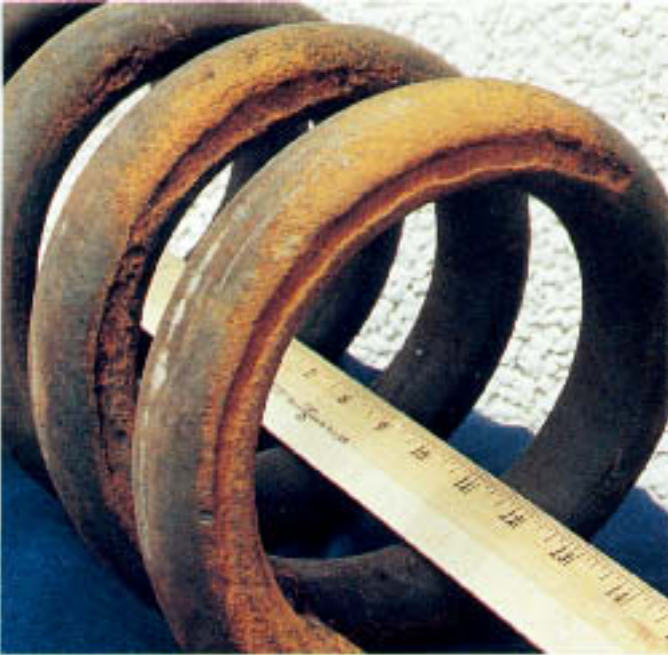
Figure 7.13 Vertical carbon steel gas cooler with grooving at bottom of the last three coils. Carbonic acid-containing condensate attacked.
