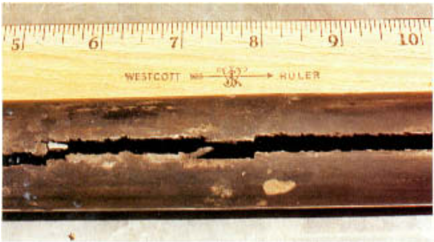
Figure 9.2 Longitudinal stress-corrosion cracks in a heat exchanger tube; the broad gap between the crack faces reveals that high-level residual hoop (circumferential) stresses from the tube-forming operation provided the stress component required for SCC.
