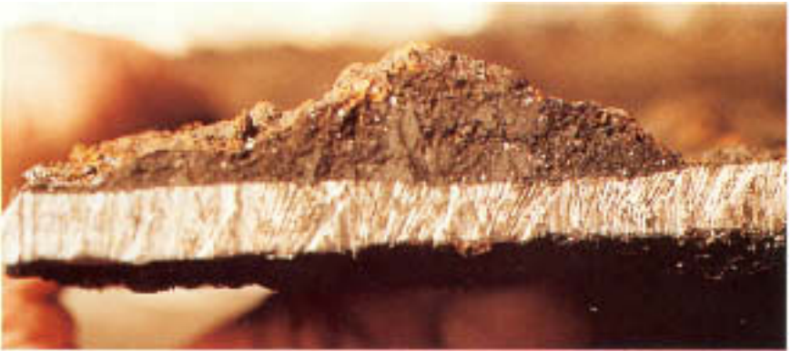
Figure 3.10 Large-diameter steel pipe wall cross section. Note the very shallow, broad depression beneath the tubercle. (Courtesy of National Association of Corrosion Engineers, Corrosion '91 Paper No. 84 by H. M. Herro.)
