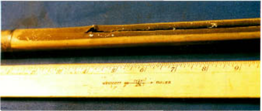
Figure 11.9 Erosion-corrosion damage on the surface of a brass tube facing the steam inlet nozzle.
