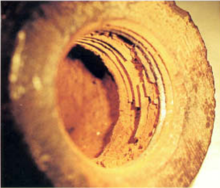
Figure 2.19 Gray cast iron elbow showing thread wastage.
