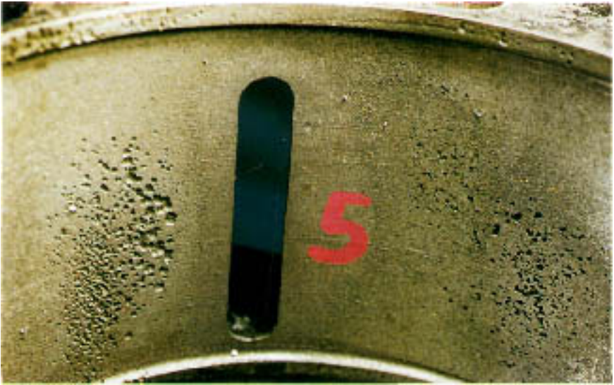
Figure 12.11 Zones of cavitation damage segregated to both sides of a vertical opening.
