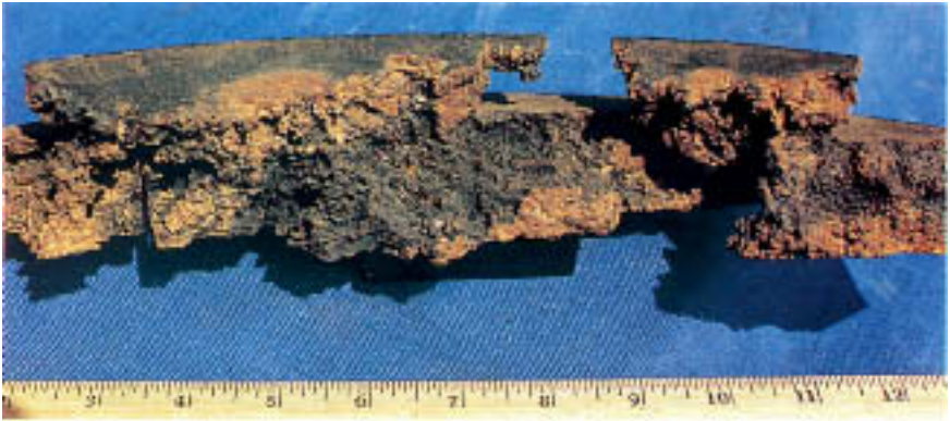
Figure 12.13 Severe damage to a cast iron pump component.
