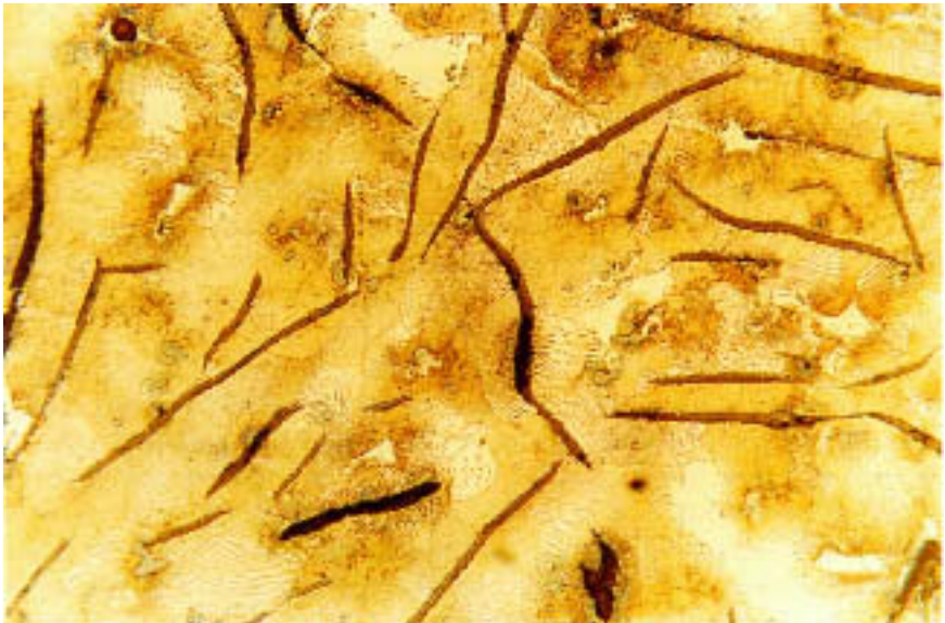
Figure 17.1 Flakes of graphite embedded in a matrix of iron (gray cast iron).
