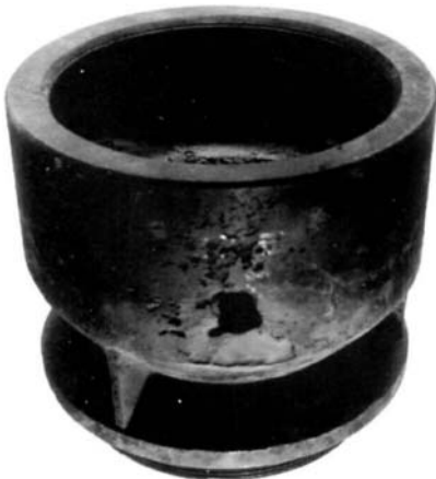
Figure 17.16 Pump casing as received. Note the large perforation near the center.
