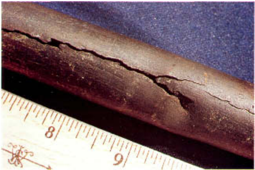
Figure 6.1 Stress-corrosion cracking of a brass condenser tube caused by ammonia from decomposing slime masses lodged on internal surfaces.
