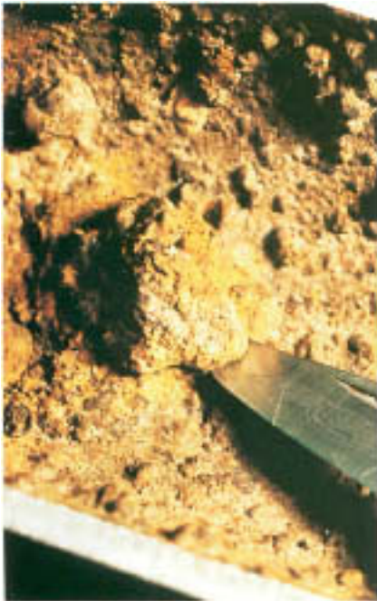
Figure 3.17 Intact tubercle showing physical integrity after removal from surface in Figs. 3.15 and 3.16.
