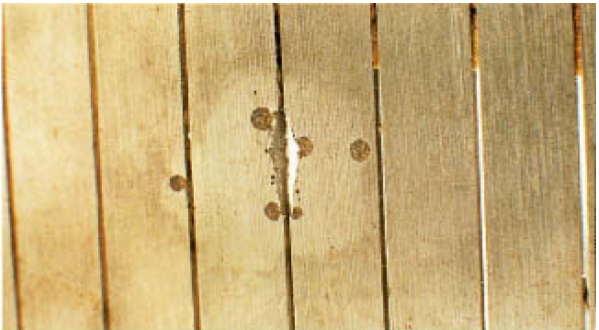
Figure 6.4B As in Fig. 6.4A. Note the smooth hemispherical pit contours and the tendency of the pits to cluster together.
