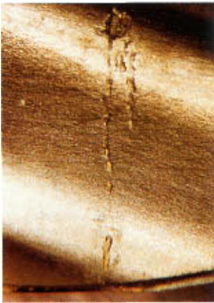
Figure 2.24 Cracklike corrosion site at apex of corrugation.
