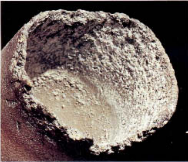
Figure 8.3 General wastage of an aluminum water manifold from a diesel engine cooling system. Note the generally wasted internal surface due to concentrated caustic and the presence of white deposits and corrosion products.
