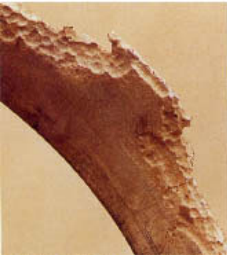
Figure 8.13 As in Fig. 8.12, but a threaded portion of the annealing sleeve. Note the heavy caustic deposits.
