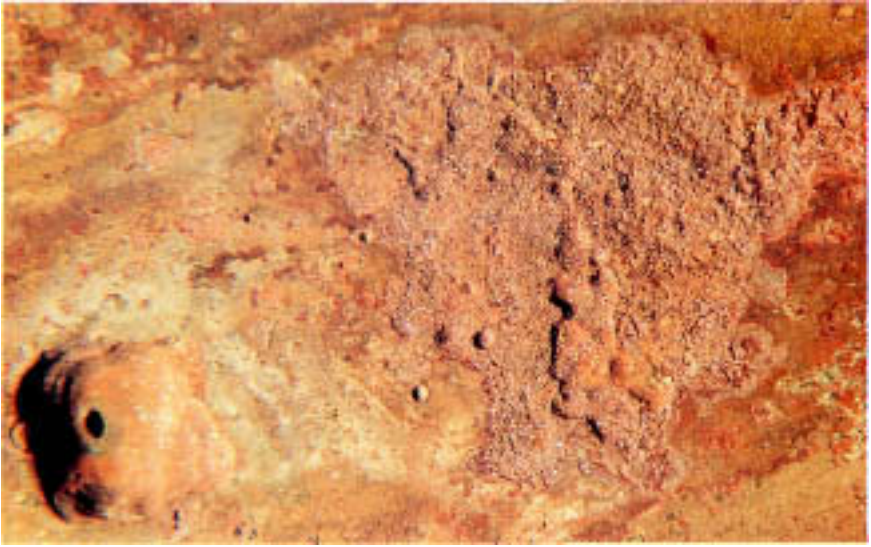
Figure 11.19 Perforated pit downstream of an arrowhead-shaped area of corrosion. (Magnification: 7.5 \times .)
