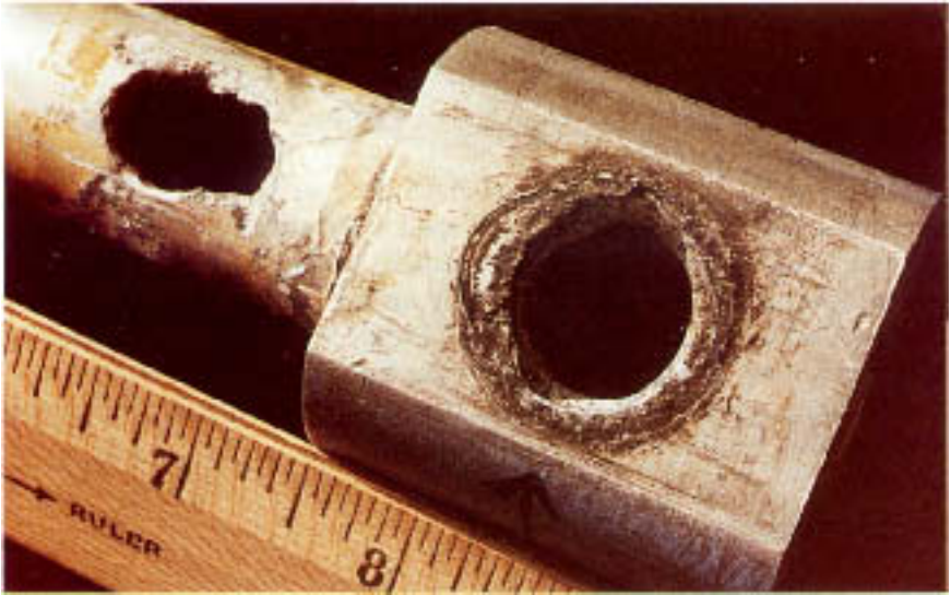
Figure 8.11 An aluminum cooling water conduit severely attacked by a caustic in service. The large circular hole in the machined face is corroded around its edges. The elliptical hole between the 6- and 7-in. ruler markings was formed by corrosion penetrating the conduit wall.
