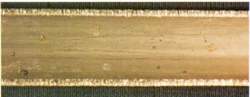
Figure 6.23B As in Fig. 6.23A, but with deposits removed to show pits.
