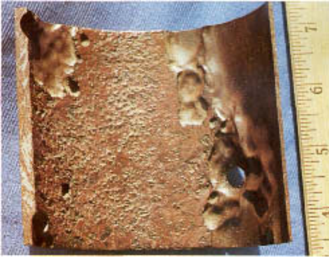
Figure 7.11 Smooth attack on carbon steel by carbonic acid. Note the vivid red color of hematite, indicating high oxygen concentrations.
