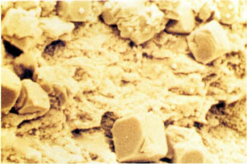
Figure 4.19 Scanning electron microscope picture of cuprous oxide crystals as shown in Fig. 4.18. Note the partial octahedral symmetry.
