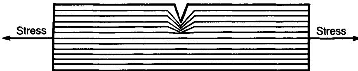
Figure 10.4 Schematic representation of localized increase in stress at a surface discontinuity.
