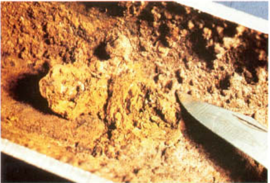
Figure 3.15 Knife dislodging a dry tubercle from a steel pipe surface.
