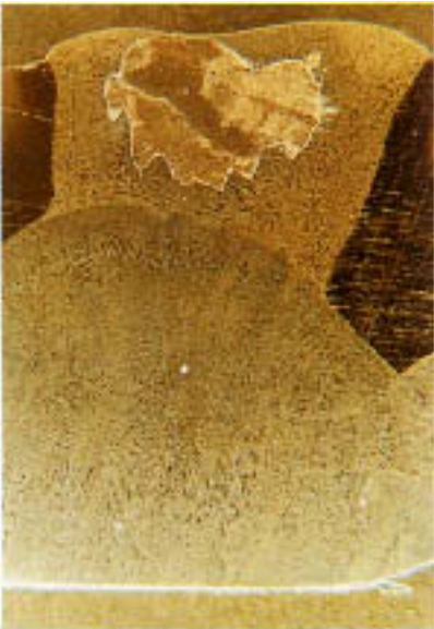
Figure 15.5 Cavity in weld bead covered by thin skin of weld metal (cross section). (Magnification: 7.5 \times .)
