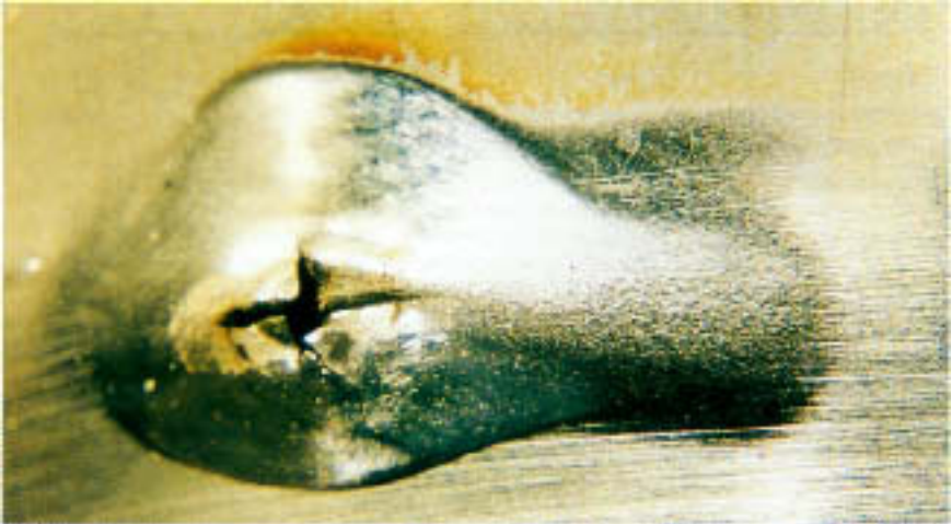
Figure 11.22 Close-up of perforated gouge shown in Fig. 11.21. (Magnification: 7.5×.)
