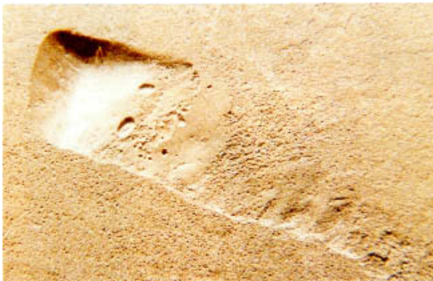
Figure 11.13 Erosion site resulting from lodgement of a foreign body inside a tube. (Magnification: 8 \times .)
