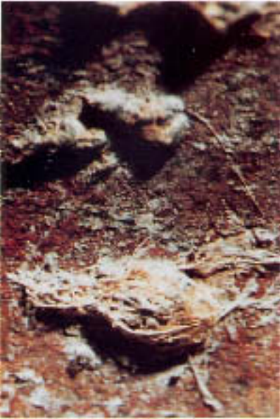
Figure 6.24A Small mounds of deposit entrapped by seed hairs that stuck to surfaces.
