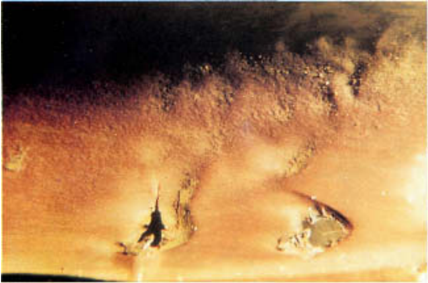
Figure 11.25 Erosion depressions and perforations at inlet ends of a brass tube.
