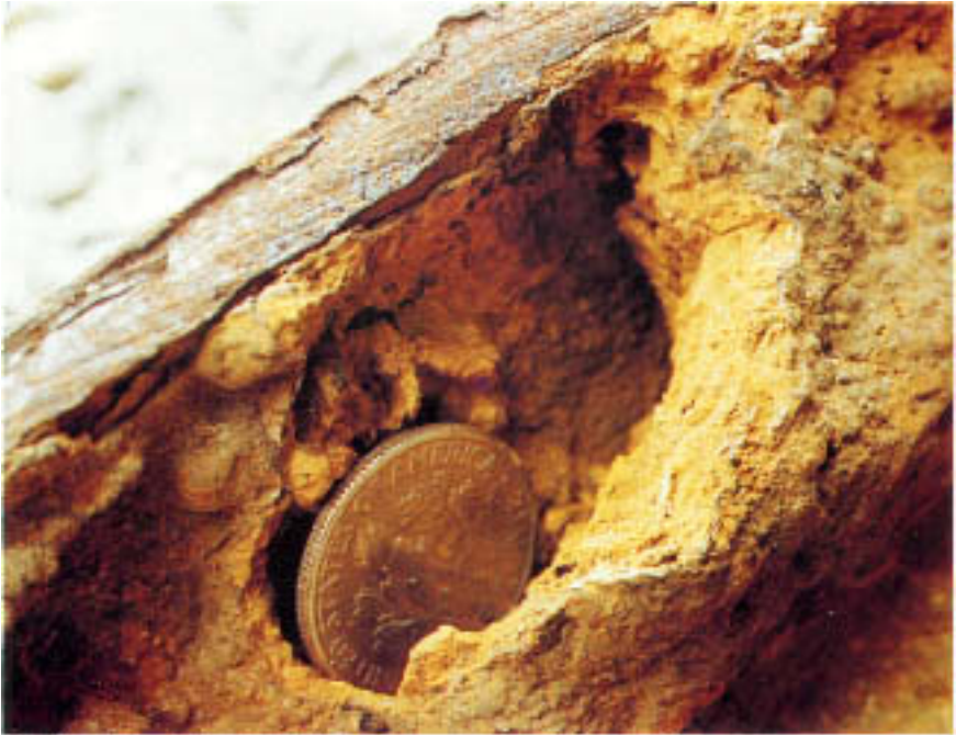
Figure 3.8 Large tubercle broken open to reveal the internal cavity. The cavity is filled with fluid in service.
