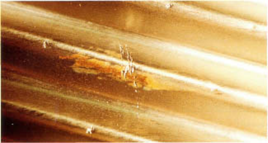
Figure 2.24 Cracklike corrosion site at apex of corrugation.
