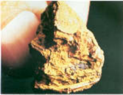
Figure 3.16 As in Fig. 3.15 but tubercle cap is completely dislodged.
