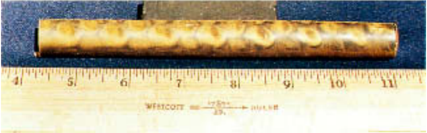
Figure 11.34 A pattern of erosion spots on the external surface facing the turbine exhaust inlet.
