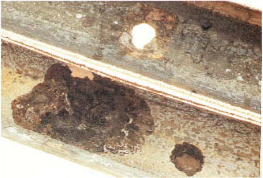
Figure 4.20 Sulfide deposits (dark patches) on longitudinally split brass heat exchanger tube. Note the perforation where wastage penetrated the tube wall. Sulfide was spalled after perforation by escaping fluids.
