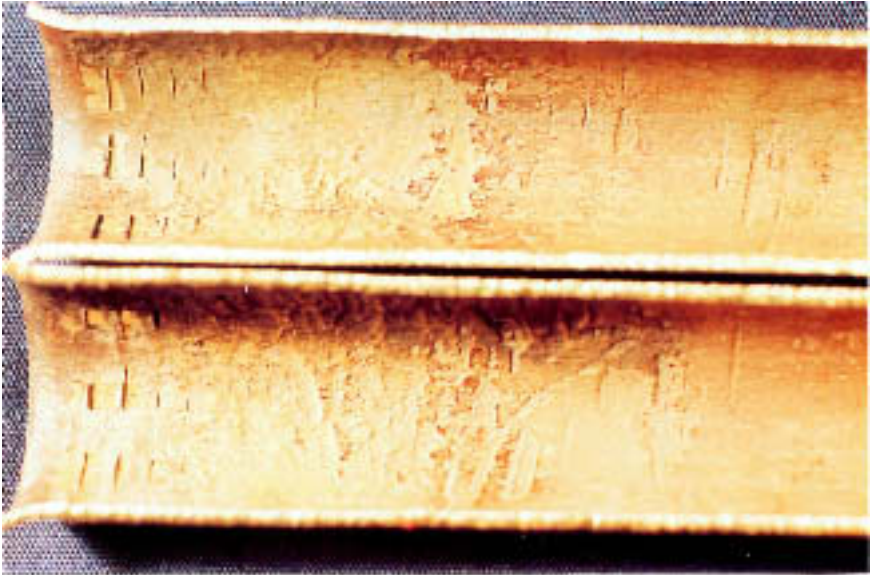
Figure 11.7 Metal loss on the internal surface at an inlet end (equally spaced circumferential gouges near the tube end were created during tube removal).
