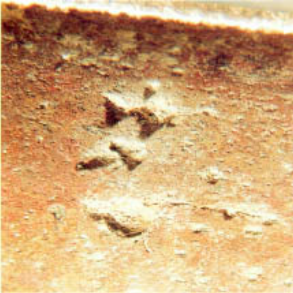
Figure 11.20 Elongated mounds of fibrous debris attached to the internal surface. (Magnification: 7.5 \times .)
