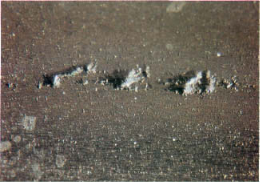
Figure 14.7 Shallow, aligned gouges on the internal surface. (Magnification: 6.5 \times .)
