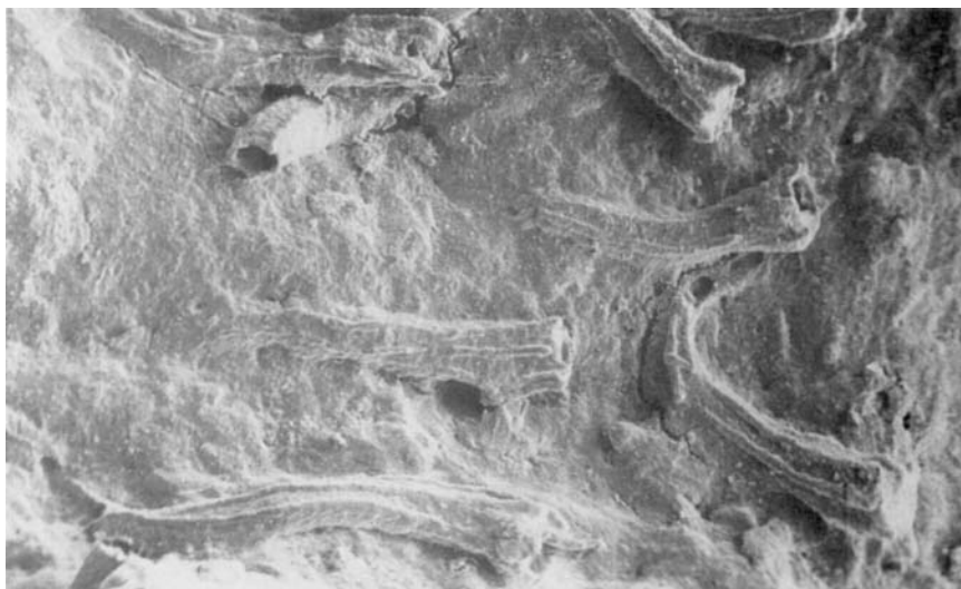
Figure 6.25 Low-power scanning electron micrograph of small tubelike organisms in Figs. 6.17 and 6.20. Note how all organisms (except one) point into the direction of flow.
