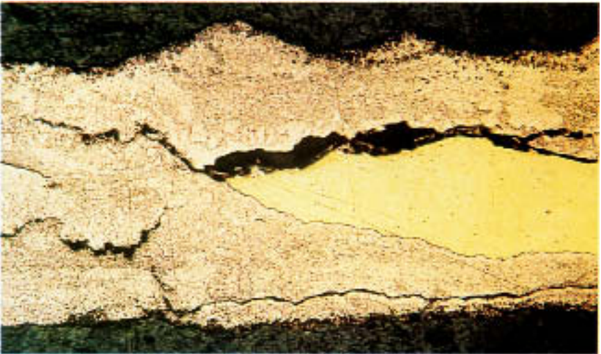
Figure 13.2 Layer-type dezincification of a thin brass plate. The 0.019-in. (0.048-cm) plate is shown in cross section. The dezincified layers converge toward the plate edge. Note the porosity of the dezincified metal.
