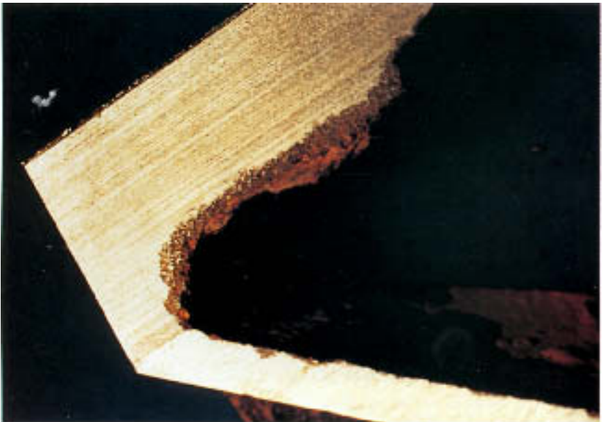
Figure 17.14 Cross section through the pump housing wall. Note the black and brown graphitic corrosion-product layer near the center of the photo.
