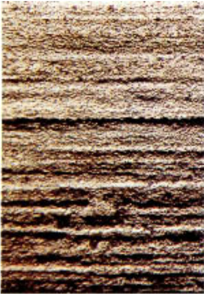
Figure 7.8 Striations on the internal surface of admiralty brass condenser tube after acid cleaning. (Magnification: 15 \times .)
