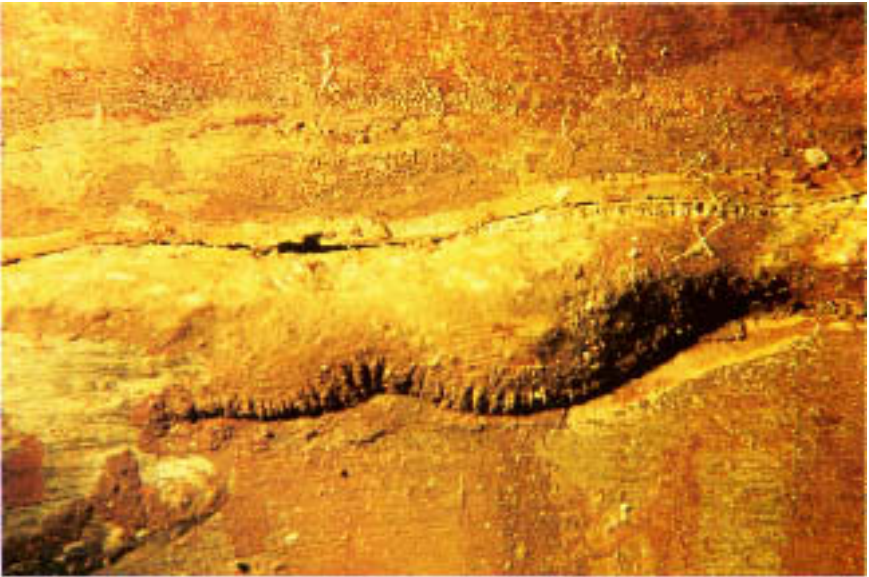
Figure 15.10 Unfused seam along edge (top) of weld bead. (Magnification: 7.5 \times .)
