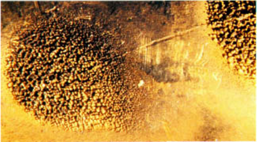
Figure 11.35 A small forest of erosion cones typical of the appearance of each site. (Magnification: 7.5 \times .)
