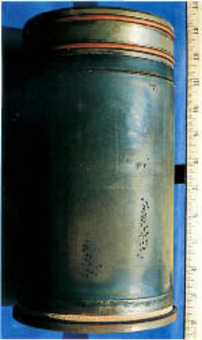
Figure 12.9 Typical vertical alignment of cavities resulting from cavitation damage in a diesel engine cylinder liner.
