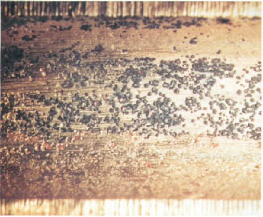
Figure 4.7 Small, manganese-rich nodules on a 90:10 cupronickel condenser tube. Note the small pits beneath each nodule. (Courtesy of National Association of Corrosion Engineers; Andy Howell Public Service of Colorado, Corrosion '89 Paper No. 197 by H. M. Herro.)
