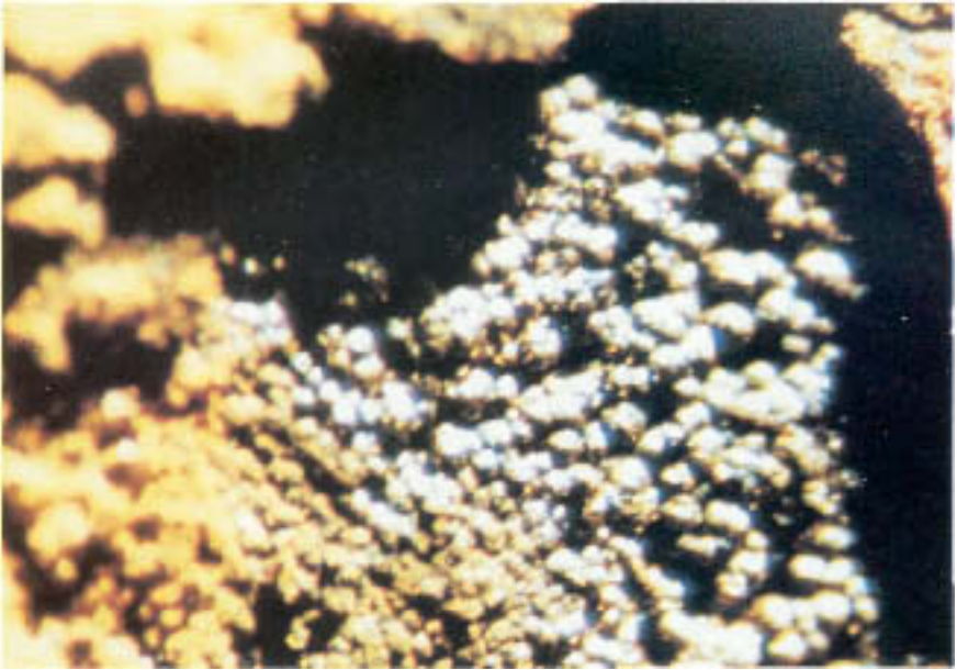
Figure 3.7 Siderite ( \text{FeCO}_3 ) nodules inside a tubercle revealed by breaking open the magnetite shell. (Courtesy of National Association of Corrosion Engineers, Corrosion '89 Paper No. 197 by H. M. Herro.)
