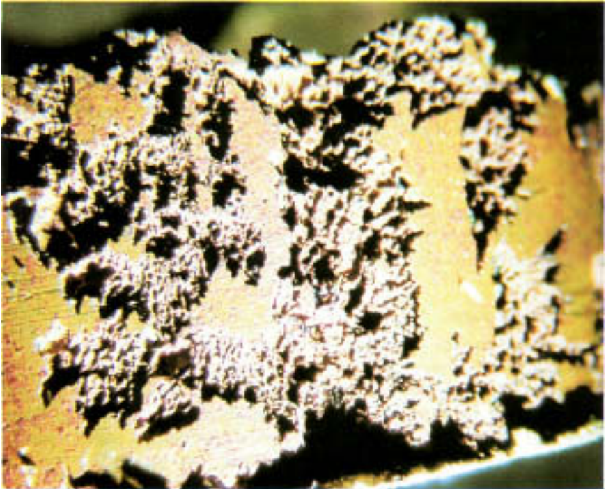
Figure 7.1 Brass condenser tube inlet end severely corroded by an acid upset involving sulfuric acid.
