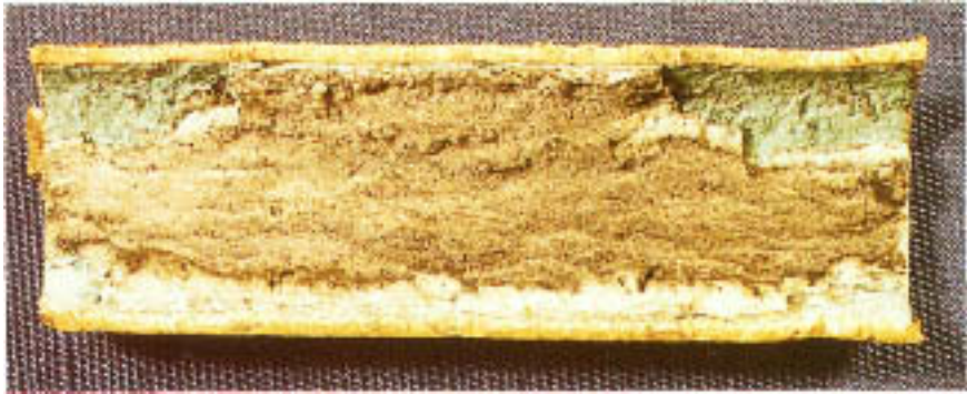
Figure 4.30B As in Fig. 4.30A. Note the light-colored deposits intermixed with bluish-green corrosion products.
