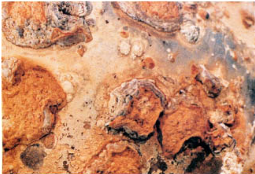
Figure 3.32 Large tubercles on gray cast iron pump housing.
