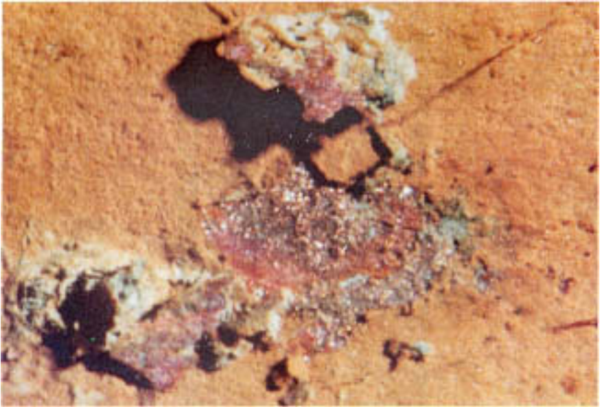
Figure 4.25 As in Figs. 4.23 and 4.24. Corrosion product mound broken open to reveal sparkling cuprous oxide crystals.
