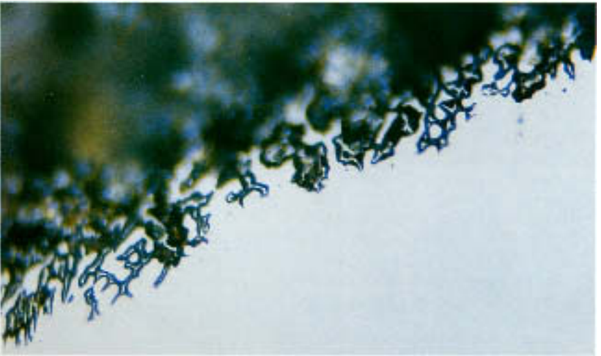
Figure 15.23 Preferential corrosion of Phase II; Phase I remains unaffected. (Magnification: 500 \times , unetched.)
