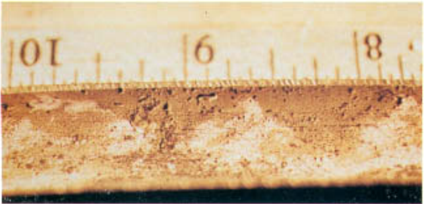
Figure 4.8 Pitting on internal surface of a brass condenser tube revealed by removal of manganese-rich deposit.
