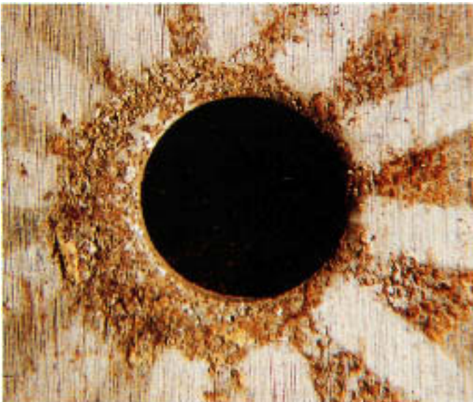
Figure 2.23 Shallow pitting in crevice areas on a 304 stainless steel coupon exposed to a misting atmosphere. Note the relatively clean areas where the washer teeth contacted the coupon surface. (Magnification: 7.5 \times .)
