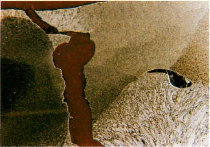
Figure 15.28 Cross section of fracture along the weldment showing subsurface porosity. Note that the fracture path runs through a large pore. (Magnification: 7 \times .)
