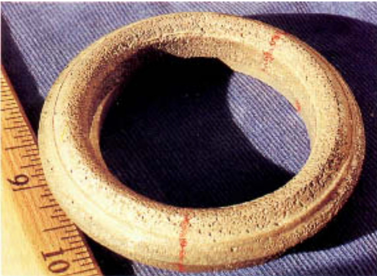
Figure 8.4 Corroded aluminum-alloy casting valve seat. The seat was in contact with water having a pH between 9 and 10 for 3 months. Red marks were drawn on the surfaces to assist metallographic preparation.
