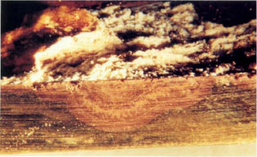
Figure 13.9 Stratified copper corrosion product in plug-type dezincification.
