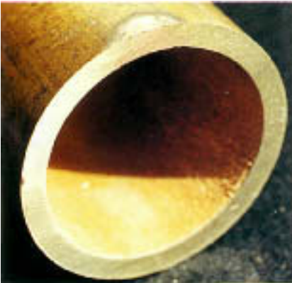
Figure 13.8 A brass tube showing plug-type dezincification. The white patch above the plug on the external surface was caused by dissolved solids, concentrated by evaporation of water leaking through the porous dezincified plug.
