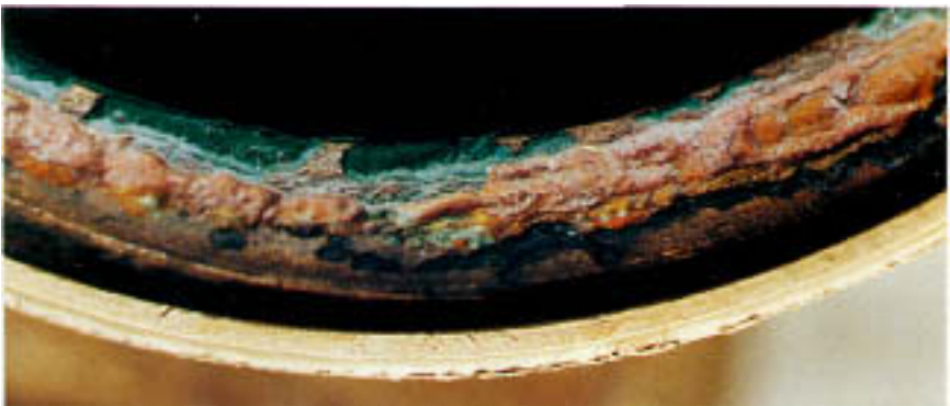
Figure 13.6A Red, dezincified gasketed surface of a cast valve throat. Note the partial spalling of the copper corrosion product.
