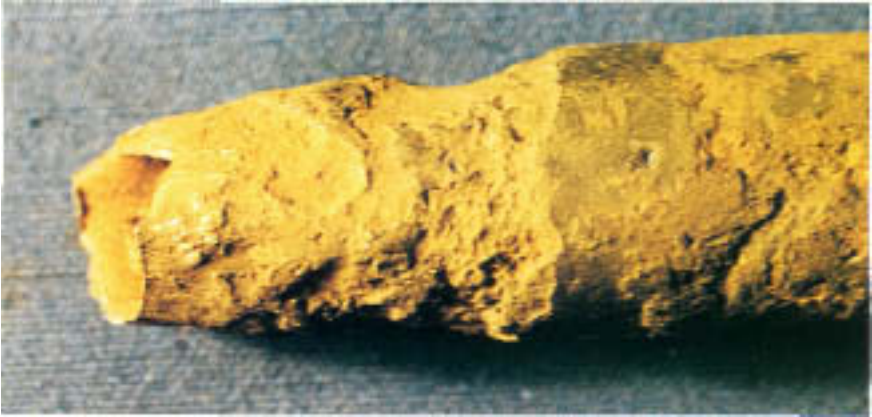
Figure 2.27 Close-up of severely thinned heat exchanger tube in a baffle.
