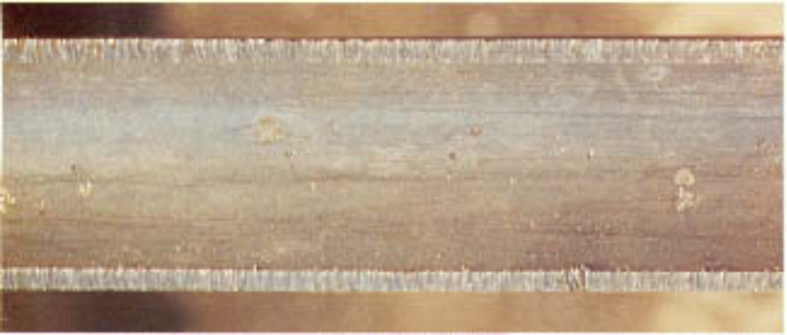
Figure 4.10B As in Fig. 4.10A, with deposits removed to show pitting.
