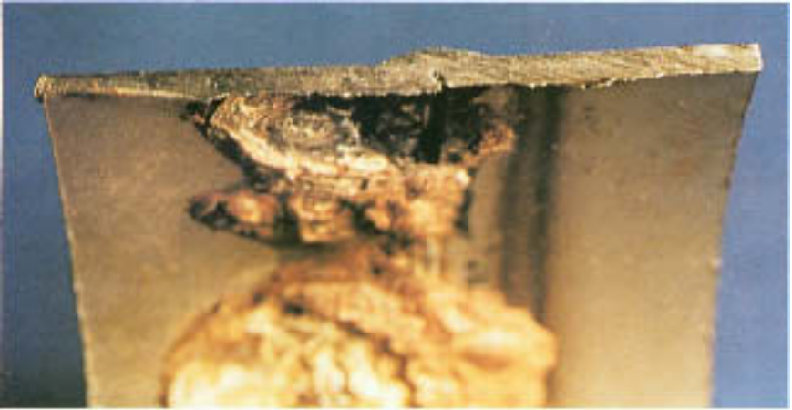
Figure 6.9B Longitudinal cross section showing a pit tunneling into an incompletely closed weld seam.
