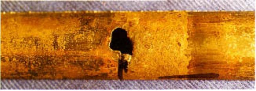
Figure 16.7 External surface at the same location as Fig. 16.7. Note location of baffle contact surface relative to the perforation.
