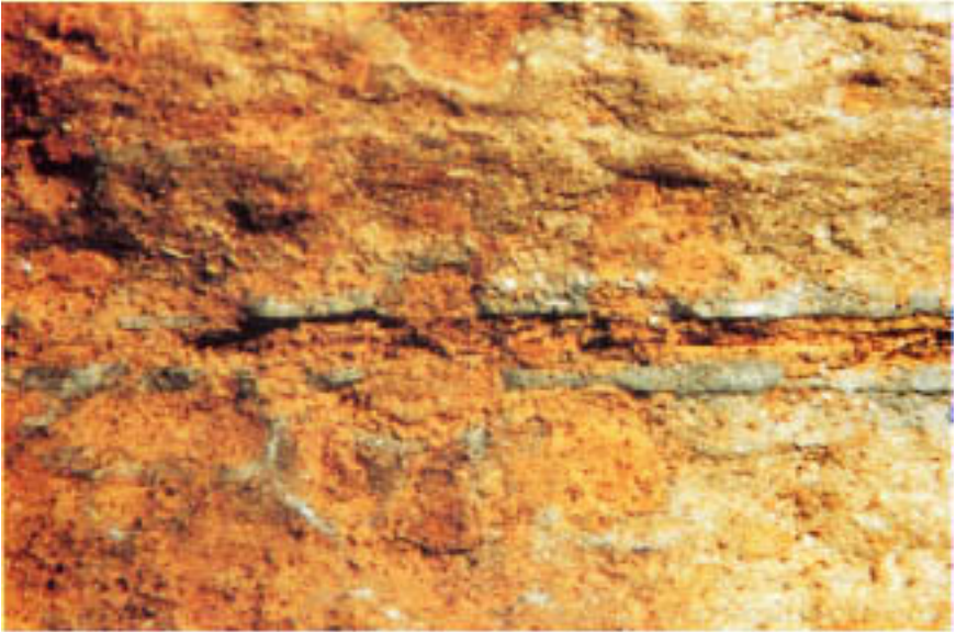
Figure 5.15 Rough internal surface contour of the tube shown in Fig. 5.14. Note the preferential attack on the weld seam. (Magnification: 7.5 \times .)
