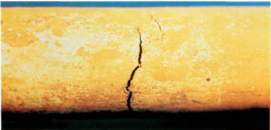
Figure 9.22 Transverse cracks originating on the external surface.
