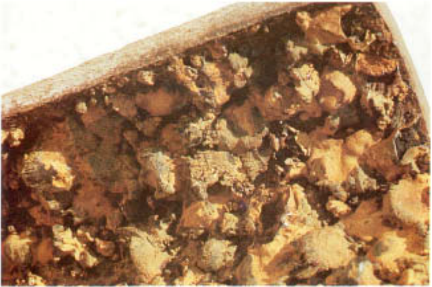
Figure 3.14 Small, hard tubercles on an essential service water system pipe in a nuclear utility.
