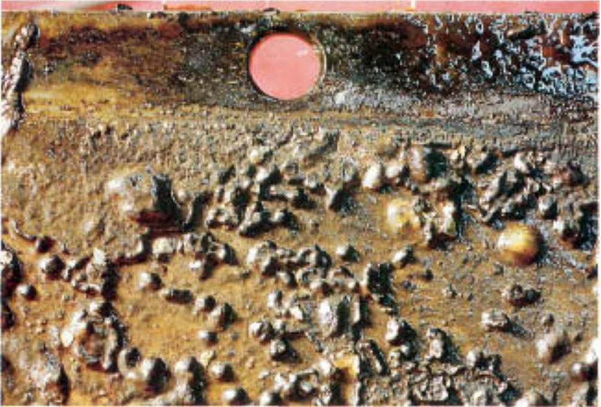
Figure 4.27A Mild steel coupon removed from a rolling mill cooling tank. Note the thick greasy deposits.
