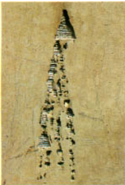
Figure 7.6 As in Fig. 7.5. Note the multiple parallel striations within the larger grooves following stress lines remaining from the original pipe manufacturing processes.
