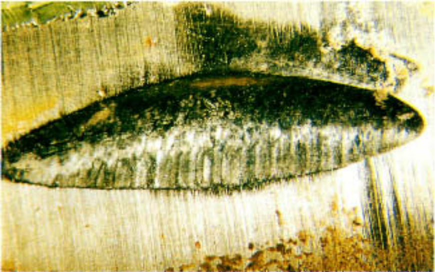
Figure 11.23 Elliptical gouge on internal surface \frac{1}{2} in. from inlet end. The long axis parallels the longitudinal tube axis. (Magnification: 7.5×.)
