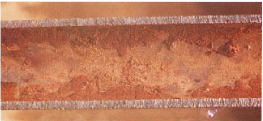
Figure 4.10A Deposits on a 316 stainless steel heat exchanger tube.
