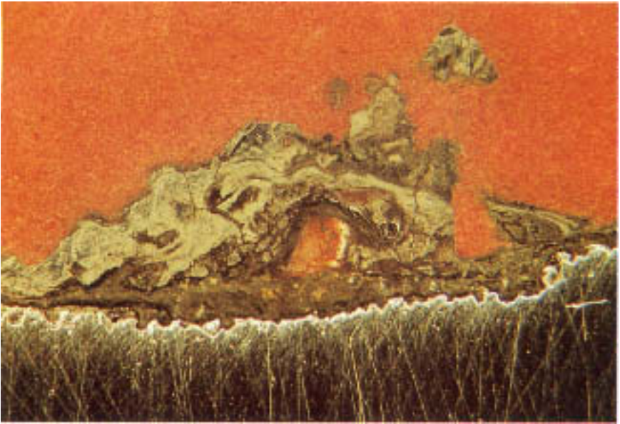
Figure 3.9 Small tubercle cross section. The steel surface is at the bottom, and the red material is an epoxy mounting medium. Note the small, shallow central cavity. (Magnification: 7.5 \times .)
