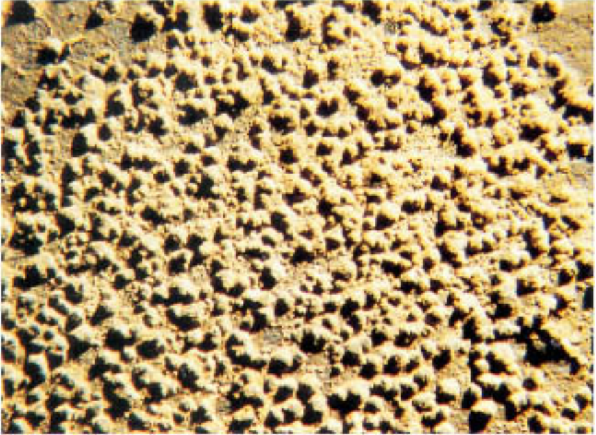
Figure 3.28 Many incipient tubercles formed on a steel battle plate in 2 weeks. (Magnification: 7.5 \times .) (Courtesy of National Association of Corrosion Engineers, Corrosion '89 Paper No. 197 by H. M. Herro.)
