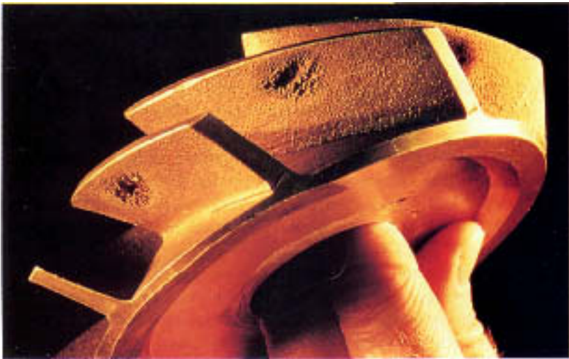
Figure 12.8 Cavitation damage repeated on successive elements of a bronze impeller.
