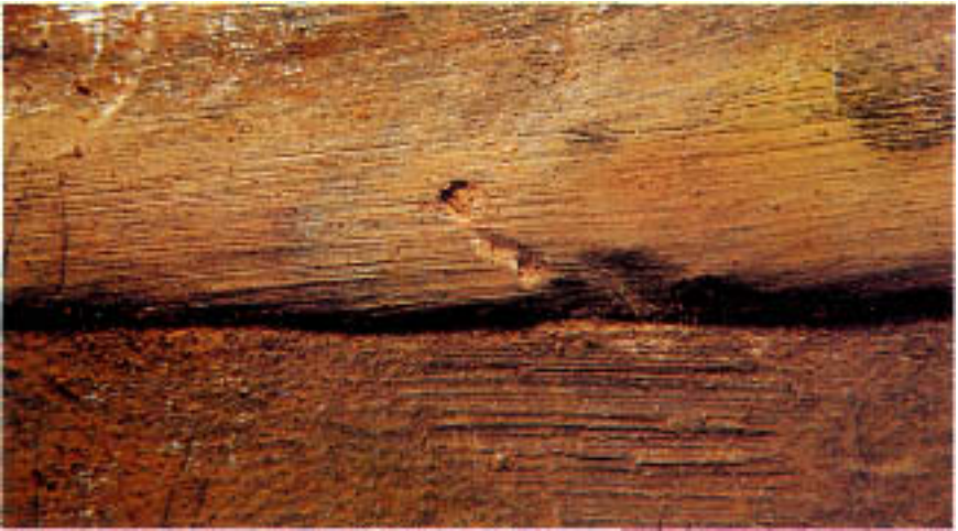
Figure 15.6 Weld bead site at which radiography indicated a large pit. (Magnification: 7.5 \times .)
