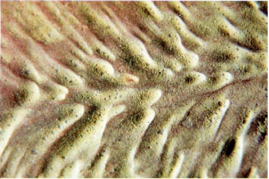
Figure 7.25 Smooth, wavelike contour in a region of general metal loss on copper due to carbonic acid. The groove patterns indicate channeling of corrosive fluids by flow. (Light is coming from the reader's right.)
