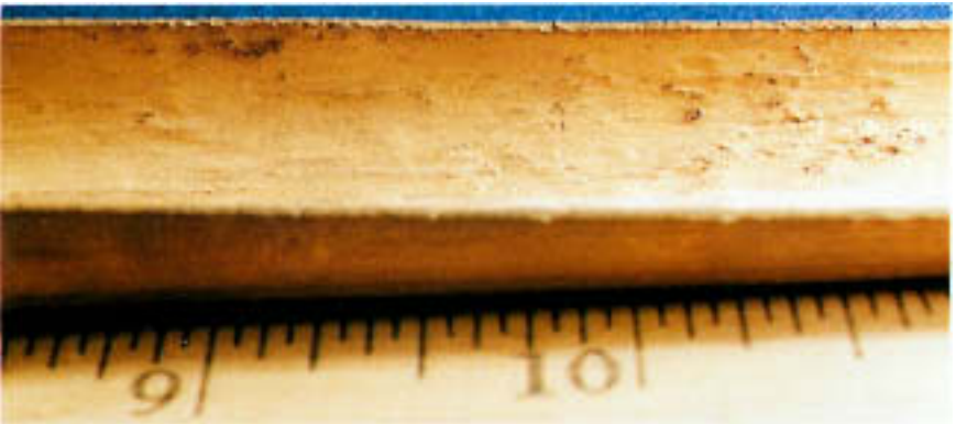
Figure 11.15 Relatively smooth, lightly rolling contour of the internal surface at the inlet end.
