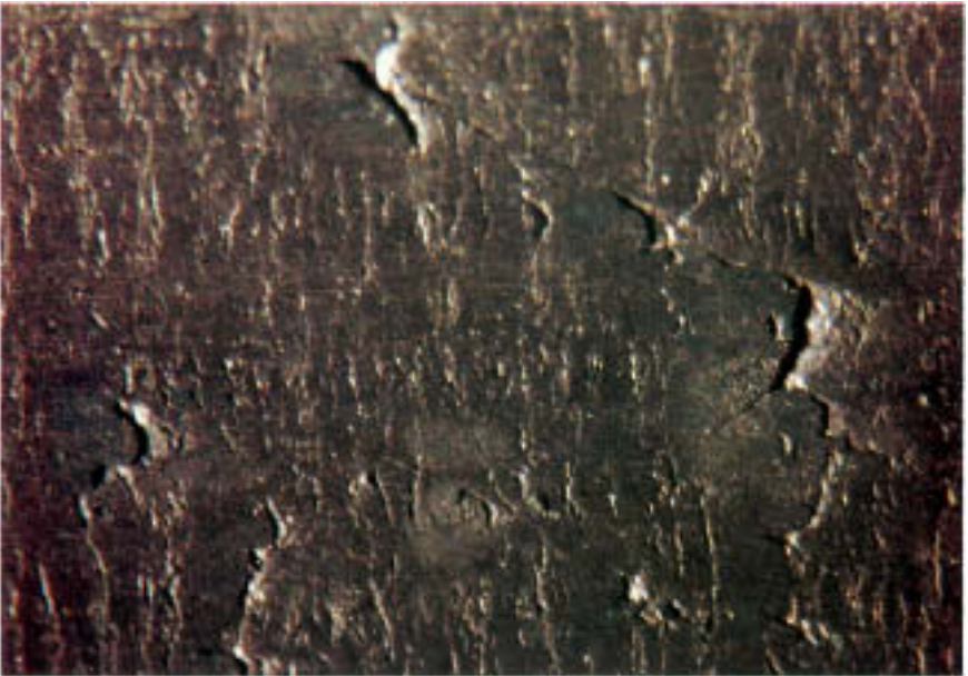
Figure 14.8 Broad patches of smeared metal aligned longitudinally along the internal surface. (Magnification: 6.5 \times .)
