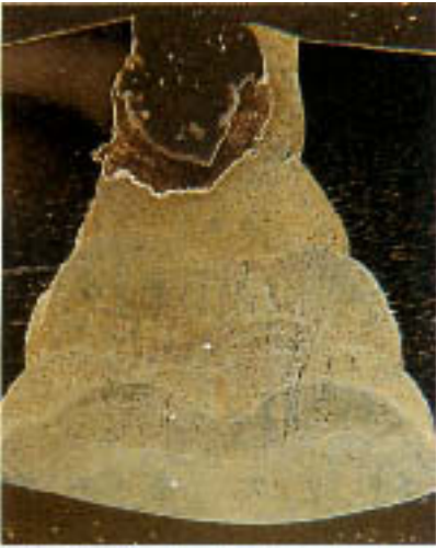
Figure 15.3 Corrosion confined to weld bead (cross section). (Magnification: 7.5 \times .)
