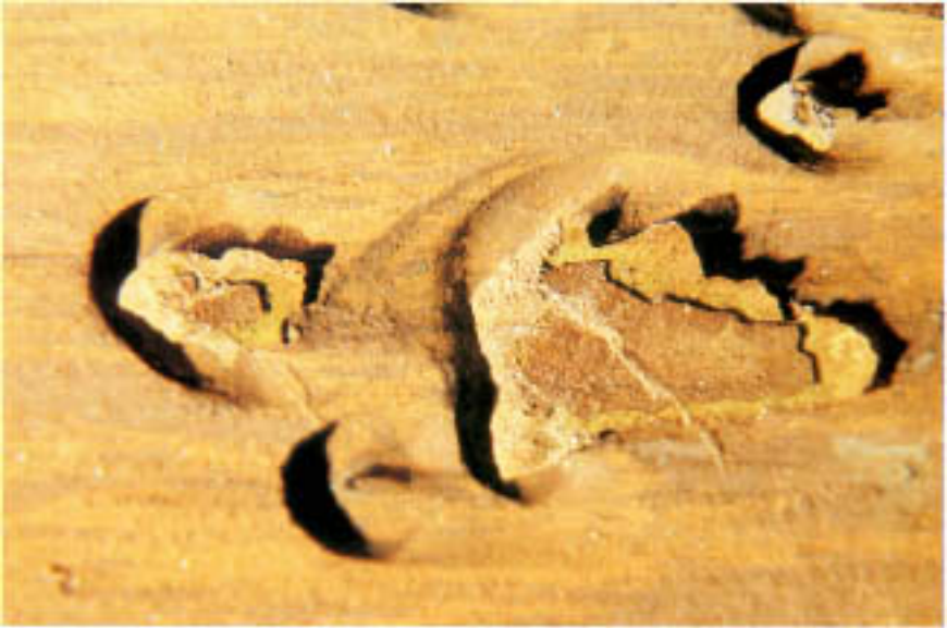
Figure 11.4 Deposits covering intact metal surfaces at sites of horseshoe-shaped erosion-corrosion depressions. (Magnification: 15 \times .)
