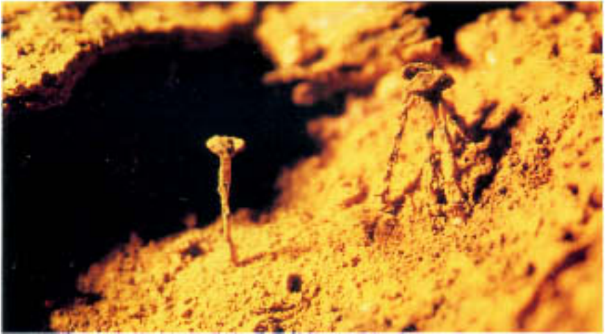
Figure 6.19 Small organisms found inside a tubercle. Each is about 0.05 in. (0.13 cm) high. The organisms have segmented, fibrous stalks and bivariate heads.
