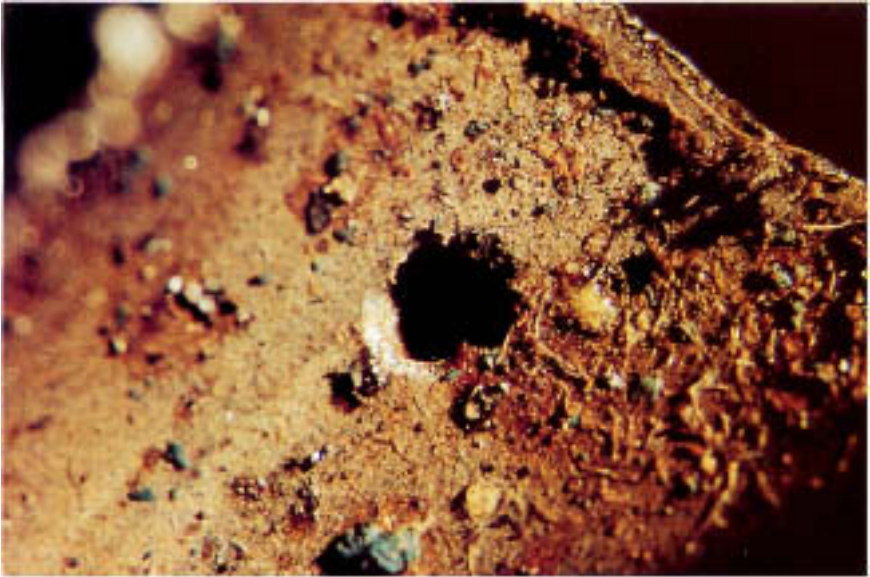
Figure 6.11 A \frac{1}{16} -in. (0.16-cm) diameter pit on the internal surface of a 316 stainless steel tube. Note the absence of significant corrosion products or deposits in the pit.
