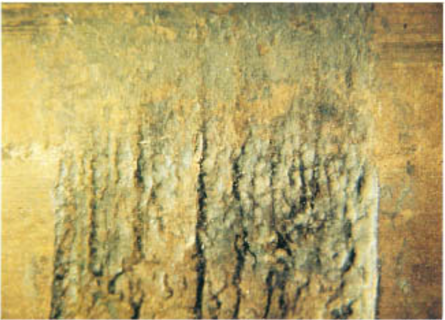
Figure 2.11 As in Fig. 2.10. Note the more severe attack at the bottom of the tube where the tube rested against its support. (Magnification: 7.5 \times .)
