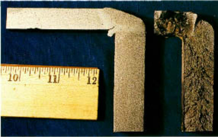
Figure 15.27 Fracture face (right) contrasted with corresponding, intact weldment. Note that the transition from a rough to a smooth fracture surface occurs abruptly at the junction of the weld metal with the base metal.
