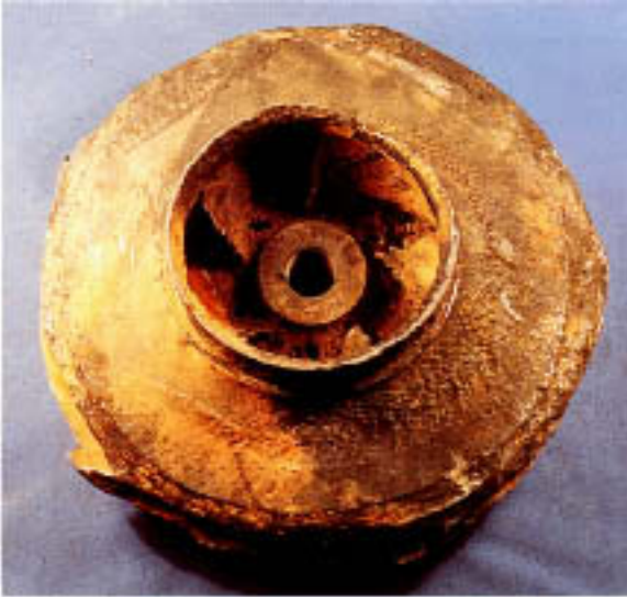
Figure 17.9 Pump impeller that has suffered erosion associated with graphitic corrosion.
