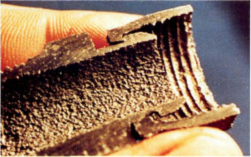
Figure 7.23A Free-machining carbon steel hose coupling after 2 months in a solution containing several percent oleic acid.
