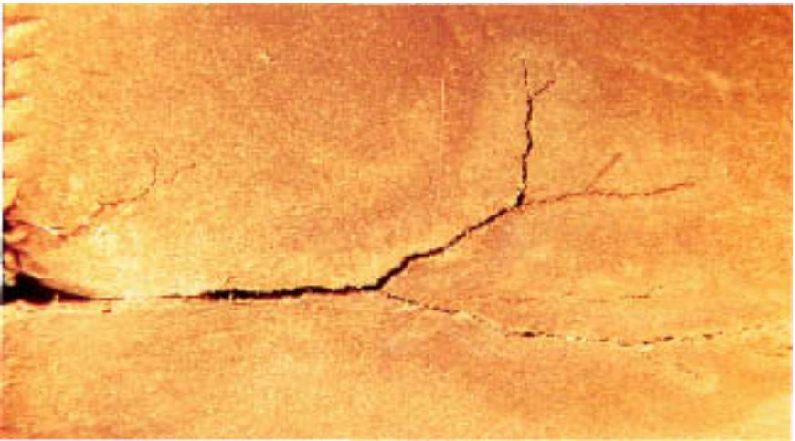
Figure 9.21 Branched, longitudinal cracks on the external surface. (Magnification: 7.5×.)
