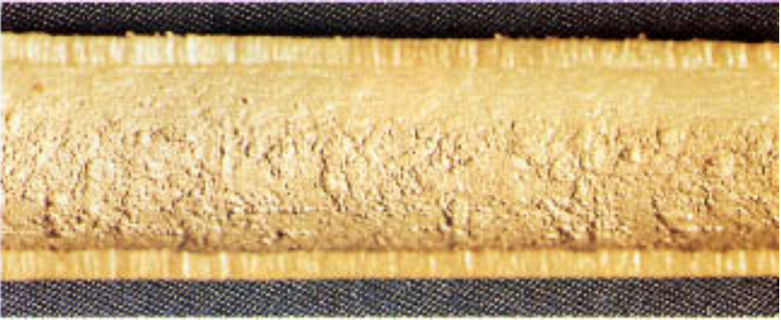
Figure 4.26 Internal surface of steel heat exchanger tube after removal of deposits. Note the mutually intersecting areas of metal loss.
