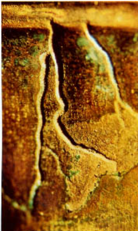
Figure 8.7 Small grooves on the tube shown in Fig. 8.6. Grooves are condensate rivulet paths cut into the tube surface. (Magnification: 10 \times .)
