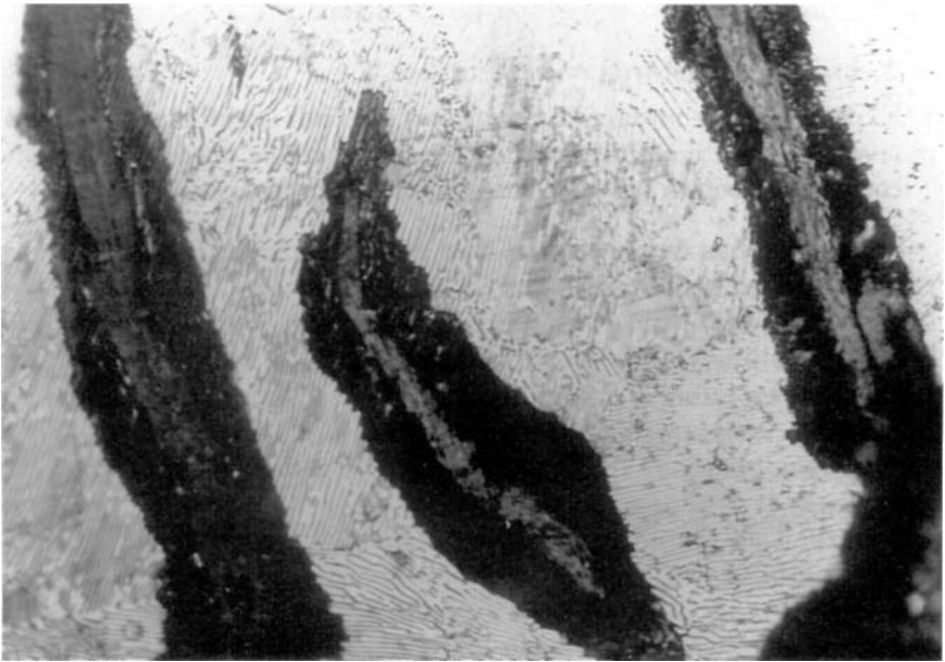
Figure 17.3 Graphite flakes surrounded by graphitically corroded iron. Bright background is uncorroded metal. (Magnification: 1000x.)
