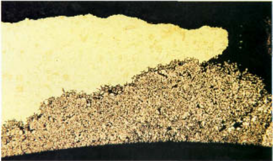
Figure 13.11B Porous copper corrosion products filling an internal surface depression. The edge of one crater seen in Fig. 13.11A is to the right.
