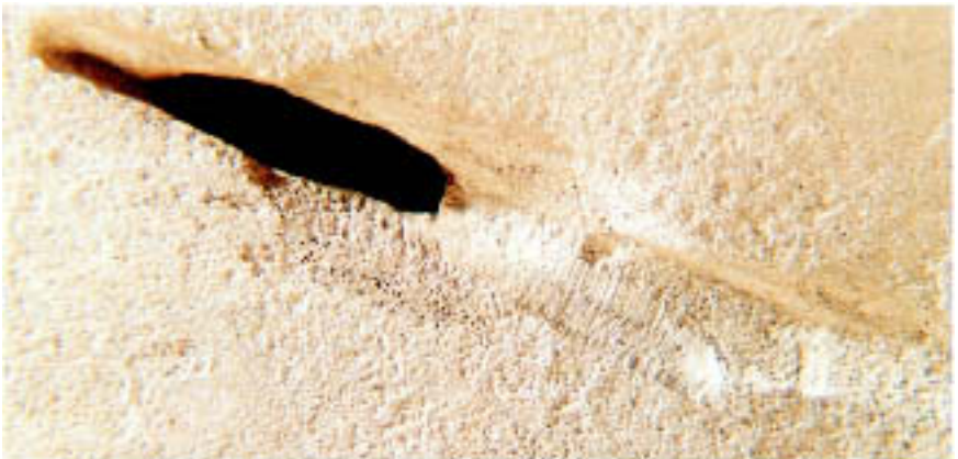
Figure 11.12 Erosion site resulting from lodgement of a foreign body inside a tube. (Magnification: 8 \times .)
