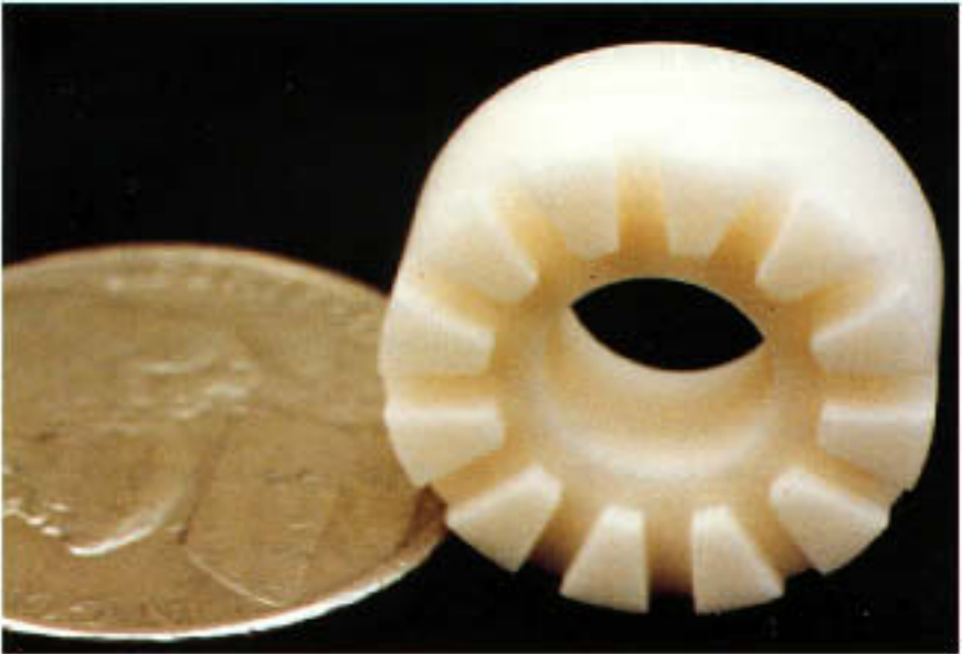
Figure 2.22 Crevice washer. The radially oriented, wedge-shaped washer teeth provide small areas between which crevices are formed.
