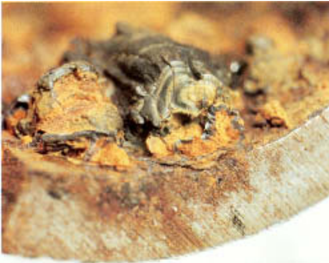
Figure 3.18 Multiple magnetite shells in a small tubercle. Multiple shells form due to successive fracture during growth. (Magnification: 2 \times .)
