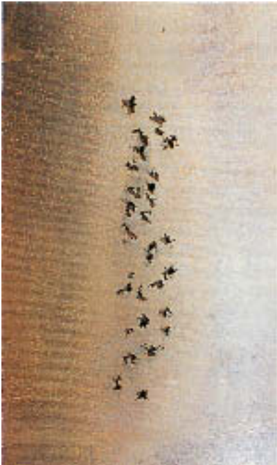
Figure 12.10 Jagged, cavernous pits typical of cavitation damage.
