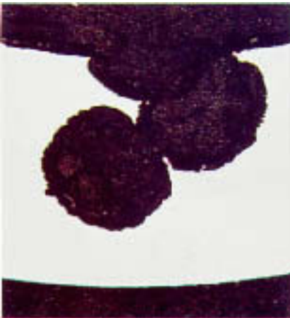
Figure 6.8 Scalloped, partially undercut pits in a cross section of a 316 stainless steel tube.
