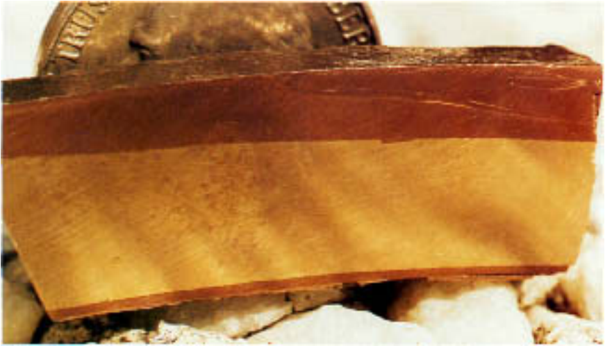
Figure 13.1 Layer-type dezincification on a brass casting. The red layers are uniformly corroded regions. The original yellow of the brass is visible in between.
