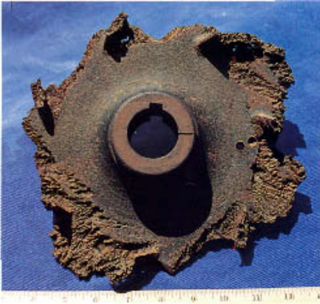
Figure 12.7 Cast iron pump impeller with severe cavitation damage.
