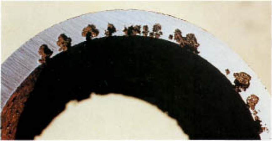
Figure 7.3 As in Fig. 7.2. Note the narrow pit mouths and the pronounced undercutting.
