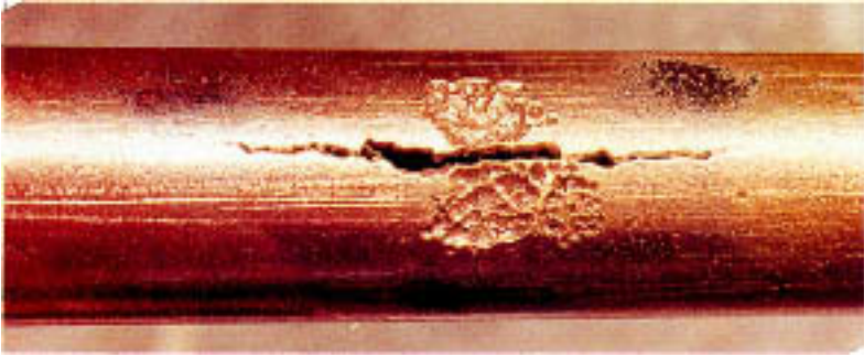
Figure 9.5 Stress-corrosion cracks associated with simple corrosion.
