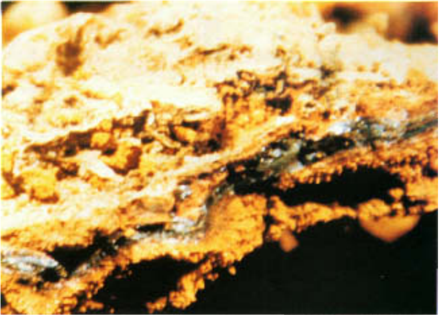
Figure 3.6 Tubercle cross section shows black magnetite-rich shell beneath deposit and hematite cap. Note the core material below the magnetite shell. (Magnification: 7.5 \times .) (Courtesy of National Association of Corrosion Engineers, Corrosion '89 Paper No. 197 by H. M. Herro.)
