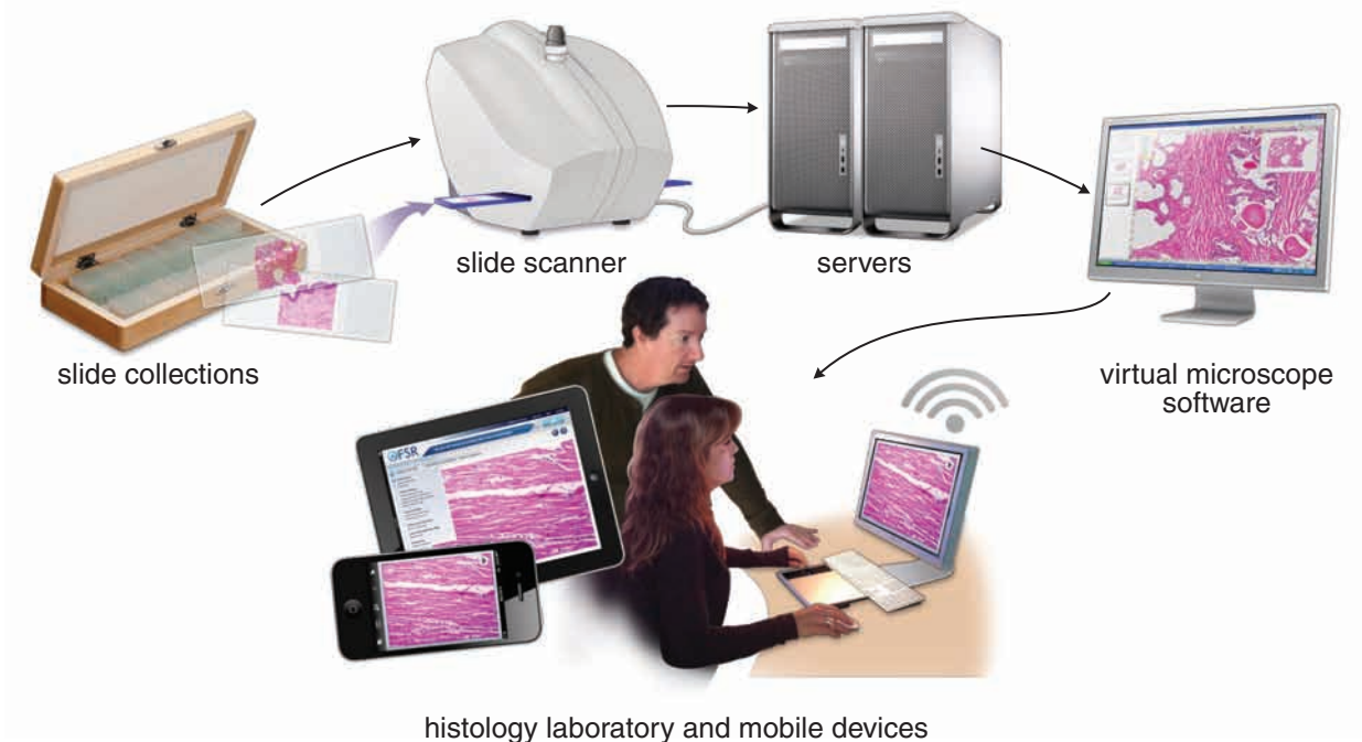
FIGURE 1.15 ▲ Virtual microscopy. Glass slides are scanned using a high-resolution automated slide scanner to create digital files that are stored typically in dedicated virtual microscopy servers. The virtual slide is a digital representation of a glass slide and can be displayed by using a specialized software viewer referred to as a virtual microscope. Virtual slides are distributed over a computer network or the Internet for remote viewing. Note that the virtual slides may be viewed individually or in groups on any mobile device, such as tablet computers or smartphones with virtual microscopy applications.
