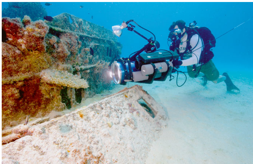
Fig. 11.2 Brett Seymour, NPS SRC, is using a high-definition stereoscopic 3D camera with hard-wire surface connection to record the details of a US Army landing craft in Saipan. (Photo: Lou Larmar, WHOI AVIL)
