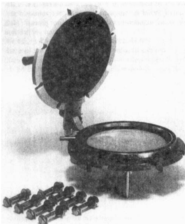
Figure 13.15 Pressure membrane extractor. (Photograph courtesy of Soilmoisture Equipment Corporation, Santa Barbara, CA.)
