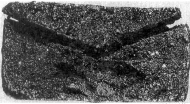
Figure 11.6 Passive-type failure of compacted clay till resulting from swelling in an oedometer ring.
