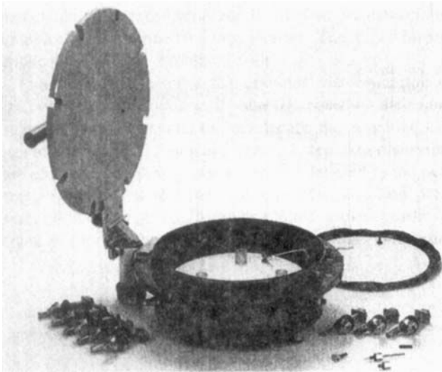
Figure 13.14 A 15 bar ceramic plate extractor (i.e., maximum applied matric suction is 1500 kPa). (Photograph courtesy of Soilmoisture Equipment Corporation, Santa Barbara, CA.)
