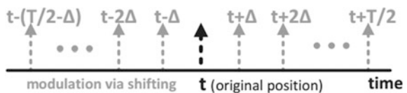
Fig. 6.4 Encoding time shift of beacon message for communication
