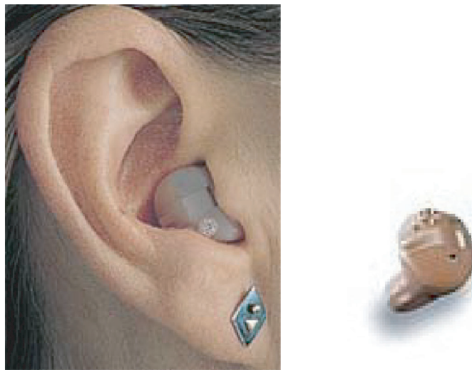
FIGURE 21: ITC style hearing aid with the device positioned further into the canal.
