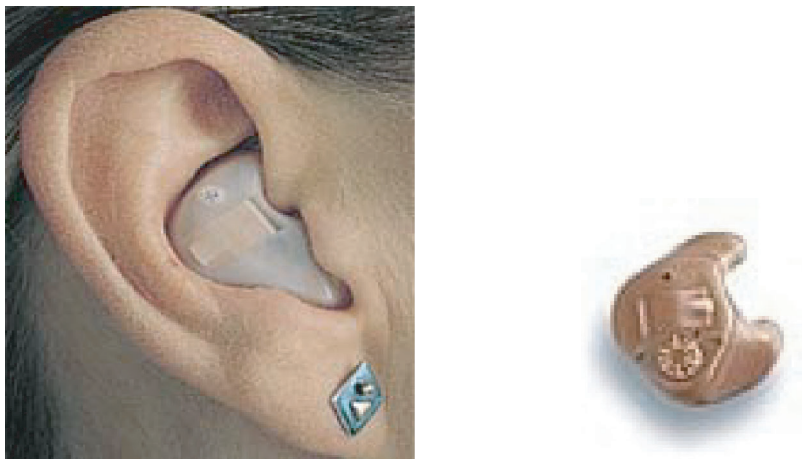
FIGURE 20: ITE style of hearing aid with the device easily accessible and removable.
