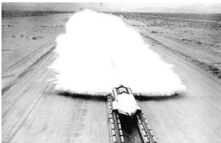
Fig. 7.2 SNORT Rocket Sled, NAWS China Lake, California. The four-mile supersonic track has created a cultural landscape, as sleds move at speeds up to Mach 4. Test tracks were also built at Edwards AFB but have been removed (U.S. Navy)
