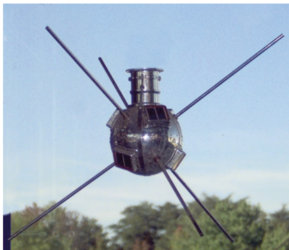
Fig. 1.1 Vanguard 1, launched March 17, 1958, and known as the “Grapefruit Satellite.” Vanguard 1 became the second artificial satellite successfully placed in Earth orbit by the United States. It was the first solar-powered satellite; just 152 mm (6 in) in diameter and weighing just 1.4 kg (3 lb) (NASA)
