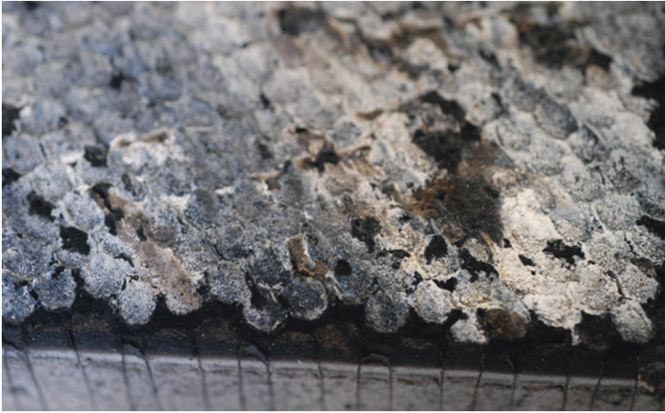
Fig. 5.4 Reinforced carbon–carbon (RCC) shield applied on the leading edges and nose of the shuttle orbiter (courtesy of Dr. Nathan Jacobs, NASA Glenn Research Center)
