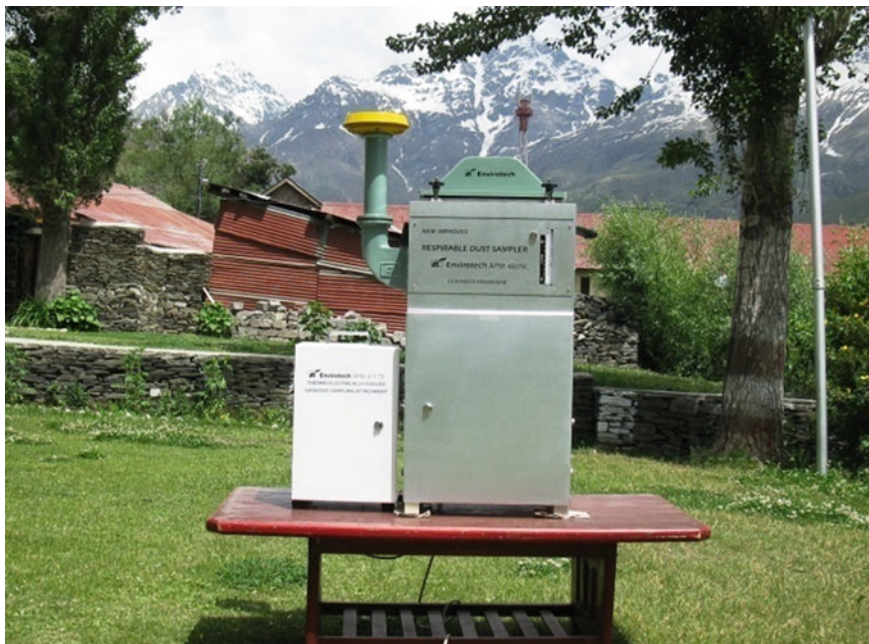
Fig. 13.2 Respirable Dust Sampler (RDS) installed in Keylong, district Lahul and Spiti
