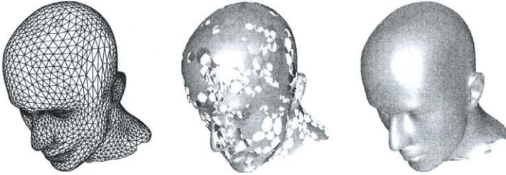
Figure 10.16. A generalized box spline surface of order 2 (middle) with control net (left) and G^2 -fillings (right). (courtesy of Georg Umlauf)
