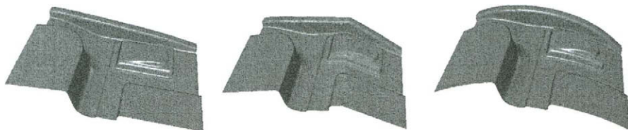
Figure 14.8. A deformation of the global shape is not only characterized by a large support (topologically coarse) but also by its smoothness (low geometric frequency). The object on the left is globally deformed by using a (non-smooth) piecewise linear function in the center and a smooth function on the right.
