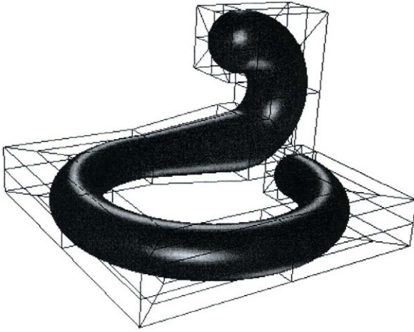
Figure 5.10. A canal surface composed of piecewise quadratic patches. (Figure courtesy of D. Hansford).
