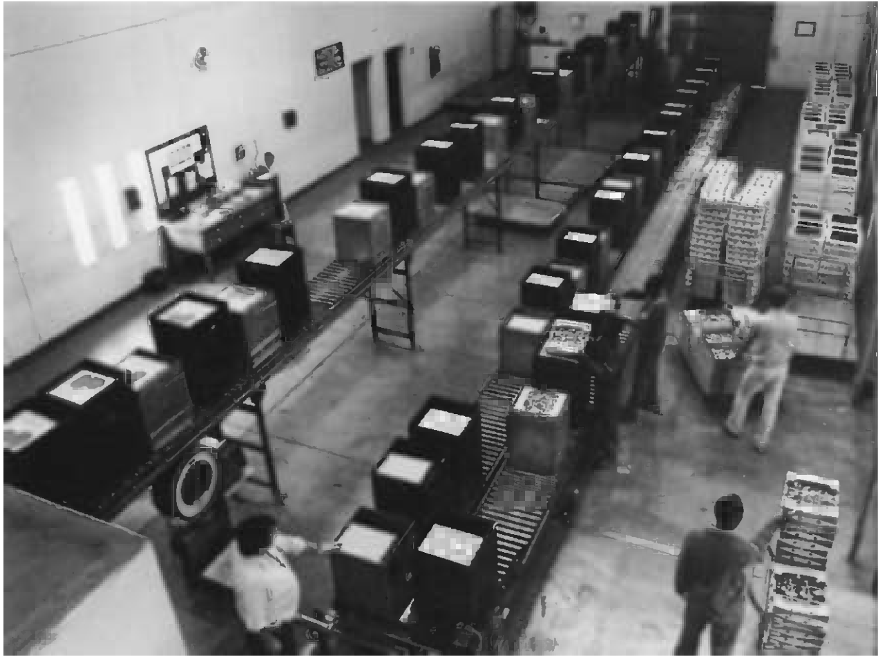
Figure 15.24 Radionuclide (380 kCi ^{60}\text{Co} ) commercial irradiator. Product loading area. Radurization (2.4 kGy) of strawberries to control Rhizopus and Botrytis . Courtesy of Radiation Technology Division, Atomic Energy Corporation of South Africa (Pty.) Ltd., Pretoria.
