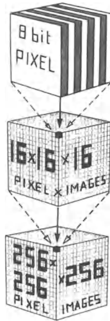
Figure 4. Graphic demonstration of the amount of information stored in a digitized block of data comparable to the average requirements in digital angiocardiology. Each picture element (“pixel”) has 8 bits for gray level resolution. Each cube appears at the upper corner of the lower cube.
