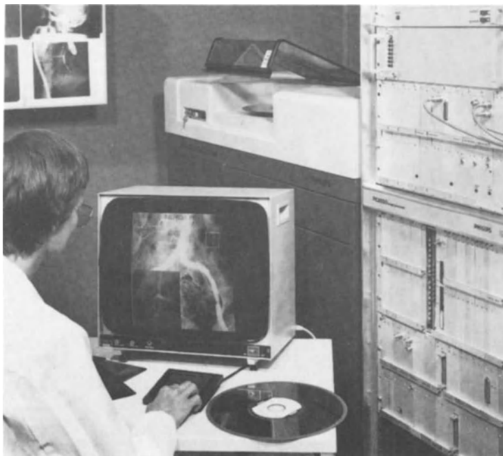
Figure 4. Experimental PACS based on an early laboratory prototype of a DOR drive, and a laboratory model high-power picture processor for workstation application.
