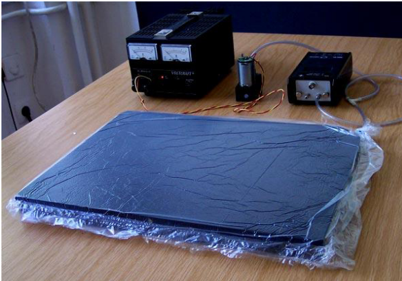
Fig. 6. Sound-insulating experimental panel enclosed in an airproof package (Vacuum (low pressure) pump and indicator in the rear)
