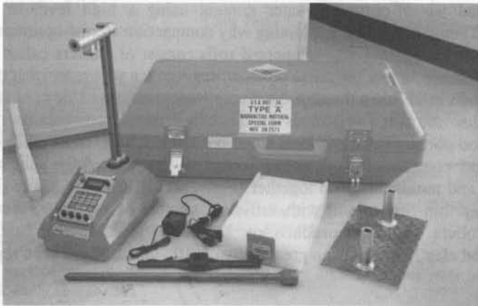
Fig. 2.15 Troxler 3400 Series Nuclear Moisture-Density Gauge (Distributed by Troxler Electronic Laboratories, Inc., U.S.A.)
