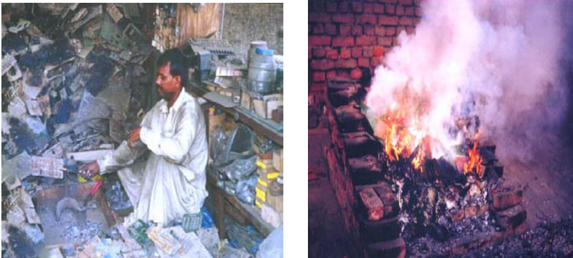
Fig. 3.3 'E-waste recycling shop in Pakistan Burning of WEEE to recover metals (Source: Toxics Link).
