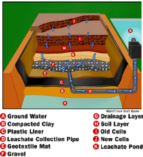
Fig. 7.4 The cross-section drawing shows the structure of a municipal solid waste landfill. The arrows indicate the flow of leachate
