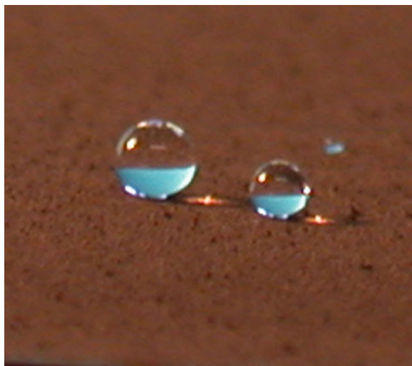
Fig. 4. Water droplets resting on a fluorinated copper oxide nano-needle surface.
