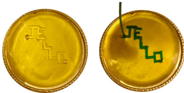
Fig. 4. A chip made into the letters “JELLO” and filled with green colored water demonstrates the ease of making complex patterns with the Jell-O® technique (reproduced from ref. 8 with permission from American Chemical Society).
