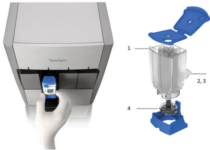
Fig. 6. GeneXpert® platform and disposable cartridge with components such as (1) processing chambers that contain reagents, filters, and capture technologies necessary to extract, purify, and amplify target nucleic acids; (2) optical window that enables real-time optical detection; (3) reaction tube for rapid thermal cycling; and (4) valve that enables fluid transfer from chamber to chamber and may contain nucleic acid lysis and filtration components. (Reproduced with permission from Cepheid).
