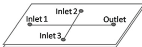
Fig. 1. Schematic of the microfluidic glass chip with a cross-channel as used in this method. Inlet 1 is for agarose PCR sample and inlets 2 and 3 are for oil sheath flow. Use a plastic three-port valve to divide oil fluid to two equal streams infusing into inlets 2 and 3 . The generated emulsion is directly infused into a 0.6 mL PCR tube from the outlet.
