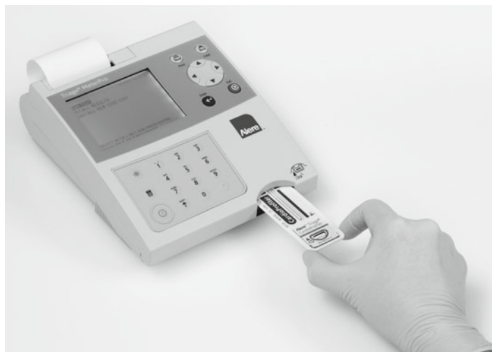
Fig. 5. Biosite's POCT Desktop Platform Triage ® MeterPlus with a test cartridge. (Reproduced with permission from Alere San Diego, Inc.).
