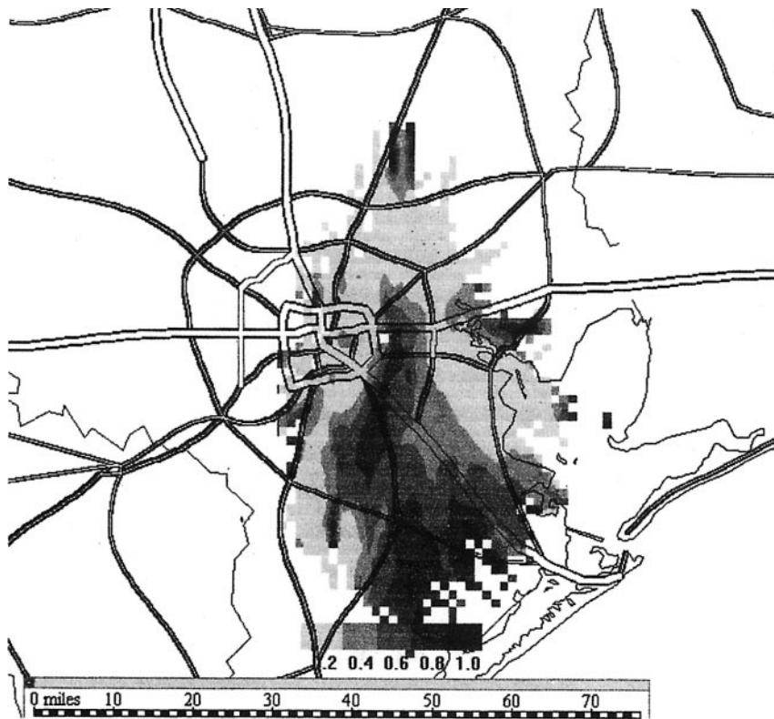
Figure 11 Residence time weighted concentration for 2-methylpentane measured at the Clinton site in Houston, TX
