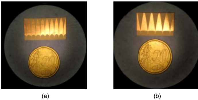
Figure 3.46 Manufactured arrays at 80 GHz (a) Vivaldi and (b) LTSA.
