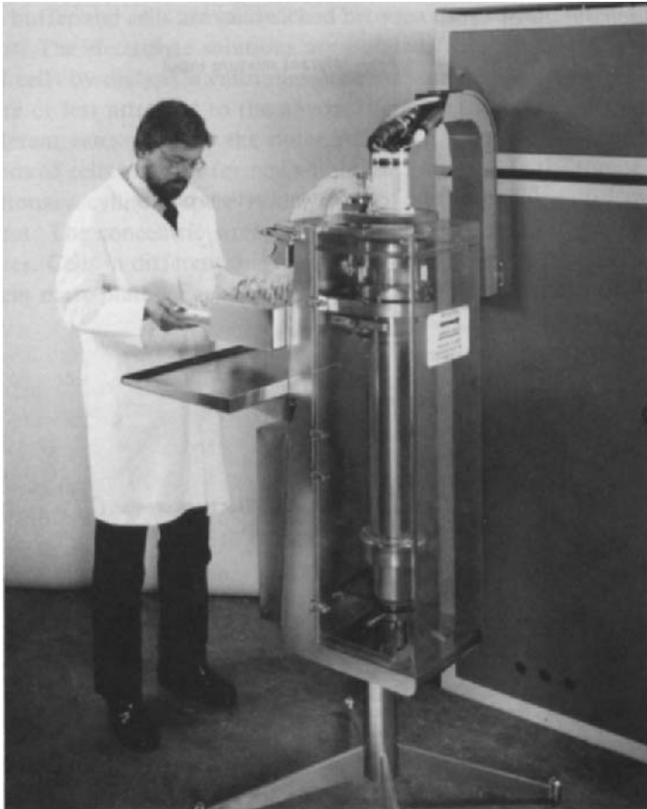
Fig. 7.5. Biostream electrophoresis apparatus. Courtesy of CJB Developments.
