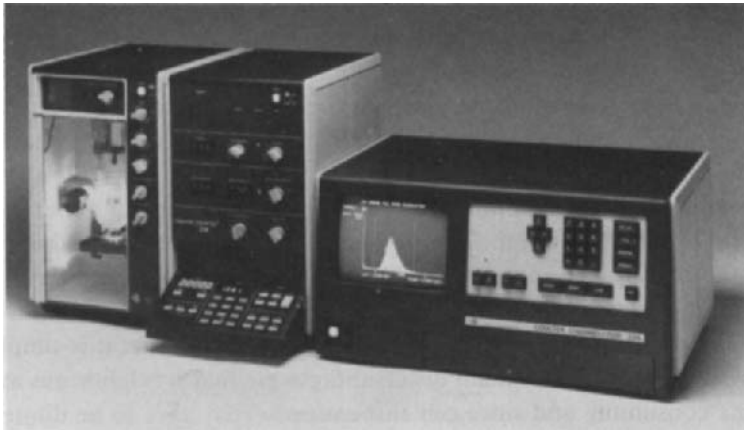
Fig. 2.3. Coulter Counter Model ZM with Channelyzer. Left, counting aperture; centre, module for setting cell size range and displaying cell count; right, Channelyzer. (Courtesy of Coulter Electronics).
