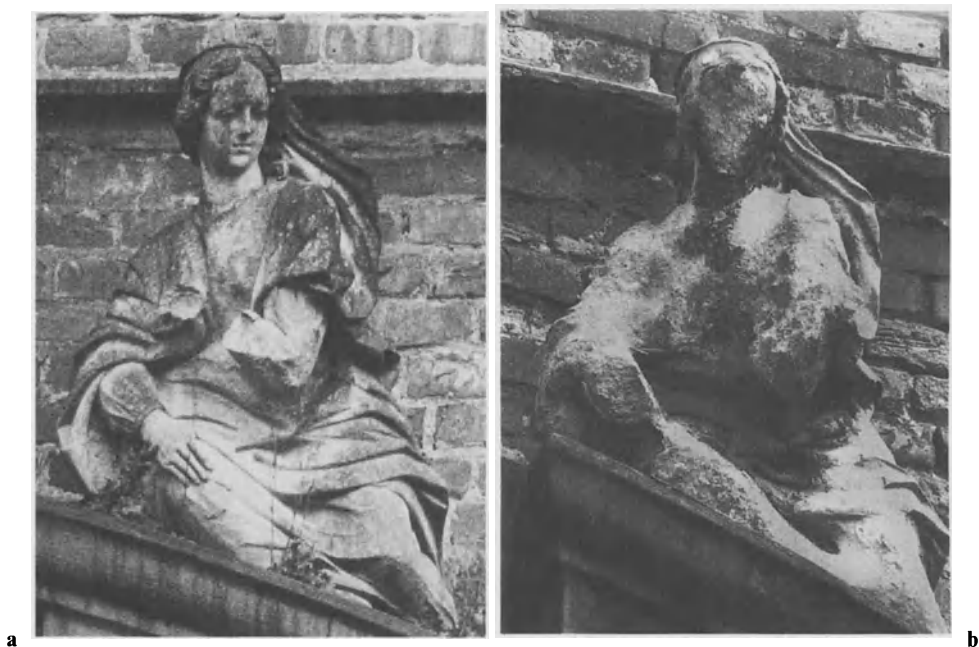
Fig. 4.4. Sandstone statue from the year 1702, Herten Castle near Essen, Germany. Condition in the year 1908 (a) and 1969 (b) [16]
