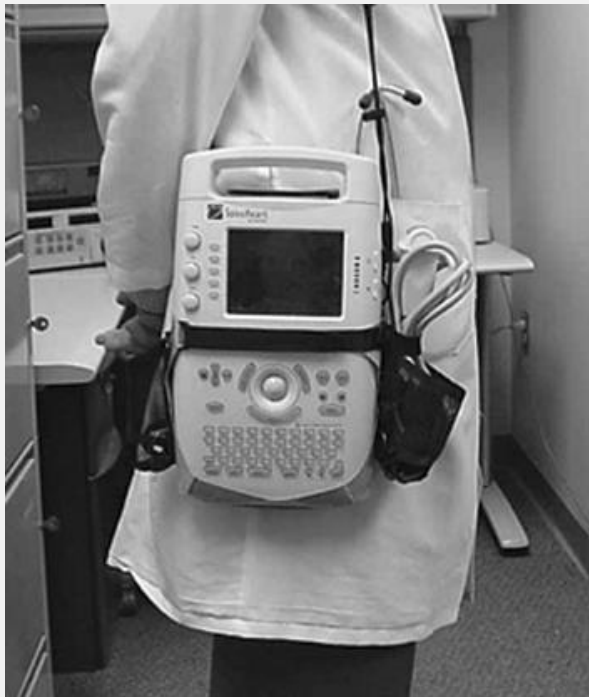
FIGURE 3.22. Hand-carried portable two-dimensional ultrasound device. Note the overall size of the device and its easy portability.
