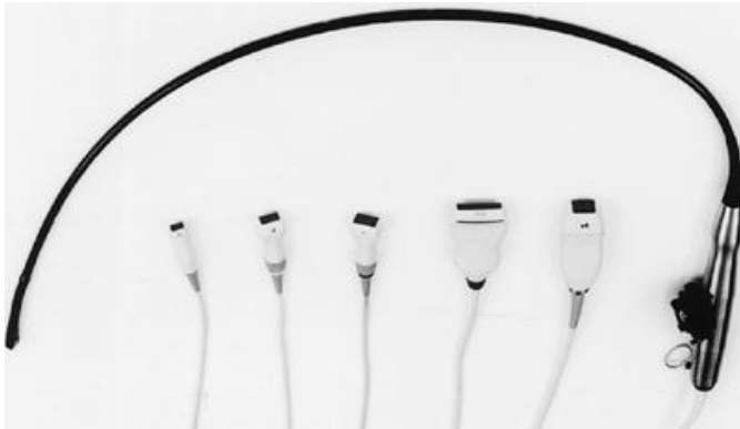
FIGURE 5.1. A variety of transducers are available for use in clinical echocardiography. A transesophageal transducer and five transthoracic probes are illustrated.
