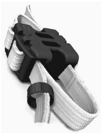
FIG. 38-3. The Wallis implant consists of polyetheretherketone interspinous spacer, anchored in its place by wrapping two woven Dacron ligaments around the spinous processes of the adjacent vertebrae under tension. (From Sengupta DK. Dynamic stabilization devices in the treatment of low back pain. Orthop Clin North Am 2003; 35(1):43–56, with permission.)
