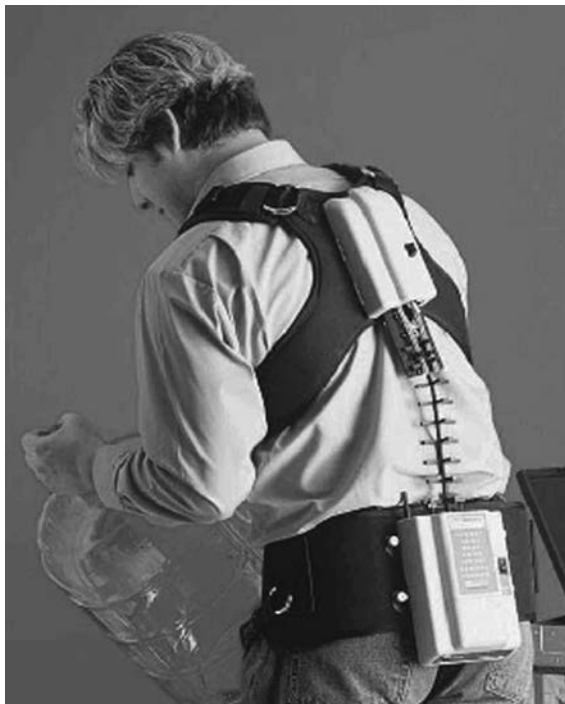
FIG. 17-7. The lumbar motion monitor used to track trunk kinematics during occupational activities.
