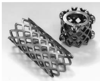
FIG. 26-2. Titanium mesh cage (Harms), an example of a vertical cylinder. End-rings ( right side ) can be added to the reduce stress concentration at the ends of the cage, and therefore reduce the chance of sinking into the end plate.
