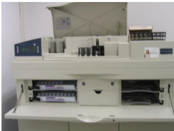
Figure 3. Automated device for cytologic assessment (ThinPrep Integrated Imager System [Hologic Inc., Bedford, MA, USA]).
