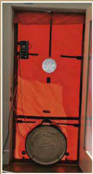
Fig. 10.6-7: A blower door, operated by a building scientist at Southern Energy Management, depressurizes the home.
