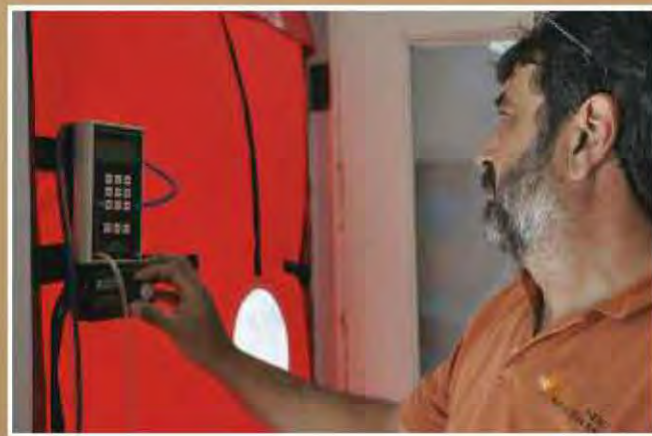
Fig. 10.6-7: A blower door, operated by a building scientist at Southern Energy Management, depressurizes the home.
