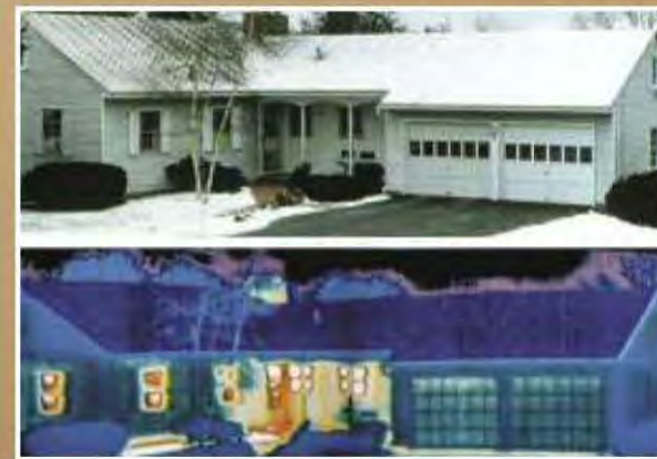
Fig. 10.2: An FLIR Camera indicates the best and least insulated parts of the home.
