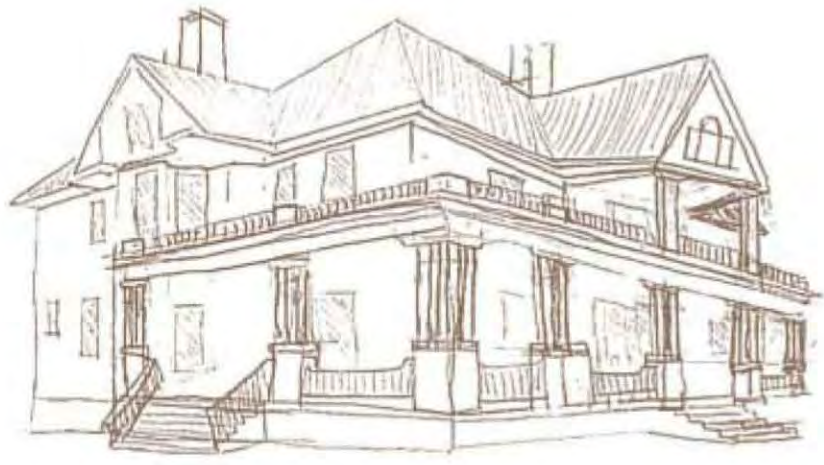
Fig. 8.39-41: This homeowner preferred the three column massing sketched above. Historic research indicated that sided columns (bottom) were original defining characteristics of the home. SHPO denied the three-column design and requested the original columns be restored (right).
