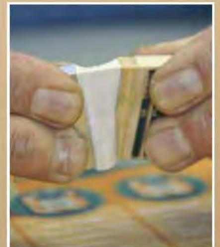
Fig. 10.8-9: There are dozens of different caulk options, each with a specific application. Above, premium Kevlar caulks are so strong and pliable they are difficult to pull apart from even dissimilar materials, making it less likely to split as a house settles and moves seasonally.
