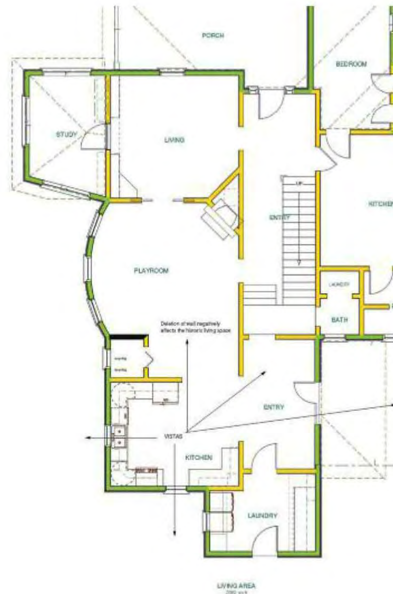
Fig. 6.4: Ideally the children could play in view of parents working in the kitchen, but the removal of the wall negatively affects the historic integrity of the living space. Such a proposal would likely be denied by a SHPO.
