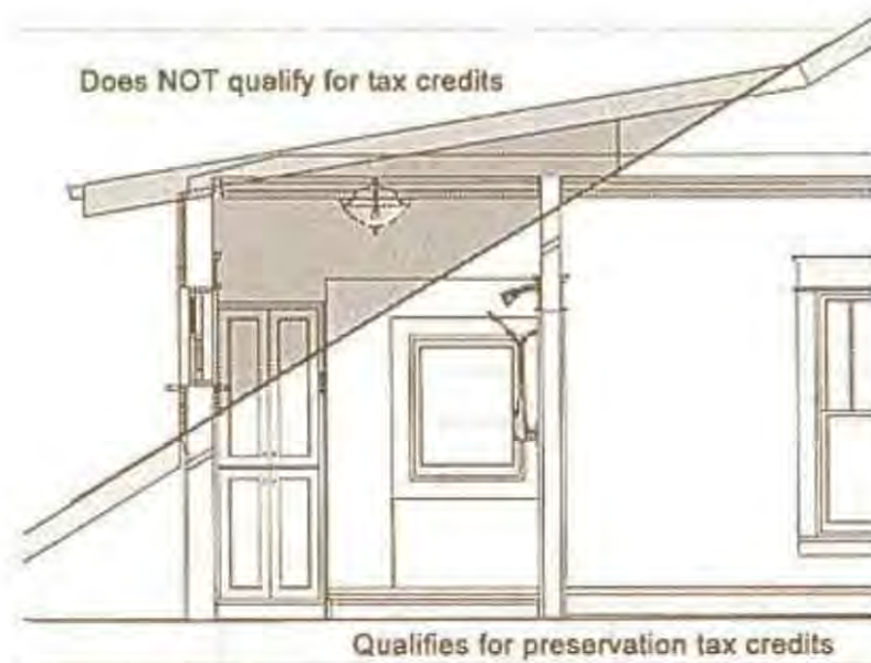
Fig. 7.14: A dormer bump-out proposal expands the envelope. This state's SHPO declared that all costs inside the pre-existing 3D envelope qualify, while costs outside do not.
