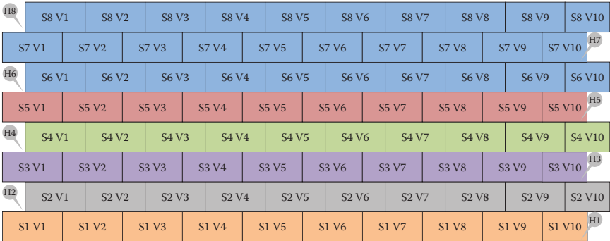
COLOR FIGURE 8.1 Shell cutting plan with weld map.
