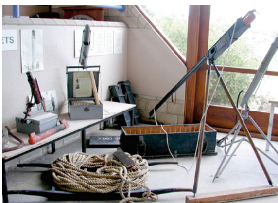
Fig. 7.7 Life-saving rocket launchers display. Note rockets projectile in barrels tubes (QMM collection)
