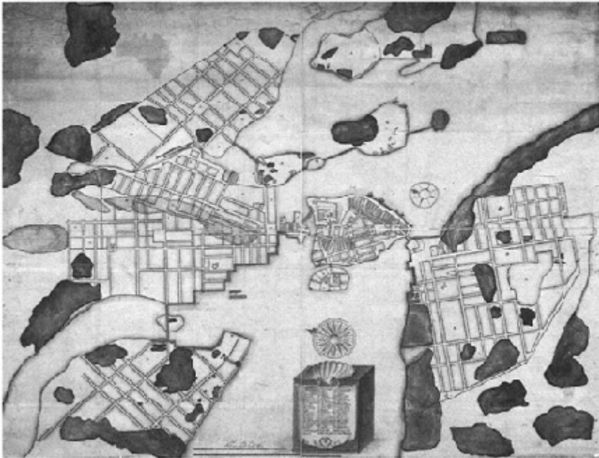
Figure 5.2. Stockholm, a map from around 1645. After 1636 'Malmarna', the districts surrounding 'Staden mellan broarna' (the Town between the Bridges) were either redeveloped or planned afresh. The old winding streets were replaced by street networks as close to a gridiron pattern as the topography permitted. Source: Det kongelige bibliotek, Copenhagen.
