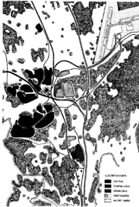
Figure 5.16. Mārsta, master plan from 1960. The centre is surrounded by residential areas situated on higher ground. The major development of Mārsta on the northern side of Stockholm was contingent on the proximity of Arlanda, Stockholm's international airport, which was inaugurated that year. (Centrum=centre; Flerfamiljshus=apartment houses; Enfamiljshus=single-family houses; Arbetsområde=commercial and industrial area; Militärt område=military area) Source: Åström (1967).
