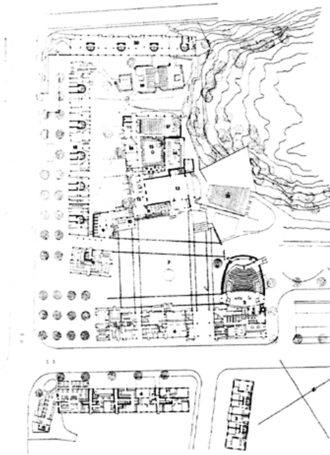
Figure 5.21. Årsta centre, designed by Erik and Tore Ahlsén and inaugurated in 1953. Årsta was the most ambitious attempt in Sweden to create a 'community centre'. The idea was to design and combine the buildings in such a way as to encourage the residents to meet and partake in various activities. (1) and (2) cinema; (3) and (20) dwellings; (5) restaurant; (6), (8) and (18) shops and officespace; (7) square; (9), (10) and (12) entrances, vestibules etc.; (11) café; (13) theatre; (14) and (15) library; (16) studios; (17) concert hall. Source: Arkitektur 1980.
