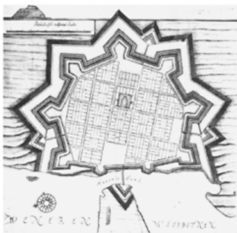
Figure 5.5. Vänersborg was founded in the early 1640s on the Göta Älv river, not far from its outflow from Vänern, the largest lake in Sweden, and thus at an important point in the communications system. The simple gridiron plan was probably drawn by Olof Hansson Örneufvud, head of the Swedish fortification corps. The planned fortifications were never executed. Source: Krigsarkivet, Stockholm.
