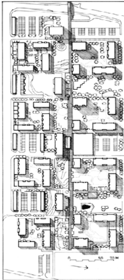
Figure 3.22. Olari, plan made at the end of the 1960s by the Espoo town planning office in collaboration with the Järvinen-Valjakka firm of architects, which produced the designs for the houses. The pedestrian street runs along the flat ridge. The blocks of flats range from three to nine storeys and the area is intended for a maximum population of 2,270. The semi-closed blocks came to be known as the 'windmill' model. The area was built 1969–73 and was later extended. The illustration has been redrawn by the author. Source: Finland bygger, 5 (Helsinki: Museum of Finnish Architecture, 1966).
