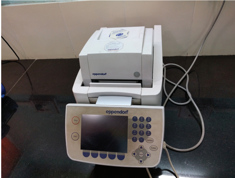
FIGURE 1.13 PCR thermal cycler. (Courtesy of Dr. S. G. Borkar, Department of Plant Pathology, Mahatma Phule Krishi Vidyapeeth, Rahuri.)
