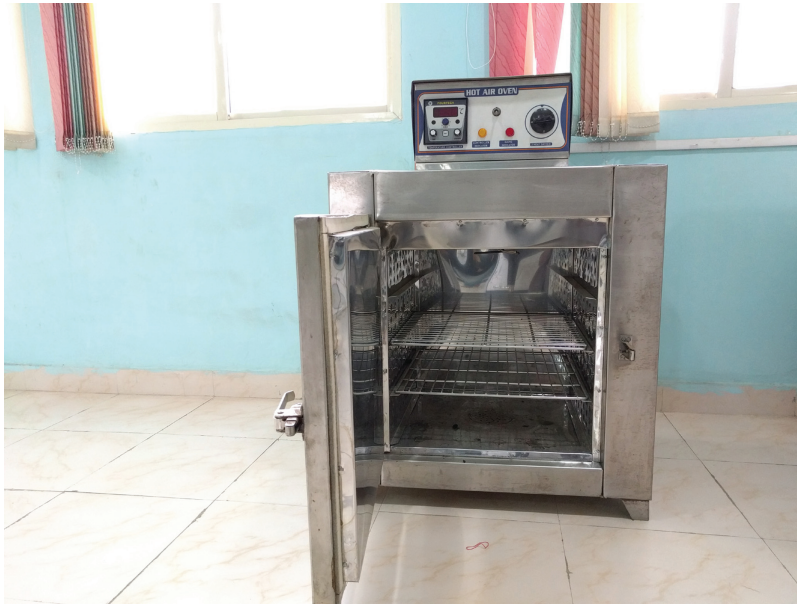
FIGURE 1.5 Hot air oven for sterilization. (Courtesy of Dr. S. G. Borkar, Department of Plant Pathology, Mahatma Phule Krishi Vidyapeeth, Rahuri.)
