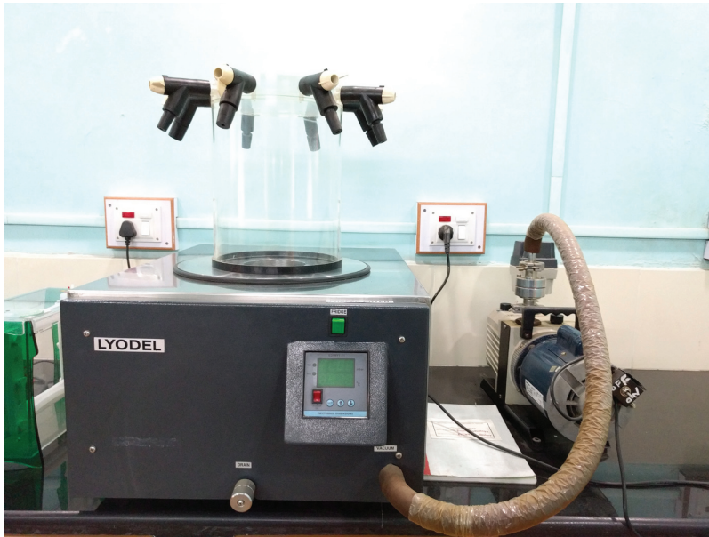
FIGURE 1.15 Lyophilizer. (Courtesy of Dr. S. G. Borkar, Department of Plant Pathology, Mahatma Phule Krishi Vidyapeeth, Rahuri.)
