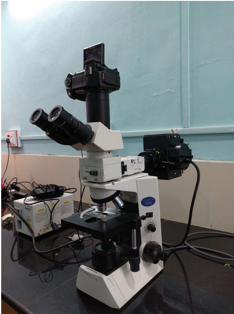
FIGURE 1.8 Compound microscope. (Courtesy of Dr. S. G. Borkar, Department of Plant Pathology, Mahatma Phule Krishi Vidyapeeth, Rahuri.)
