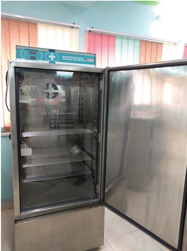
FIGURE 1.3 BOD incubator. (Courtesy of Dr. S. G. Borkar, Department of Plant Pathology, Mahatma Phule Krishi Vidyapeeth, Rahuri.)
