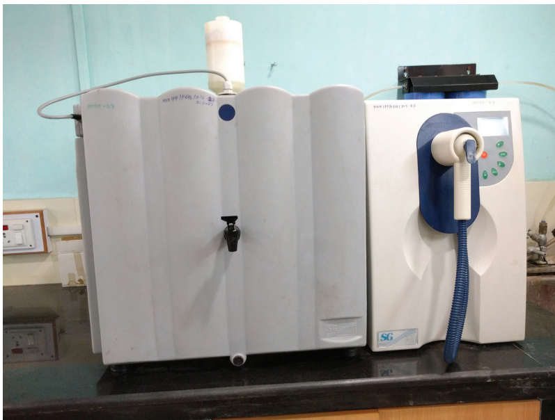
FIGURE 1.6 Ultrapure water machine. (Courtesy of Dr. S. G. Borkar, Department of Plant Pathology, Mahatma Phule Krishi Vidyapeeth, Rahuri.)
