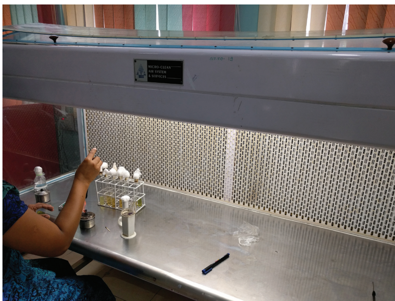
FIGURE 1.2 Laminar air flow cabinet. (Courtesy of Dr. S. G. Borkar, Department of Plant Pathology, Mahatma Phule Krishi Vidyapeeth, Rahuri.)
