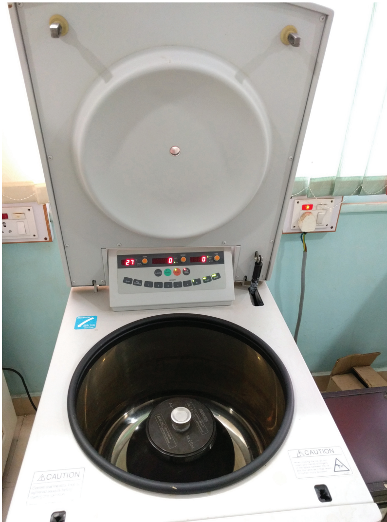
FIGURE 1.10 High speed centrifuge. (Courtesy of Dr. S. G. Borkar, Department of Plant Pathology, Mahatma Phule Krishi Vidyapeeth, Rahuri.)
