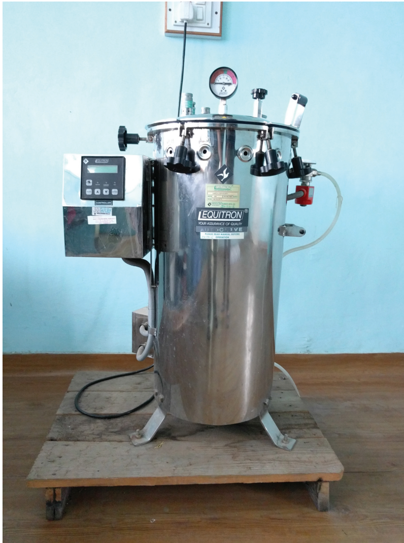
FIGURE 1.7 Autoclave for sterilization. (Courtesy of Dr. S. G. Borkar, Department of Plant Pathology, Mahatma Phule Krishi Vidyapeeth, Rahuri.)
