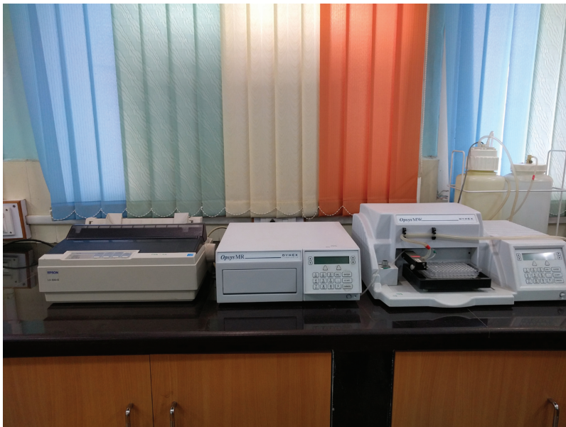
FIGURE 1.12 ELISA unit. (Courtesy of Dr. S. G. Borkar, Department of Plant Pathology, MPKV Mahatma Phule Krishi Vidyapeeth, Rahuri.)
