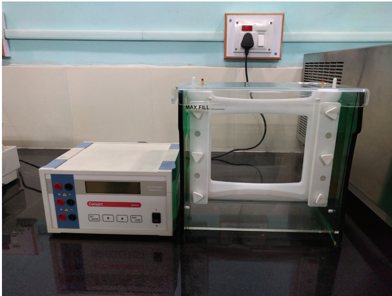
FIGURE 1.11 Gel electrophoresis unit. (Courtesy of Dr. S. G. Borkar, Department of Plant Pathology, Mahatma Phule Krishi Vidyapeeth, Rahuri.)
