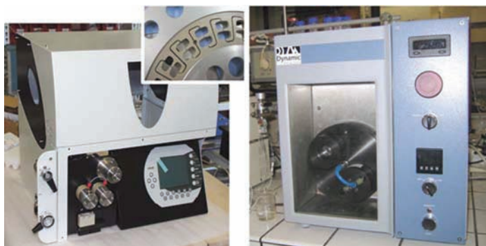
Color Figure 7.4 (Left) The fast centrifugal partition chromatograph (FCPC) 100 chromatograph with hydrostatic column of 100 mL with integrated alternating pump and pilot electronics ( www.armen-instrument.com , Vannes, France); the upper inset shows a part of a disk with the engraved double channels and connecting ducts. (Right) The Milli chromatograph with hydrodynamic CCC column of 18 mL ( www.DynamicExtractions.com , Uxbridge, UK).
