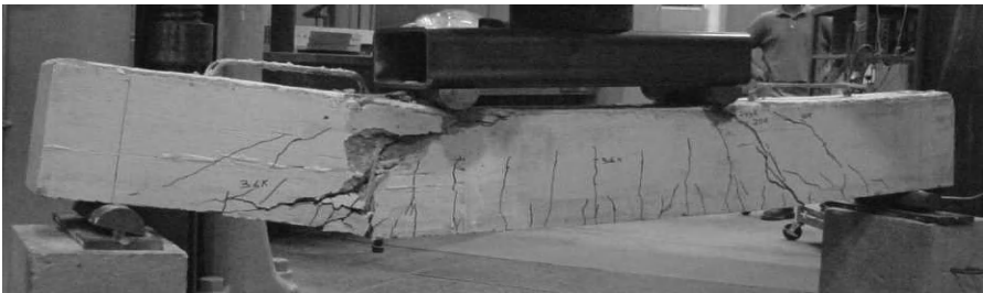
Figure 6.1 Shear failure of an FRP-reinforced beam. (Courtesy of Dushyant Arora.)
