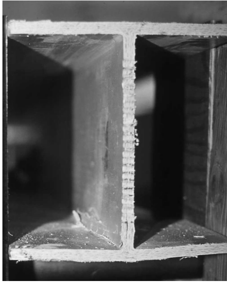
Figure 13.11 Local bearing failure at a simple support.
