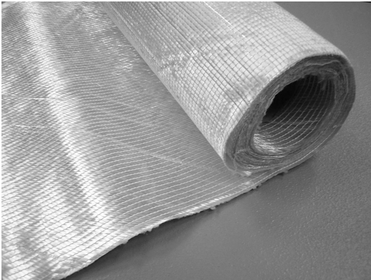
Figure 2.8 Stitched glass fiber fabric.
