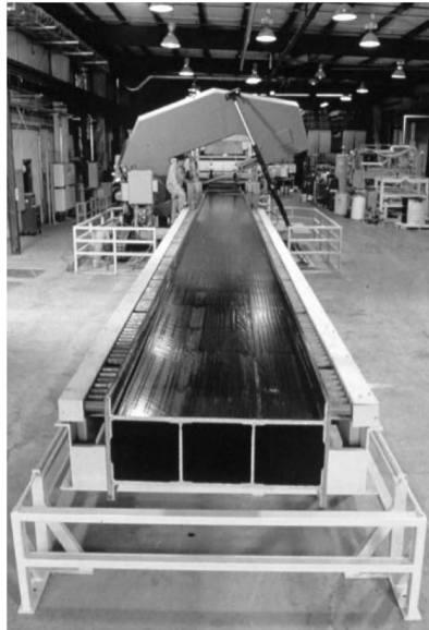
Figure 2.6 Double-web hybrid fiber pultruded beam. (Courtesy of Strongwell.)
