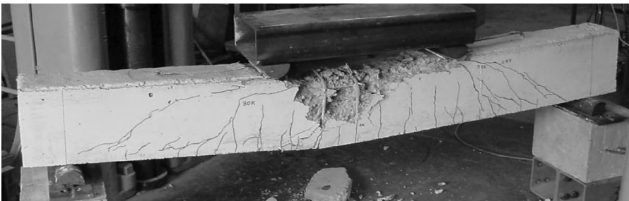
Figure 5.4 FRP-reinforced beam failure due to concrete crushing (FRP 1). (Courtesy of Dushyant Arora.)
