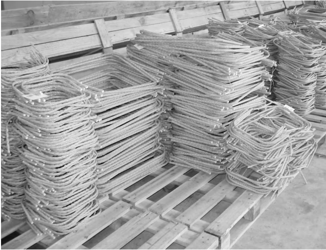
Figure 7.5 FRP rebars with bends at manufacturer’s plant ready for shipping. (Courtesy of Hughes Brothers.)
