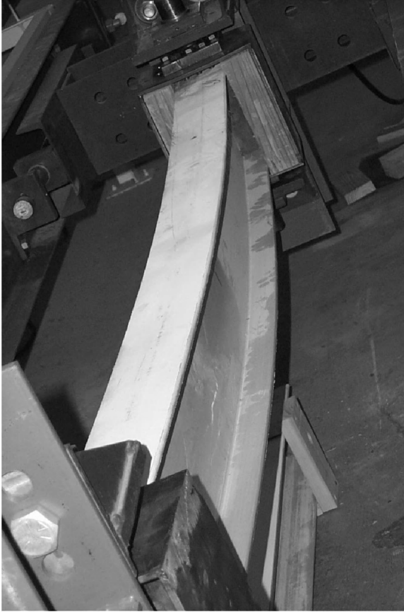
Figure 14.3 Global buckling of an I-shaped profile. (Courtesy of Pizhong Qiao and Julio Davalos.)
