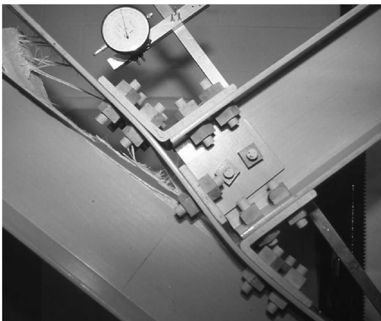
Figure 15.9 Local failure of the web-flange junction in a pultruded member at the connection.
