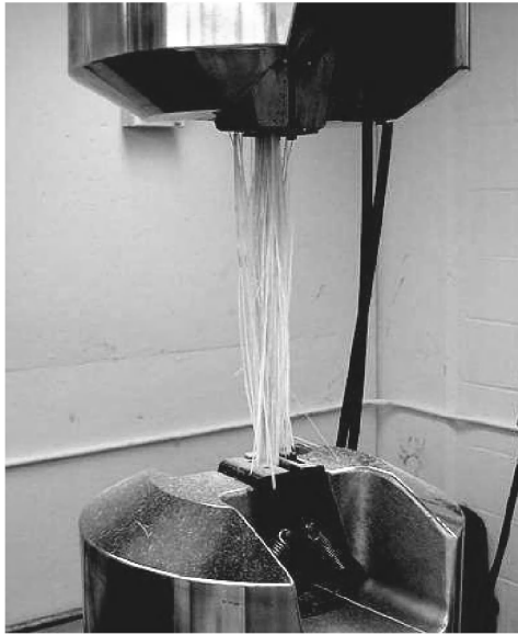
Figure 4.2 Failure of a tensile coupon cut from a No. 7 GRFP rebar. (Courtesy of Joshua Dietsche.)
